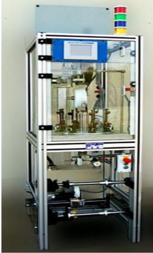
Figure 3.3 Steeger braiding machine that was used to braid the scaffolds
