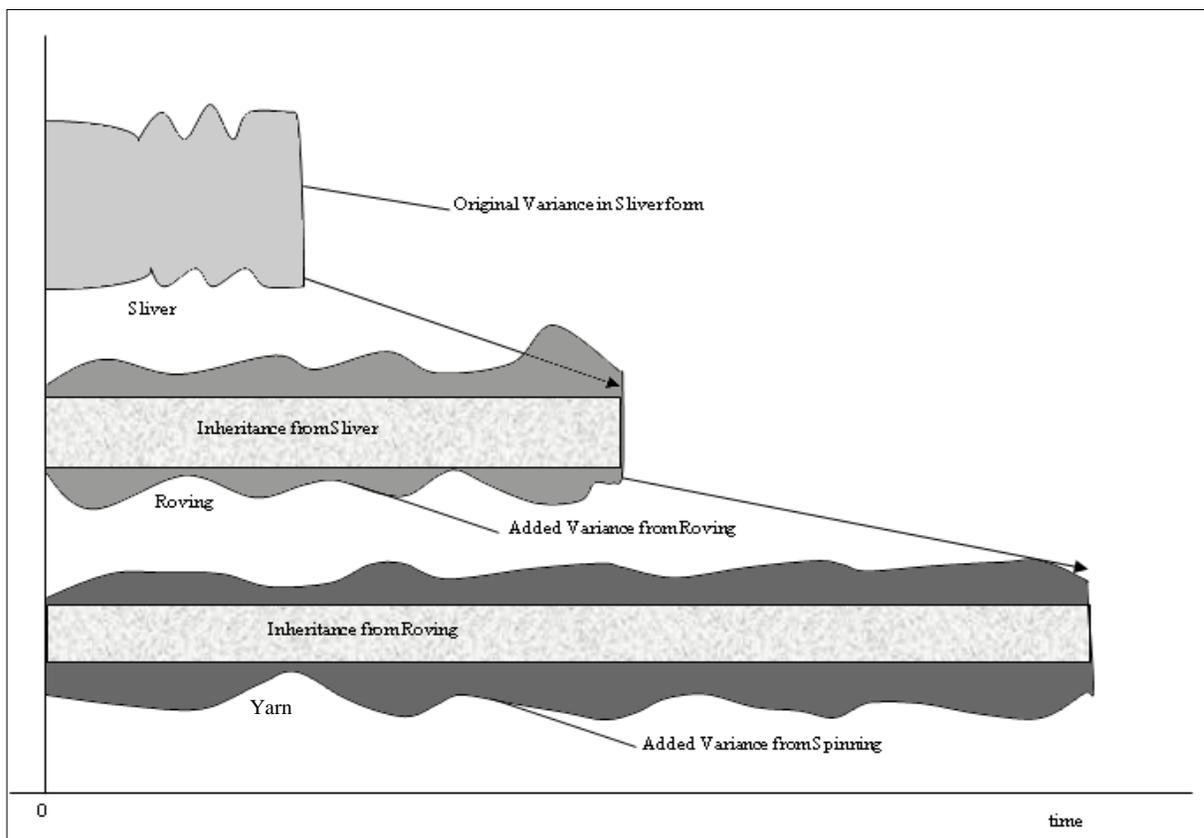
**Figure 4:** Schematic Diagram of Inheritance of Variance from Previous Process Stages
