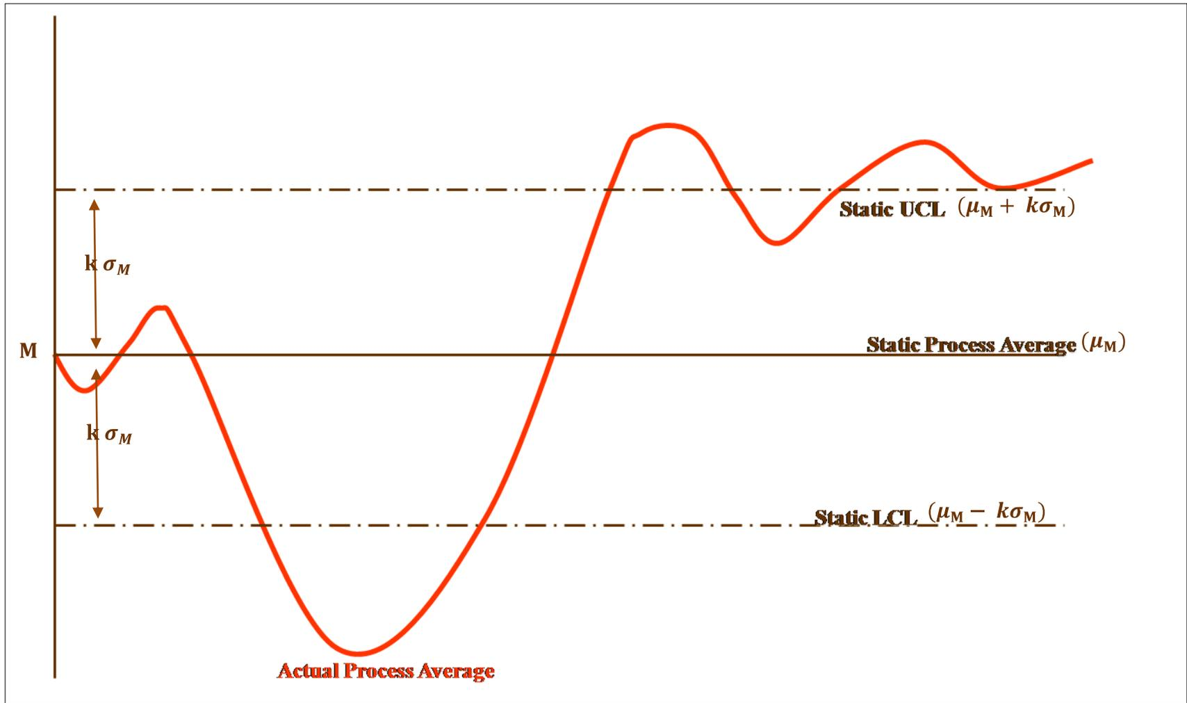
**Figure 1:** Schematic Diagram of the concept for Shewhart Control Charts for any Continuous Manufacturing Process
