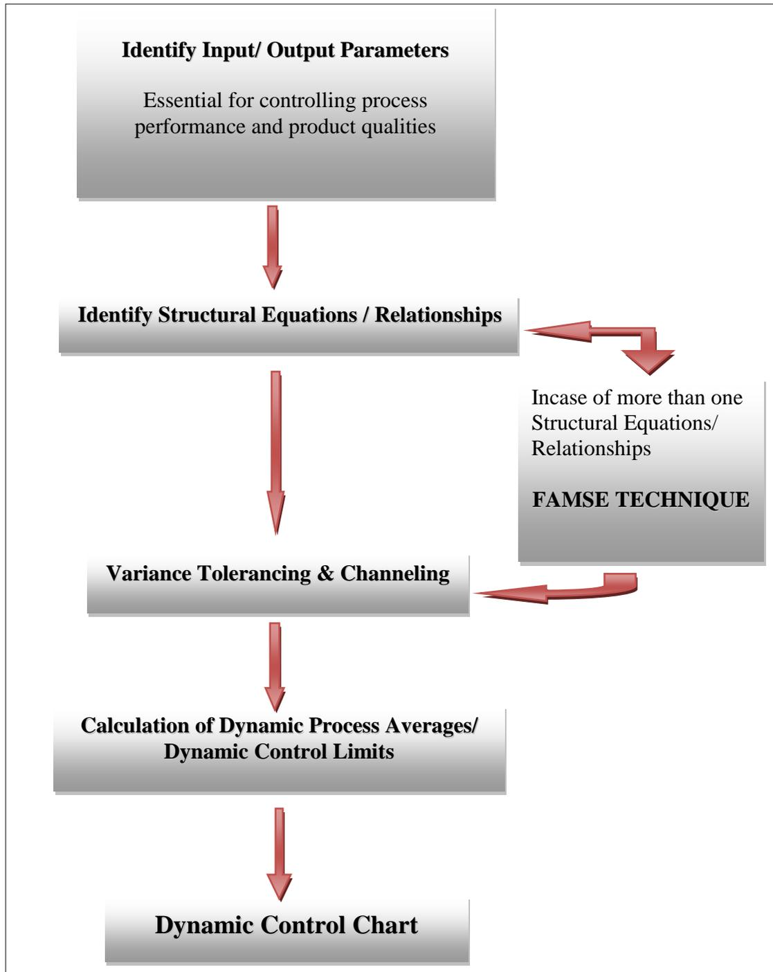
**Figure 6:** Flow Sheet for Design a Dynamic Control Chart
