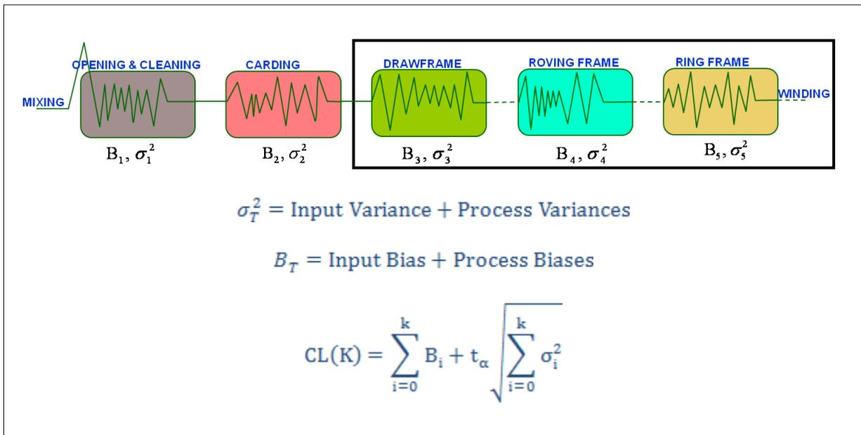
**Figure 2:** Conceptual Frame for Dynamic Control Limits from Mixing/Blending to Ring-frame via the Structural Relationships Developed.
