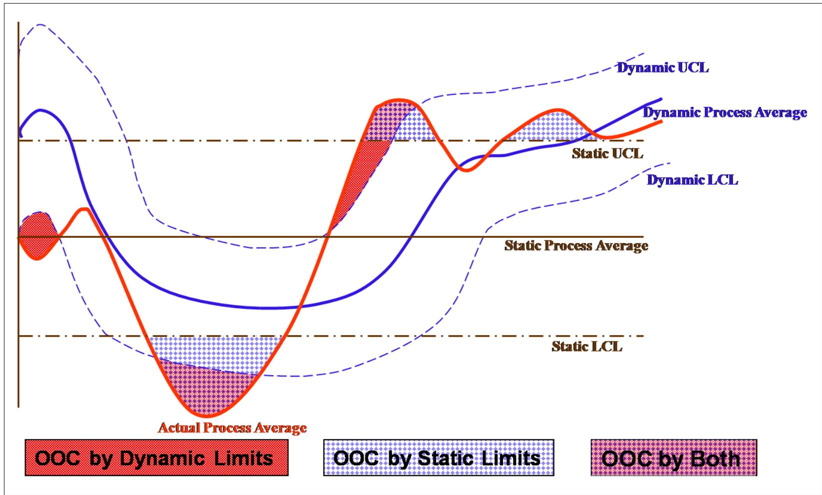
**Figure 3:** Schematic Diagram of a Dynamic Control Chart
