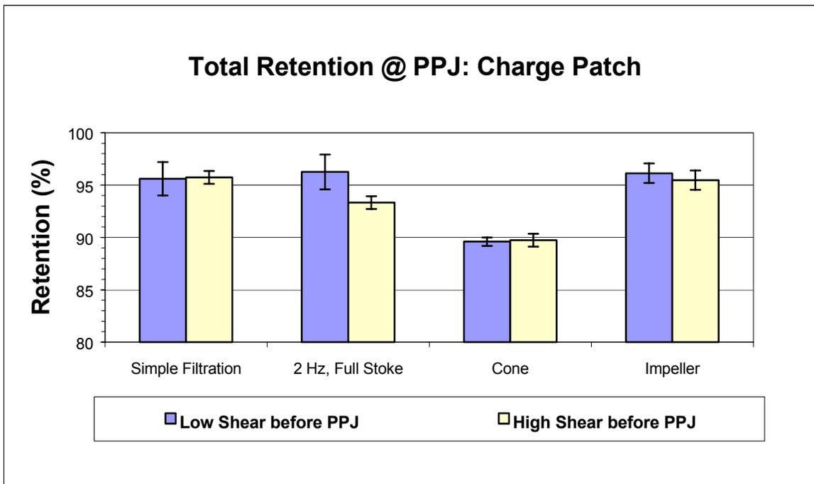
Figure 30 Total retention of different forming regimes (charge patch system)
