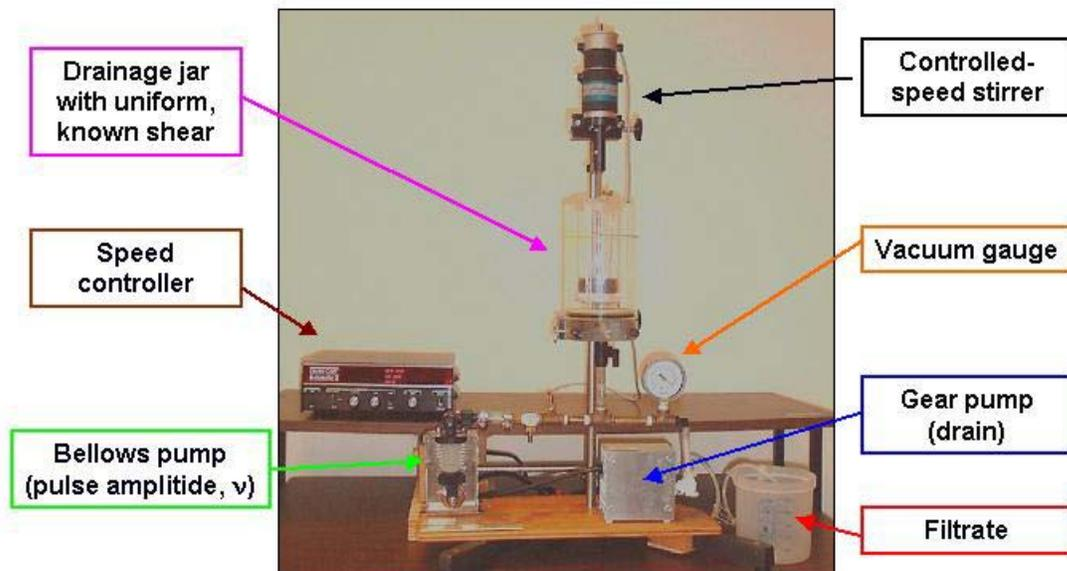
Figure 6 Positive Pulse Jar apparatus for evaluation effects of chemical additives on drainage resistance and final moisture under highly controlled conditions of mixing shear and pulsating flow to simulate the action of hydrofoils during formation of paper
