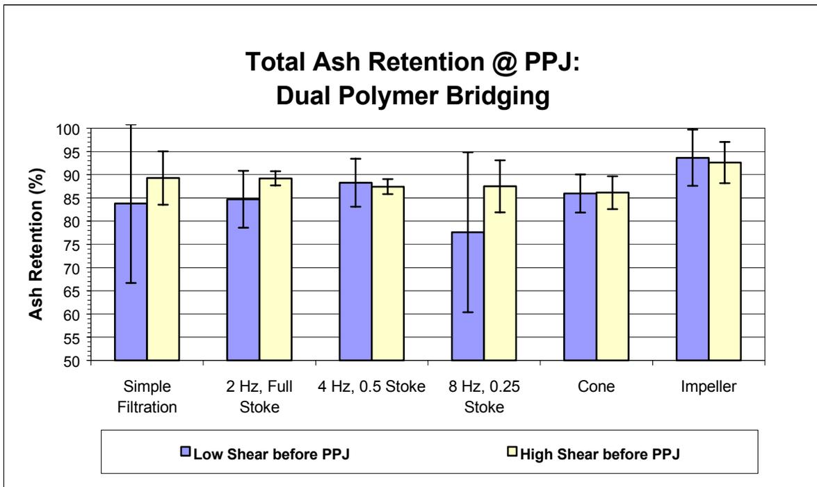
Figure 25 Total ash retention of different forming regimes (dual polymer bridging)
