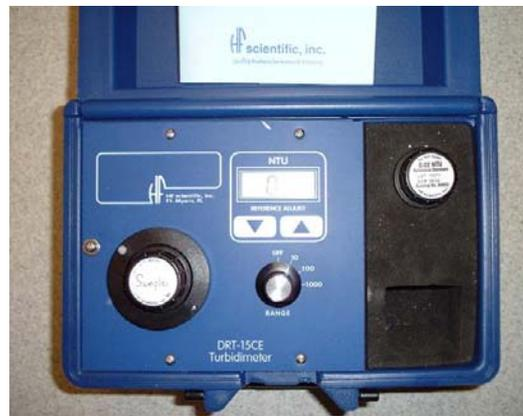
Figure 9 DRT-15CD Turbidimeter
