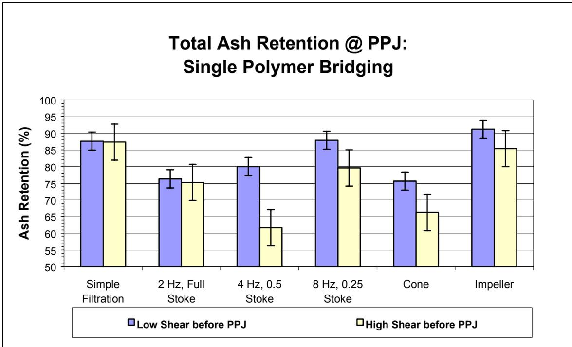
Figure 22 Total ash retention of different forming regimes (single polymer bridging)
