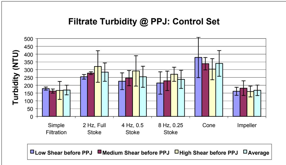
Figure 16 Filtrate turbidity results of different forming regimes (control set)
