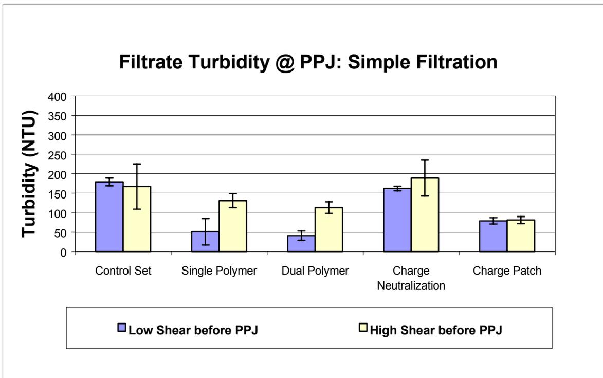
Figure 32 Turbidity results of different retention aid programs (simple filtration)
