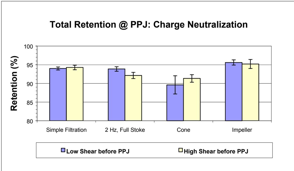
Figure 27 Total retention of different forming regimes (charge neutralization system)
