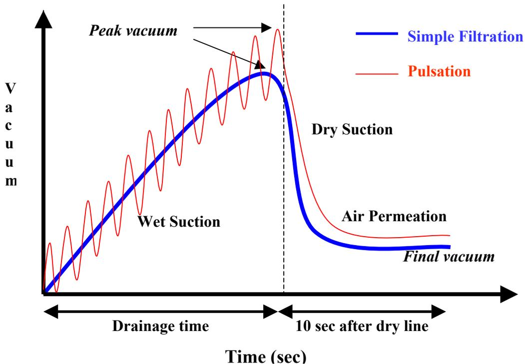
Figure 12 Schematic of observed vacuum curve during drainage in PPJ
