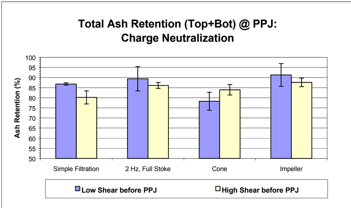
Figure 28 Total ash retention of different forming regimes (charge neutralization system)
