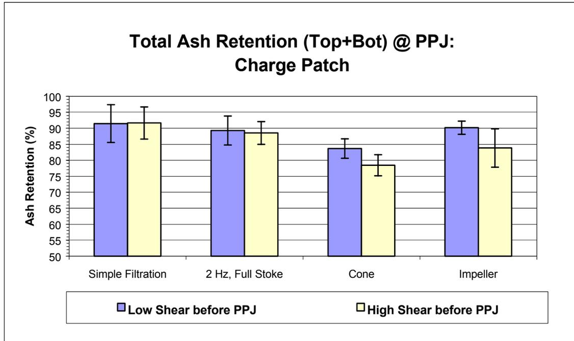
Figure 31 Total ash retention of different forming regimes (charge patch system)
