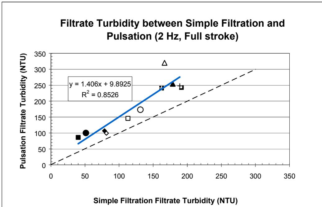
Figure 34 Relationship between simple filtration and pulsation effect in filtrate turbidity
