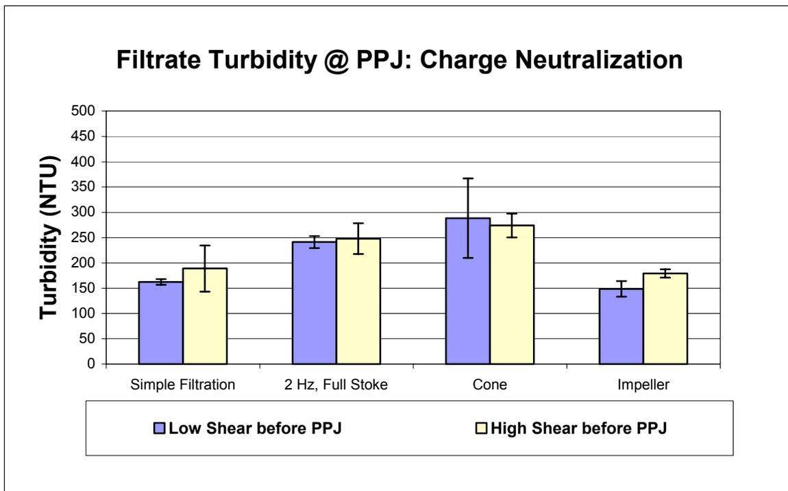
Figure 26 Turbidity results of different forming regimes (charge neutralization system)
