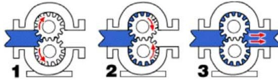
Figure 8 Schematic diagram of external gear pump (57)
