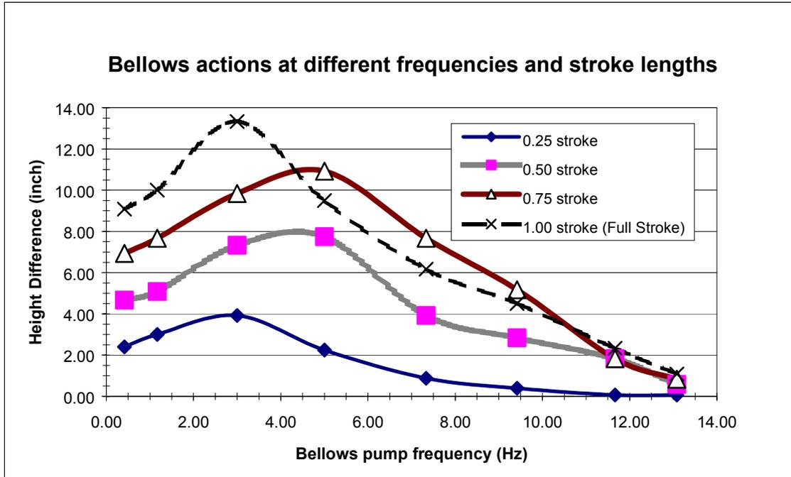
Figure 14 Bellows actions at different frequencies and stroke lengths
