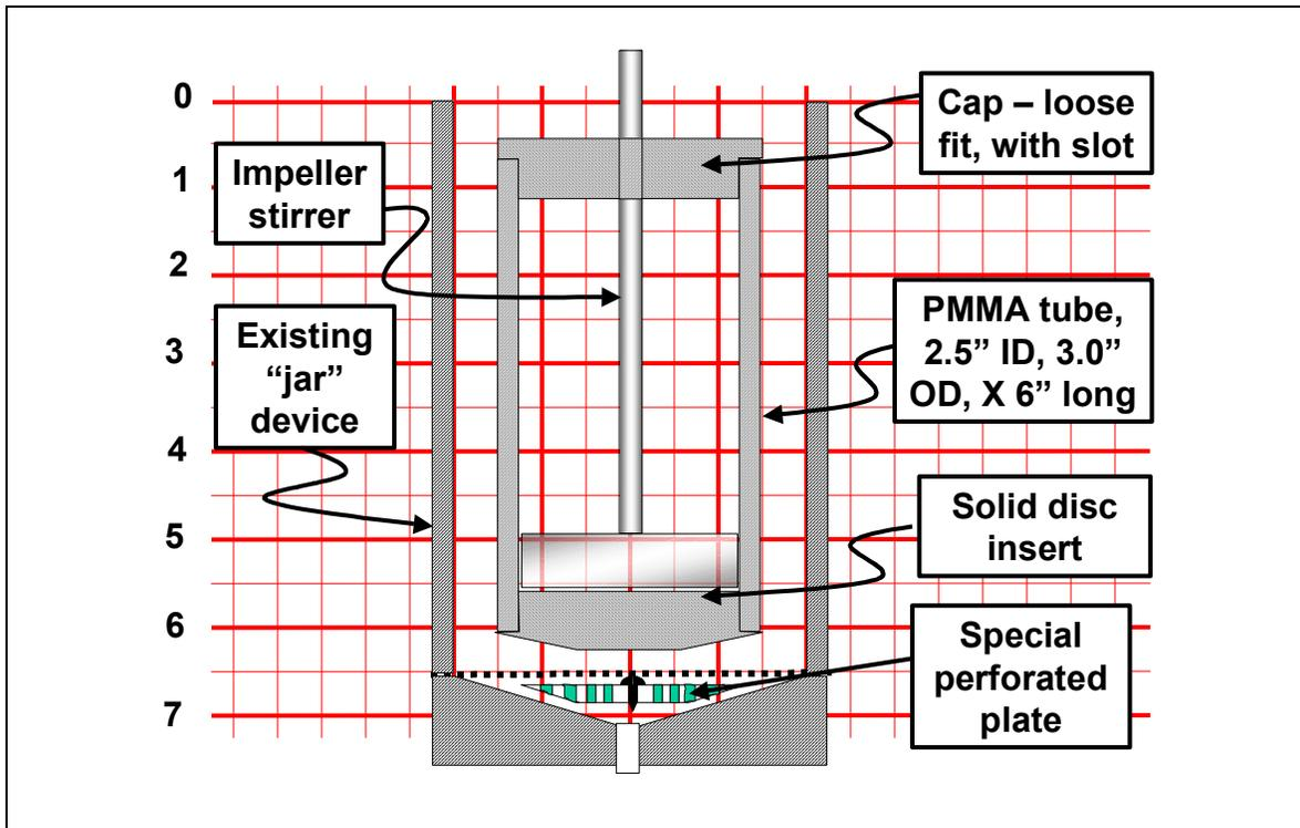
Figure 7 Detail of rotor that applies a nearly constant hydrodynamic shear field to papermaking furnish
