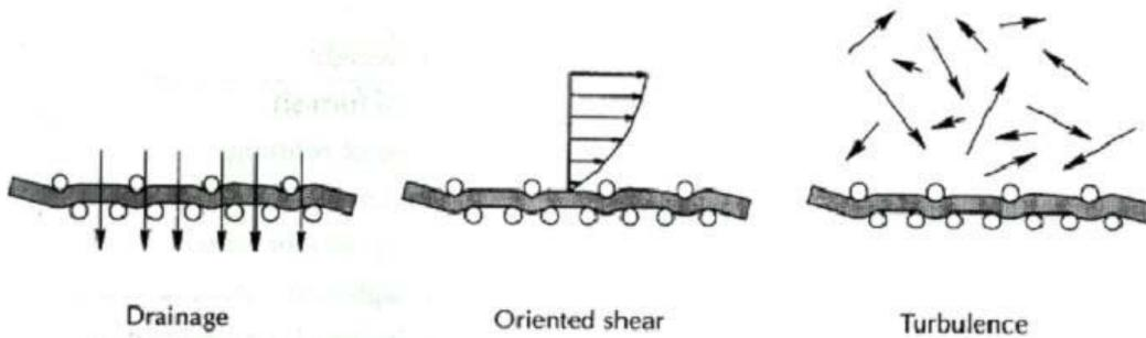
Figure 5 Different shear patterns within a fluid suspension on a wire of a Fourdrinier paper machine (19)
