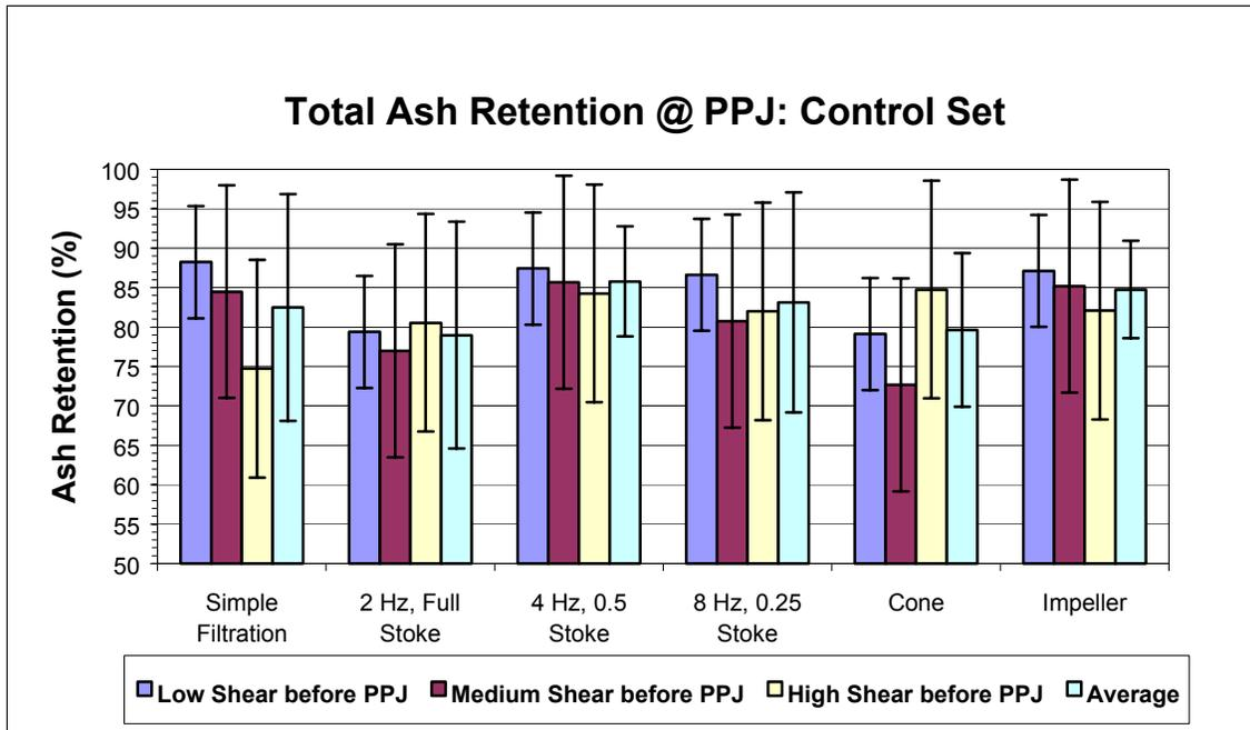
Figure 19 Total ash retention of different forming regimes (control set)
