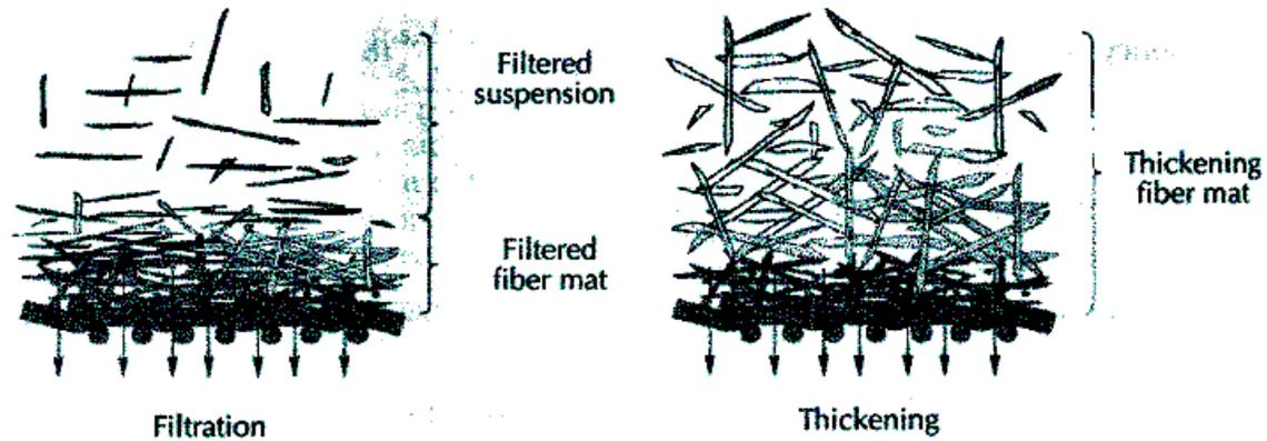
Figure 1 Difference between filtration and thickening (15)
