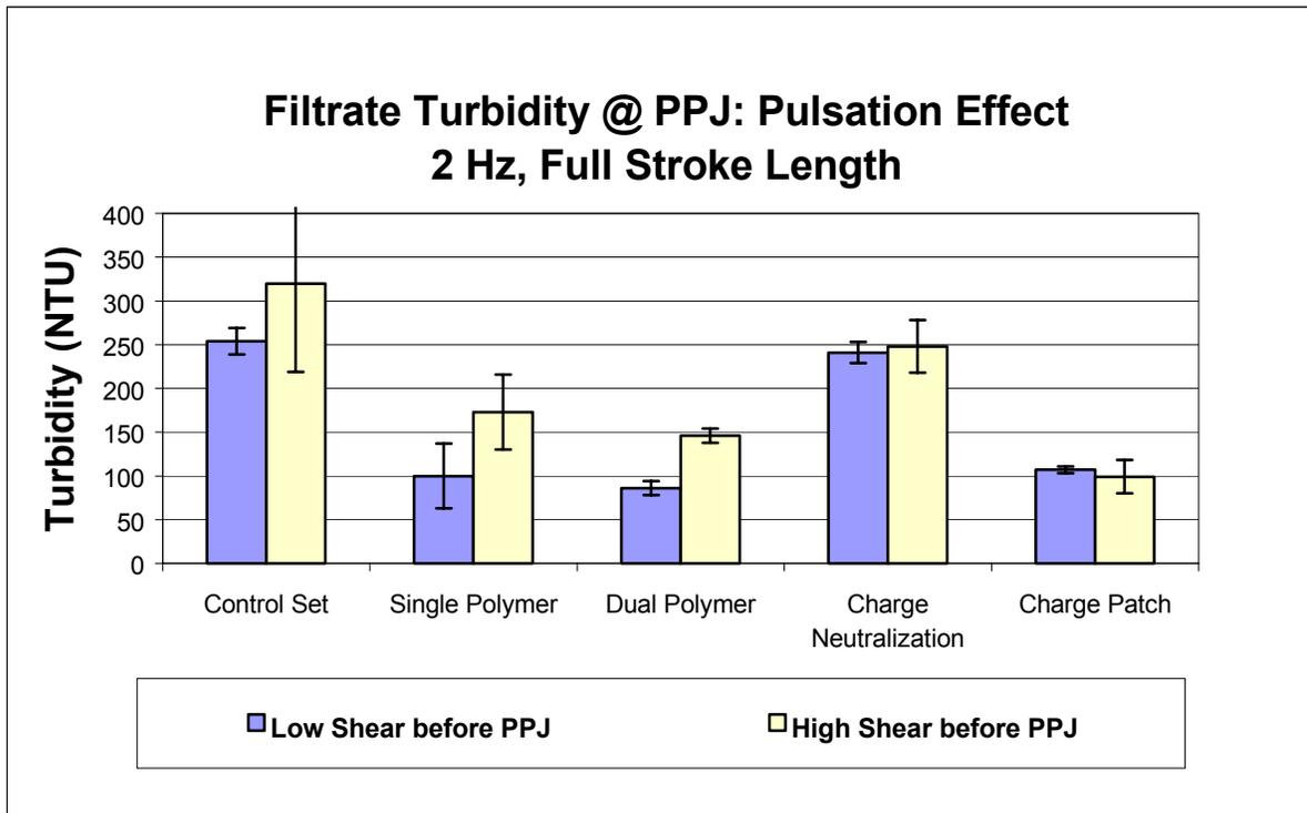
Figure 33 Turbidity of different retention aid programs (pulsation)
