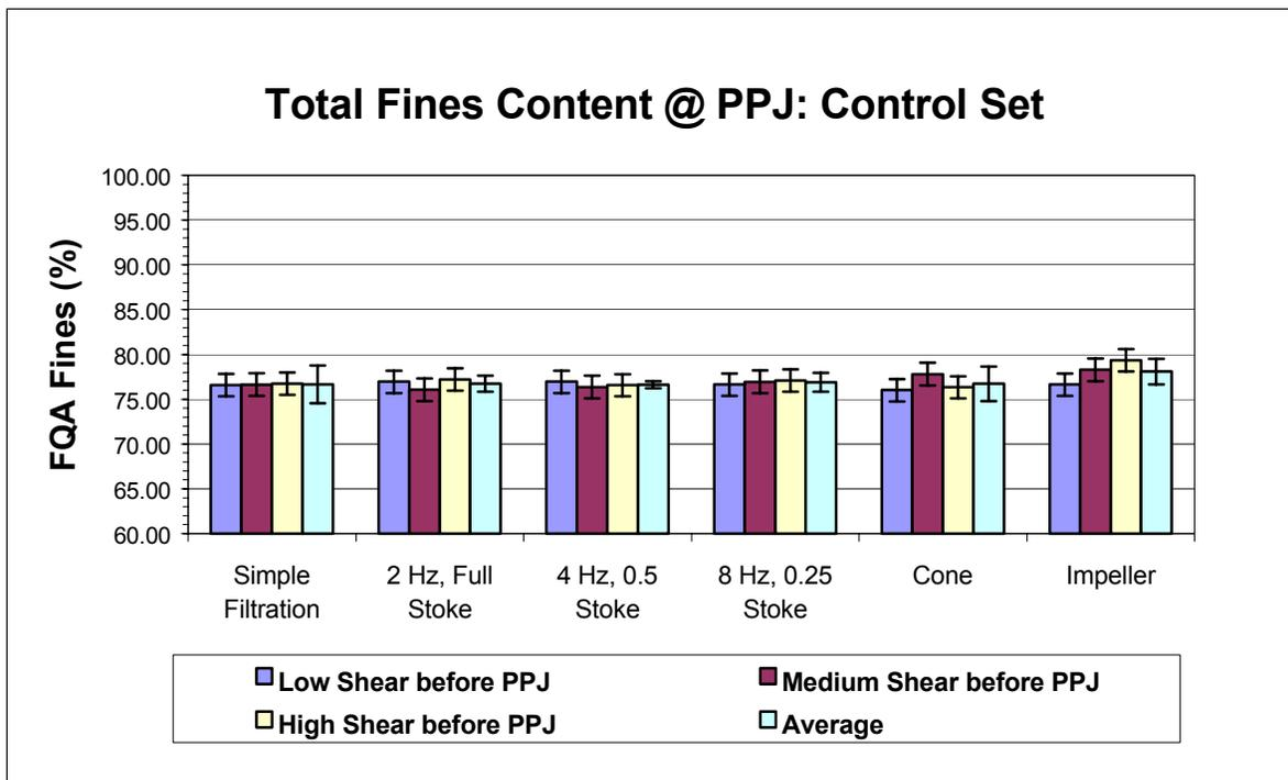
Figure 18 Total fines content resulting from different forming regimes (control set)
