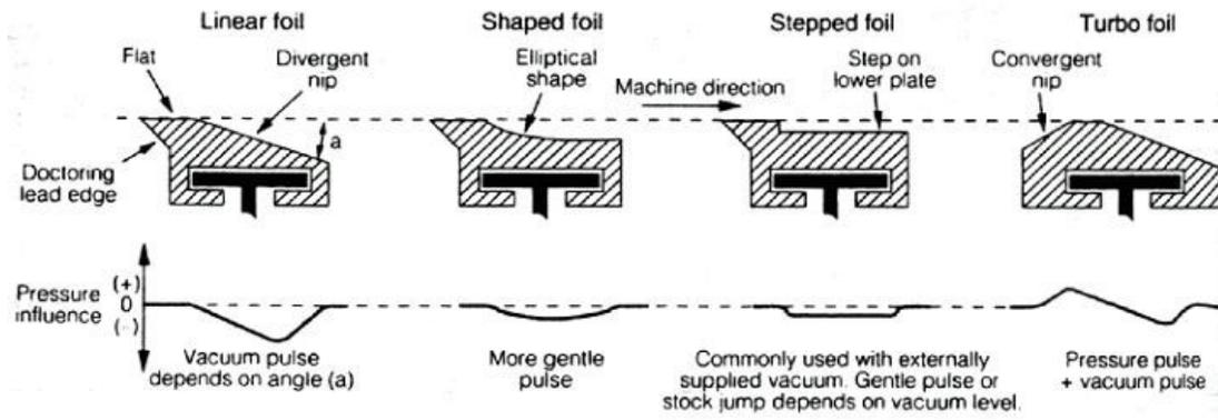
Figure 4 Hydrofoil shapes and associated pulse actions (17)
