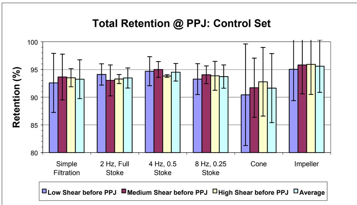
Figure 17 Total retention of different forming regimes (control set)
