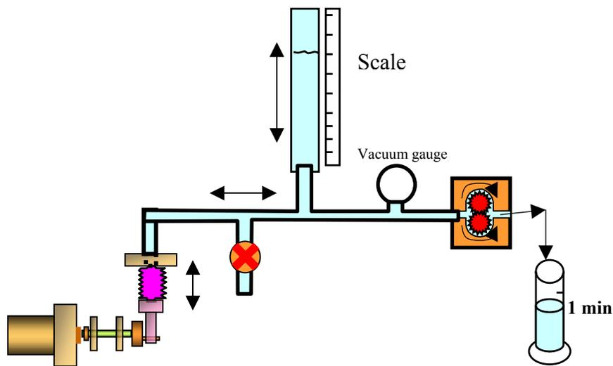
Figure13 Equipment set-up for calibrating pulsation effect
