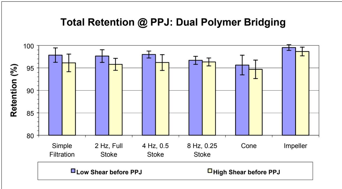
Figure 24 Total retention of different forming regimes (dual polymer bridging)
