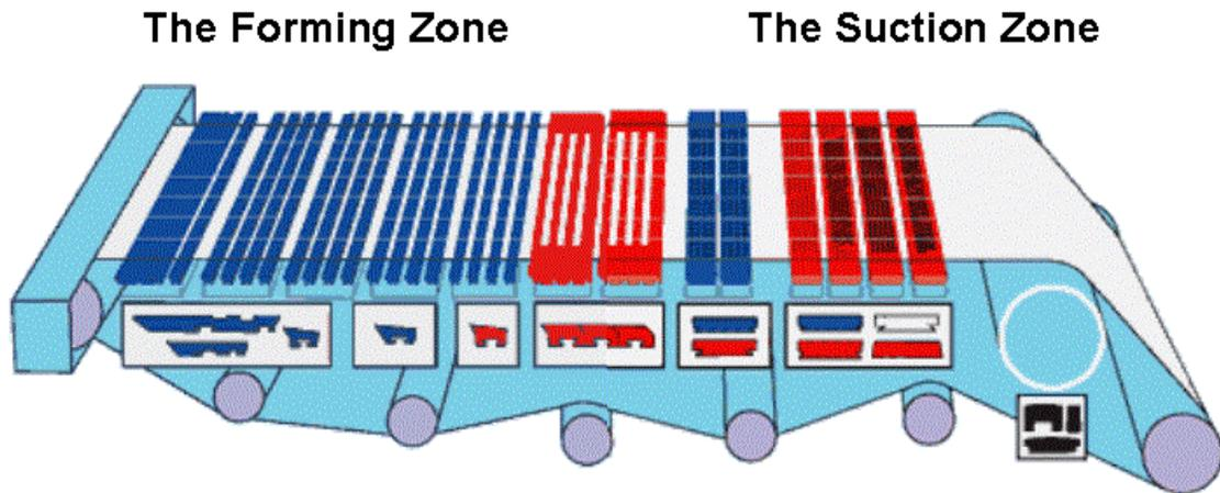
Figure 2 Two main dewatering zones on a Fourdrinier paper machine (16)
