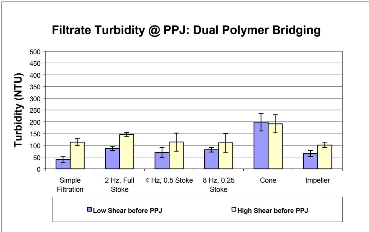
Figure 23 Turbidity results of different forming regimes (dual polymer bridging)
