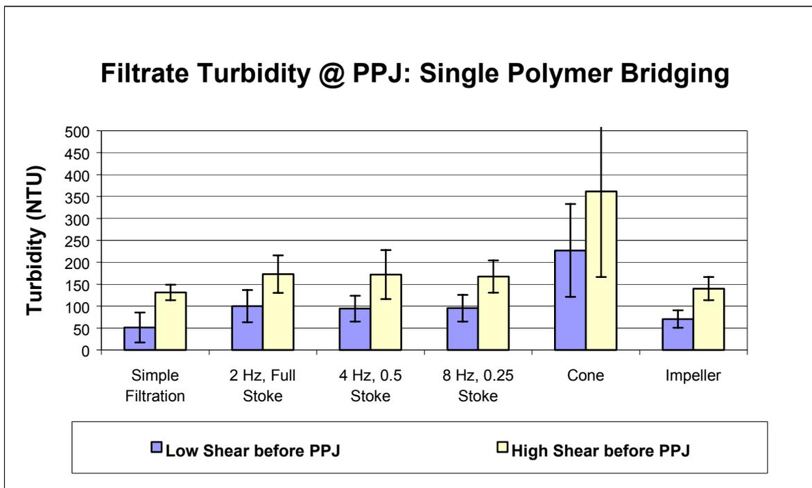
Figure 20 Turbidity results of different forming regimes (single polymer bridging)
