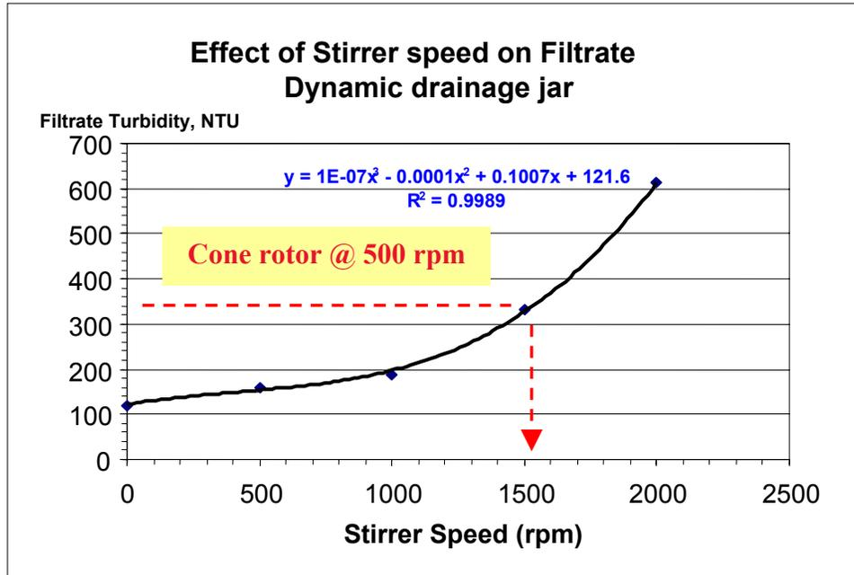
Figure 15 Calibration of the inverted cone speed with the typical stirrer
