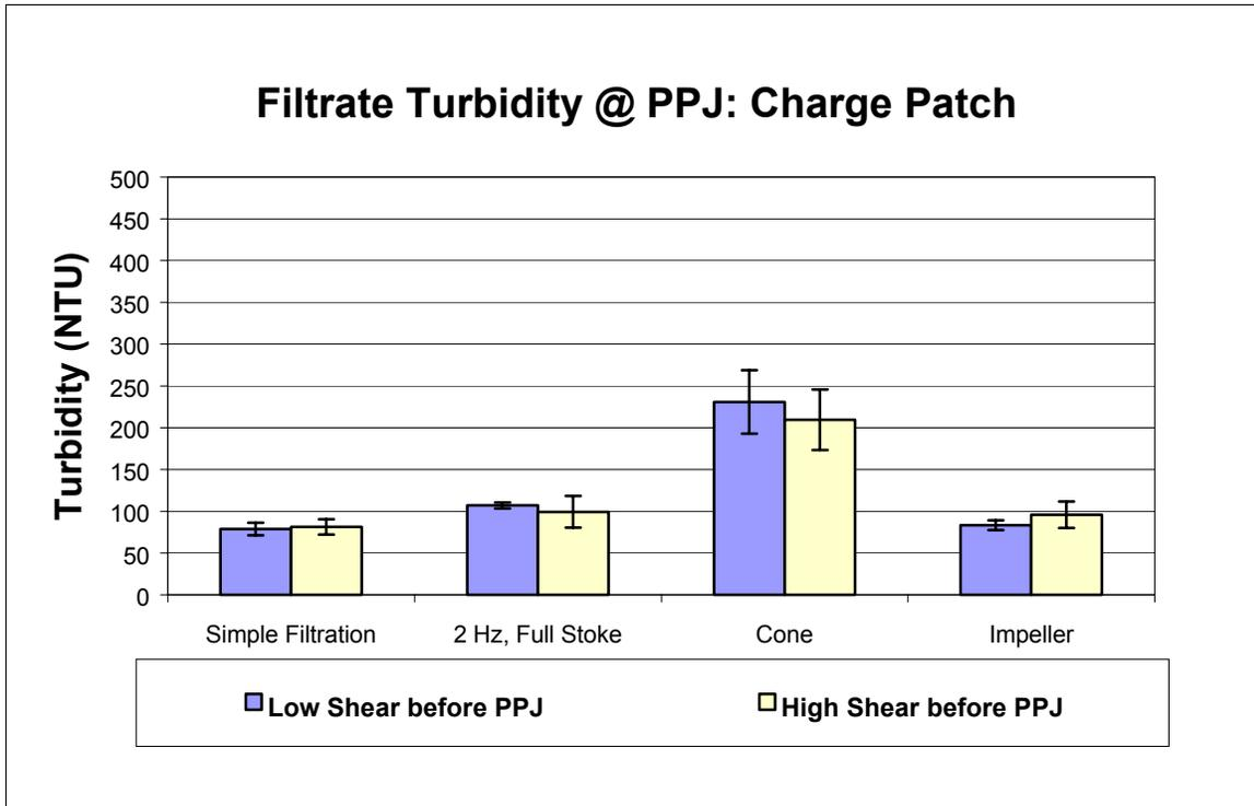
Figure 29 Turbidity results of different forming regimes (charge patch system)
