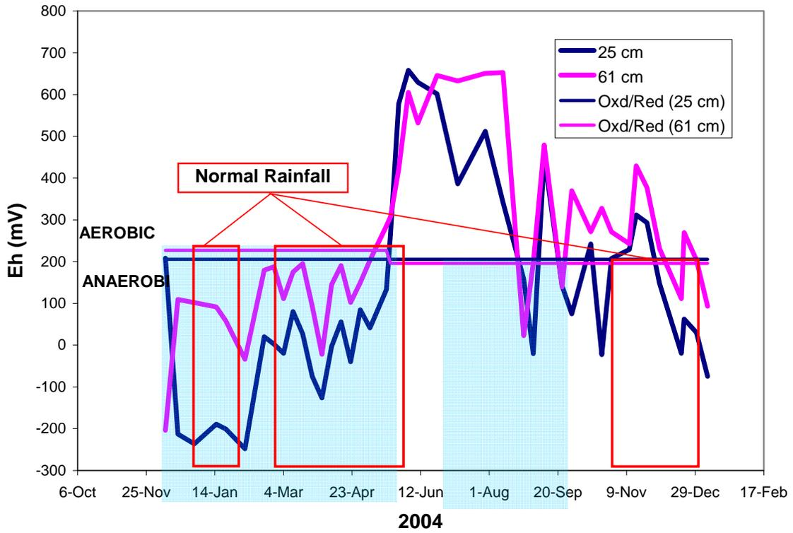
Figure 4.9. Redox potential for the control surface treatment at the 25 and 61 cm depths. The shaded areas represent periods of saturation. The HSTS is met when there is saturation and reduction during periods of normal rainfall.
