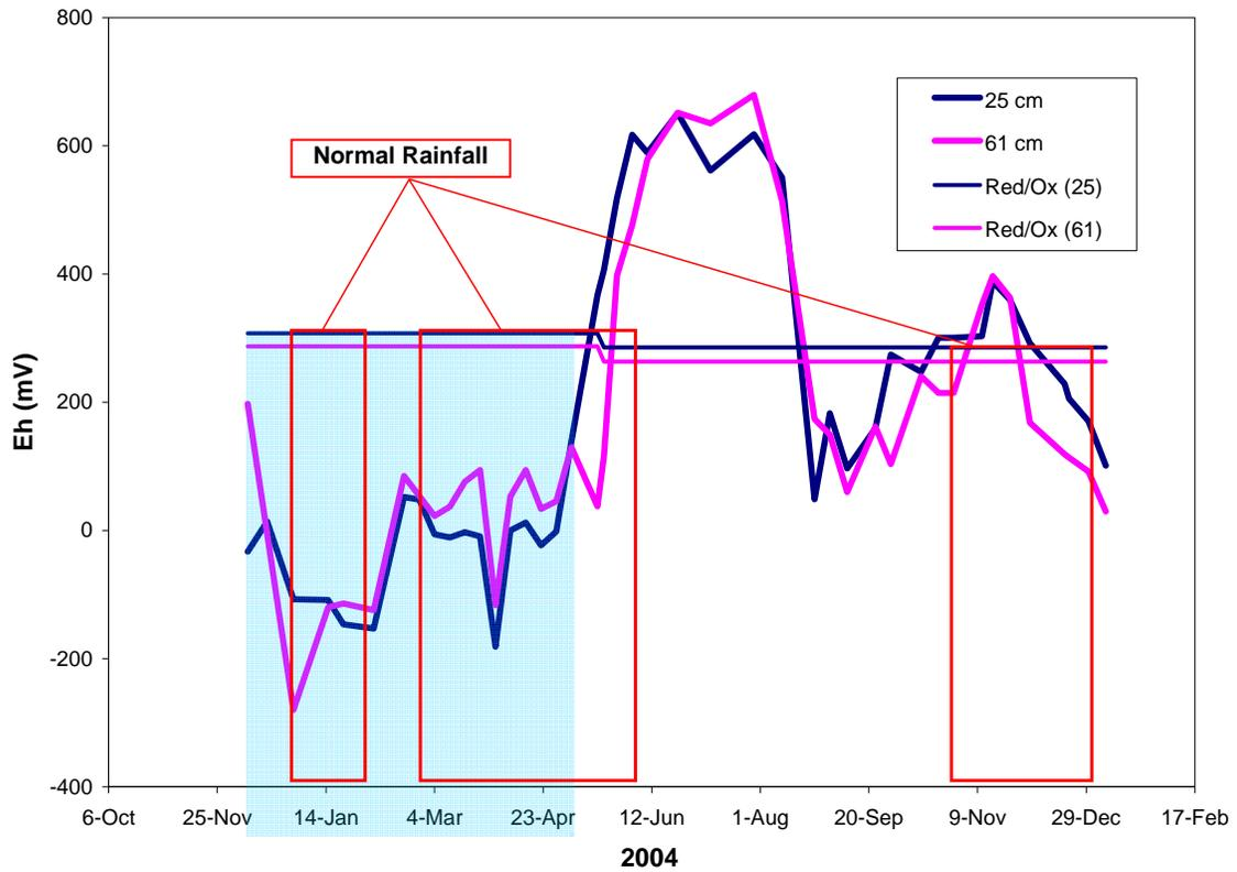
Figure 4.10. Redox potential for the micro-high in the reference site at the 25 and 61 cm depths. The shaded areas represent periods of saturation. The HSTS is met when there is saturation and reduction during periods of normal rainfall.
