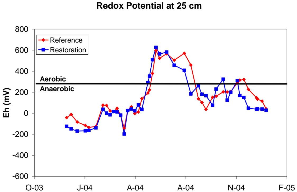
Figure 4.3: Composite redox potential for the restored and reference site at a depth of 25 cm.
