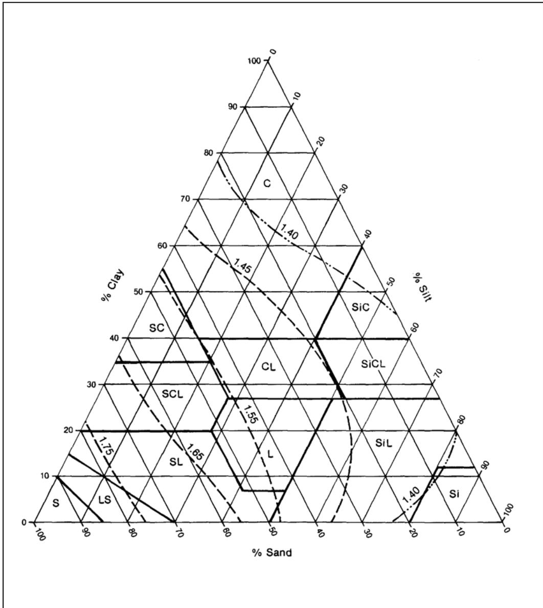
Figure 4.1: Bulk density values ( $\text{g cm}^{-3}$ ) that restrict root growth for different textural classes. Data were developed by Daddow and Warrington (1983).
