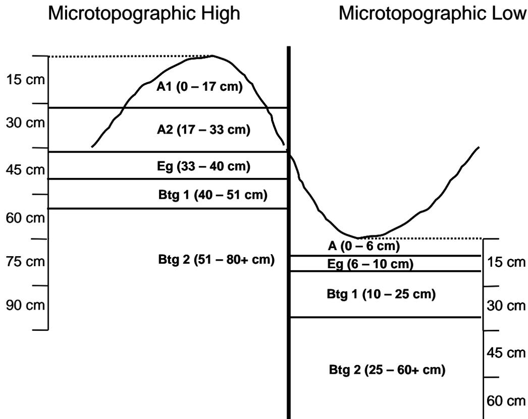
Figure 3.5. Example of how one soil pit was used to perform two profile descriptions. One description characterized the micro-topographic high and the other characterized the micro-topographic low.
