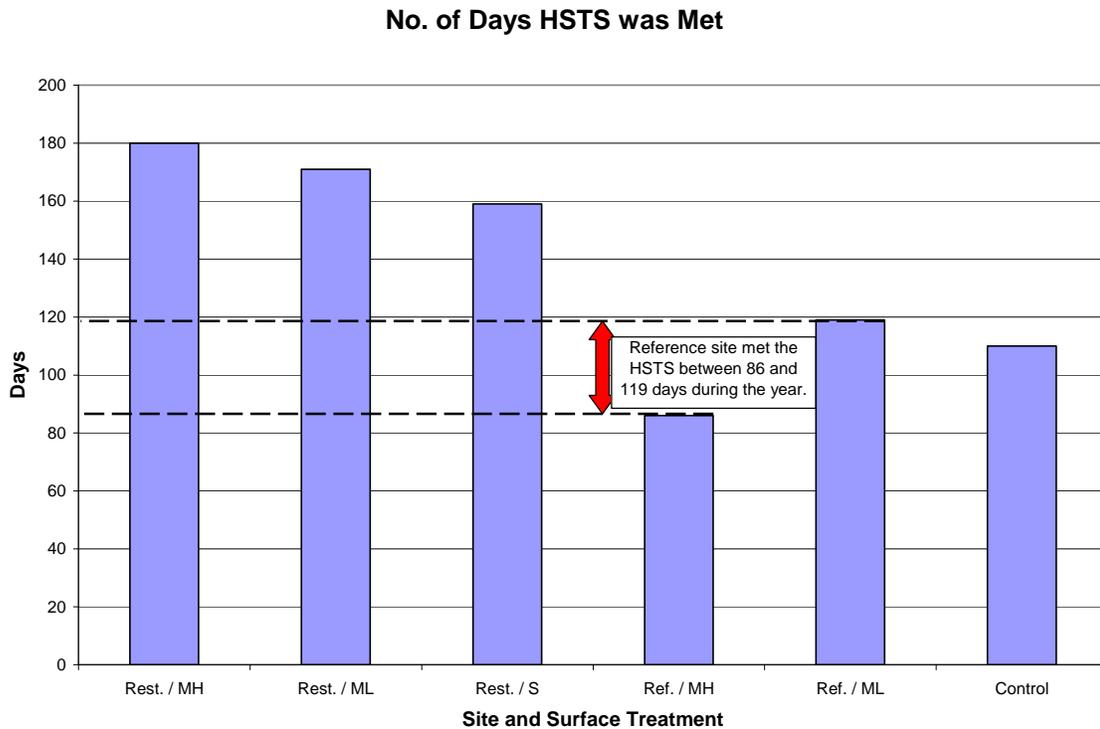
Figure 4.12. Total number of days each surface treatment successfully met all requirements for the HSTS.
