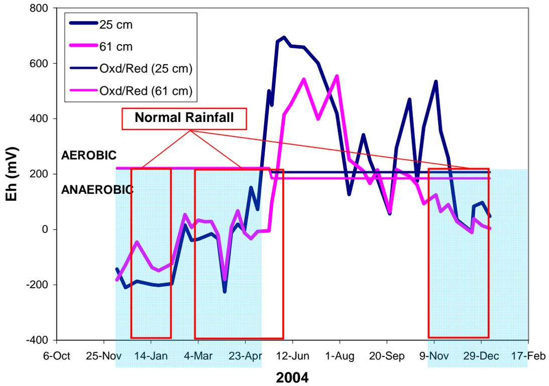
Figure 4.7. Redox potential for the restored (2003) micro-high surface treatment at the 25 and 61 cm depths. The shaded areas represent periods of saturation. The HSTS is met when there is saturation and reduction during periods of normal rainfall.
