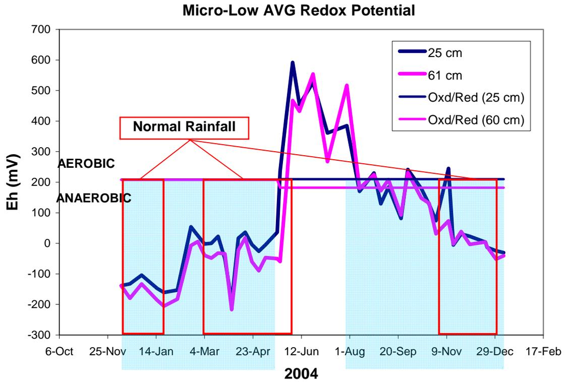
Figure 4.8. Redox potential for the restored (2003) micro-low surface treatment at the 25 and 61 cm depths. The shaded areas represent periods of saturation. The HSTS is met when there is saturation and reduction during periods of normal rainfall.
