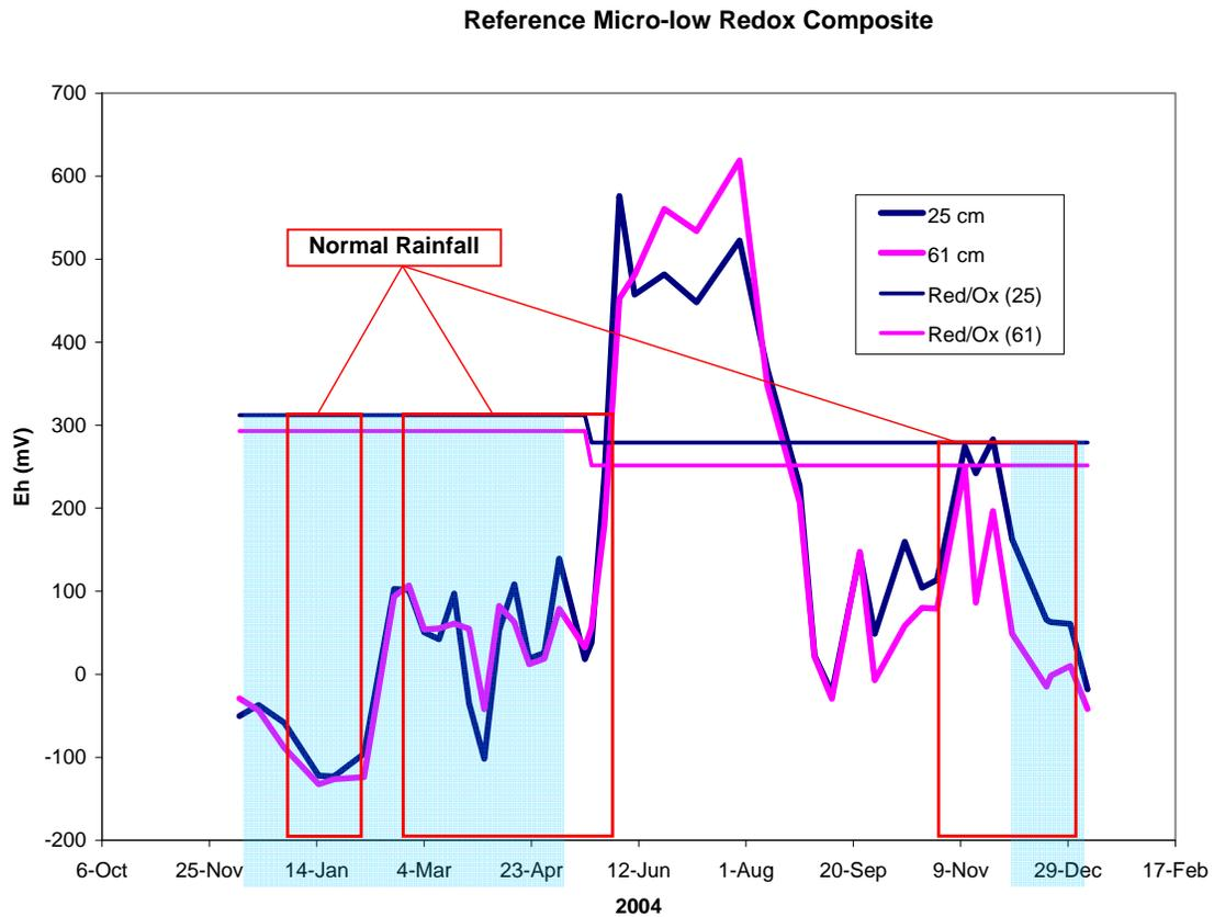
Figure 4.11. Redox potential for the micro-low in the reference site at the 25 and 61 cm depths. The shaded areas represent periods of saturation. The HSTS is met when there is saturation and reduction during periods of normal rainfall.
