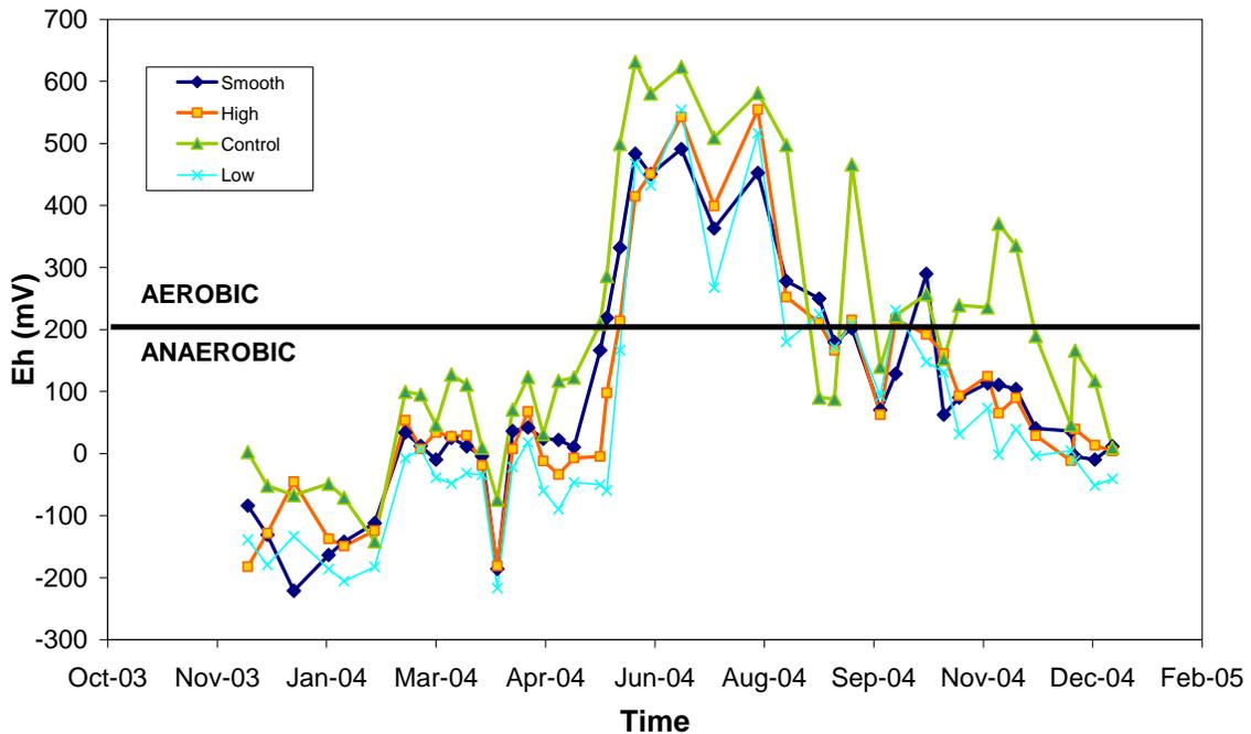
Figure 4.2: Mean redox potential of both depths (25 and 61 cm) for each surface treatment in the restored site 2003.
