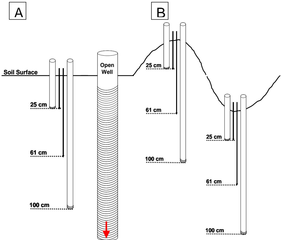
Figure 3.6. Hydric soil technical standard instrumentation for a smooth (A) and microtopographic (B) plot. Each HSTS monitoring station includes: two piezometers and five redox electrodes at 25 cm, five redox electrodes at 61 cm, two piezometers at 100 cm, and an open screen well to 200 cm. The contoured treatments include a HSTS monitoring
