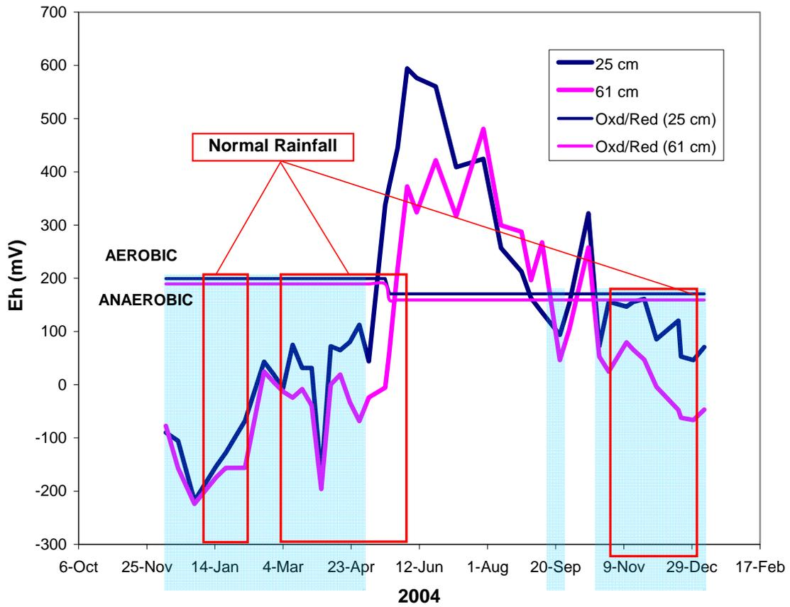
Figure 4.6. Redox potential for the restored (2003) smooth surface treatment at the 25 and 61 cm depths. The shaded areas represent periods of saturation. The HSTS is met when there is saturation and reduction during periods of normal rainfall.
