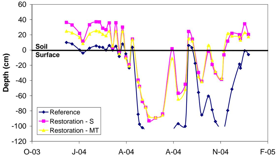
Figure 4.5. Water table fluctuations during the study period recorded by automated wells installed at a depth of 200 cm for the restored and reference site
