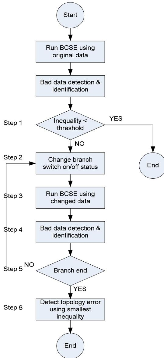
**Figure 22. Flowchart of Method II Algorithm**
