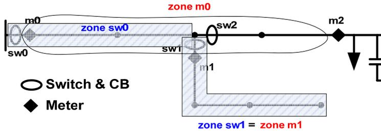
Figure 20. Zone defined by switches and meters in a feeder
