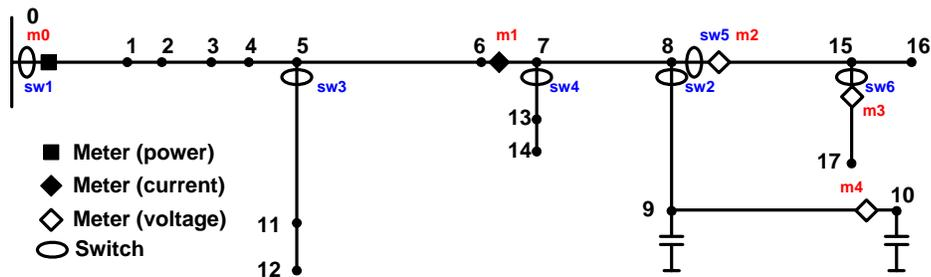
Figure 23. One-line diagram of the test feeder with switch
