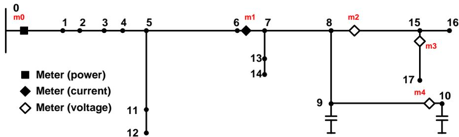
Figure 5. One-line diagram of reduced feeder
