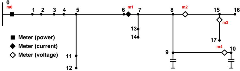
Figure 2. One-line diagram of reduced feeder
