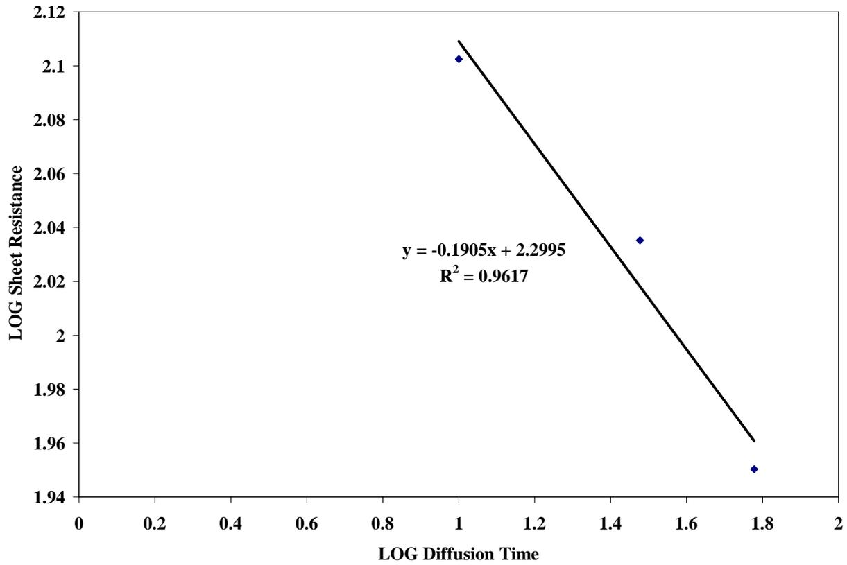
Figure 4.3 – Plot of log sheet resistance vs. log diffusion time for a constant diffusion temperature of 900°C
