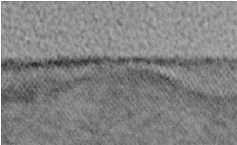
Cross-Sectional TEM Image for Sample B4 (900°C/30 min./N<sub>2</sub>O<sub>2</sub>)
