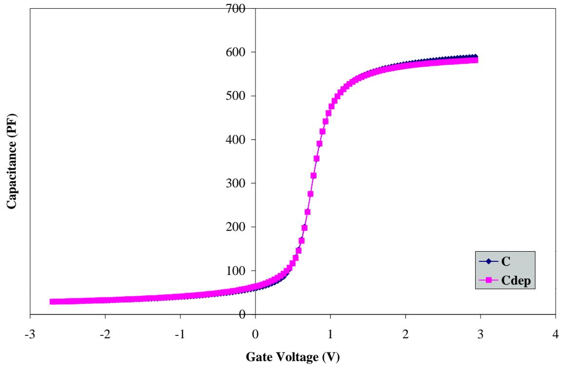
High Frequency CV Curve for Wafer A4 (800°C/20 min./N<sub>2</sub>O<sub>2</sub>)
