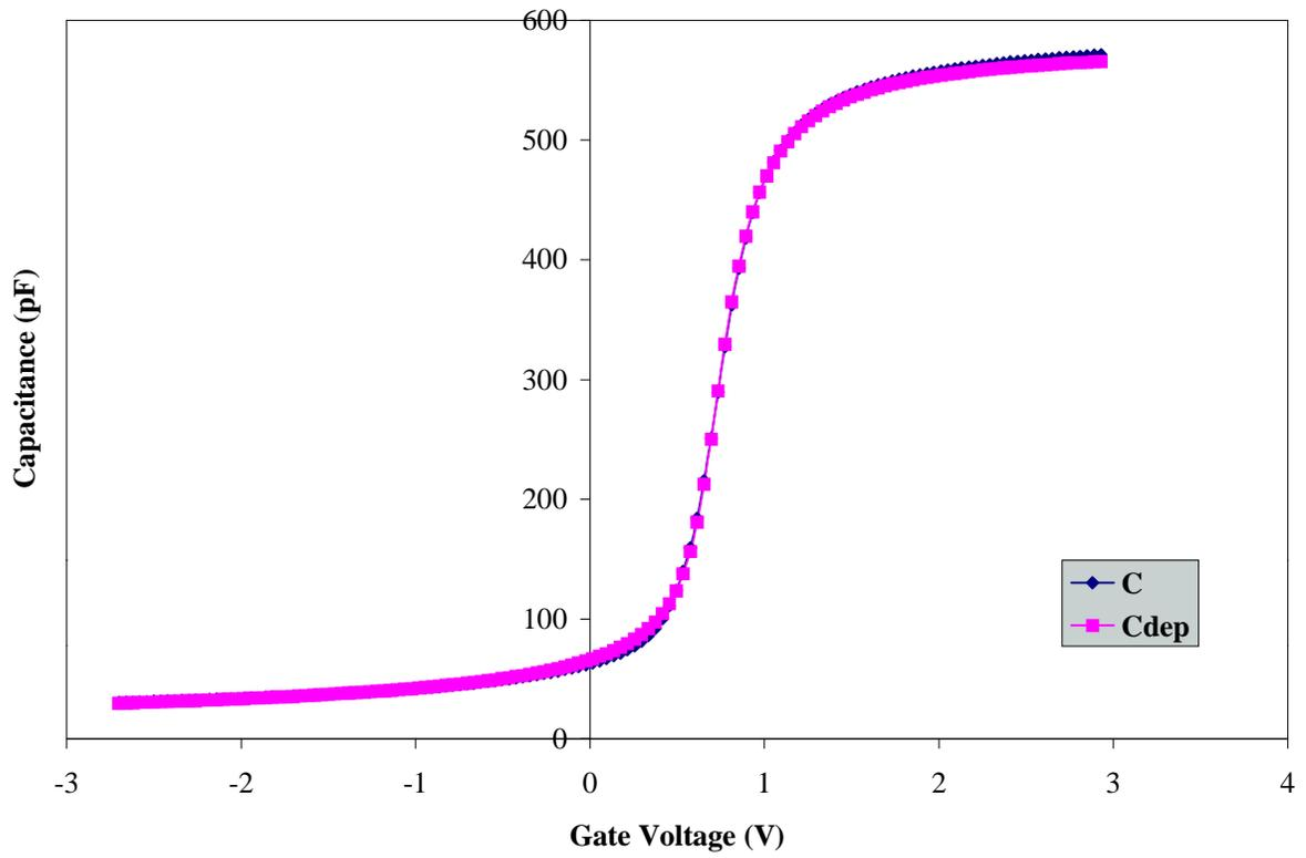
High Frequency CV Curve for Wafer A1 (800°C/45 min./N<sub>2</sub>)
