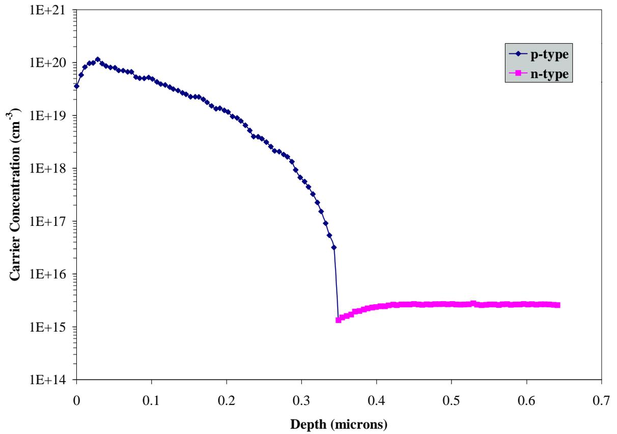
SRA Profile for Wafer B2 (900°C/60 min./N<sub>2</sub>O<sub>2</sub>)
