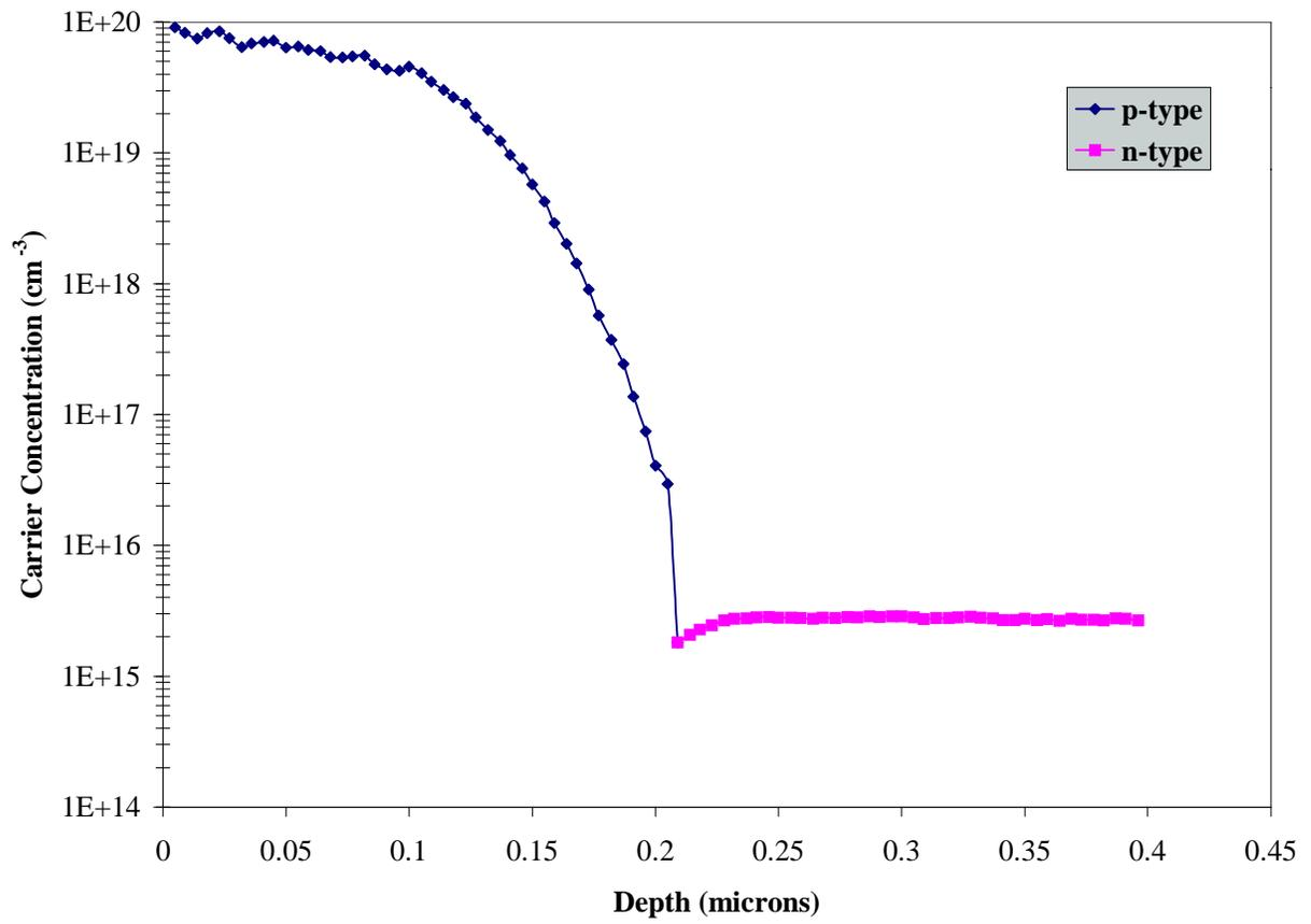
SRA Profile for Wafer B5 (900°C/30 min./N<sub>2</sub>)
