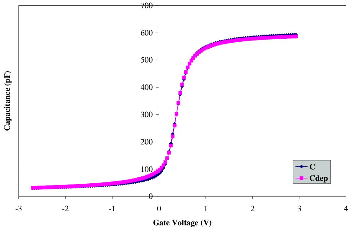
High Frequency CV Curve for Wafer B7 (900°C/10 min./N<sub>2</sub>)
