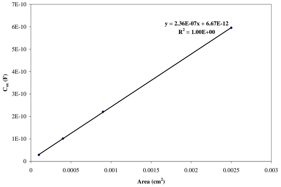
C<sub>ox</sub> vs. Capacitor Area Plot for Wafer B2 (900°C/60 min./N<sub>2</sub>O<sub>2</sub>)
