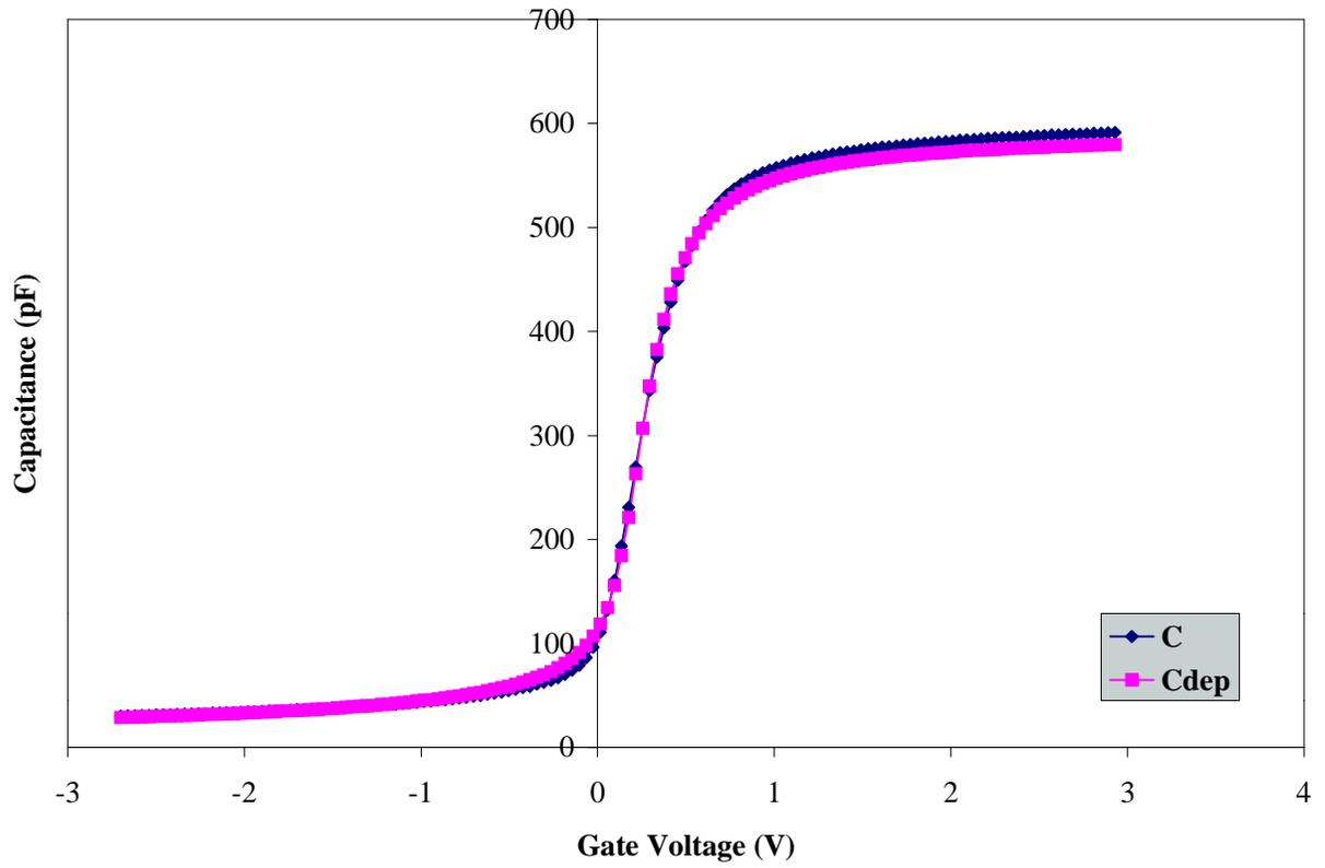
High Frequency CV Curve for Wafer B4 (900°C/30 min/N<sub>2</sub>O<sub>2</sub>)
