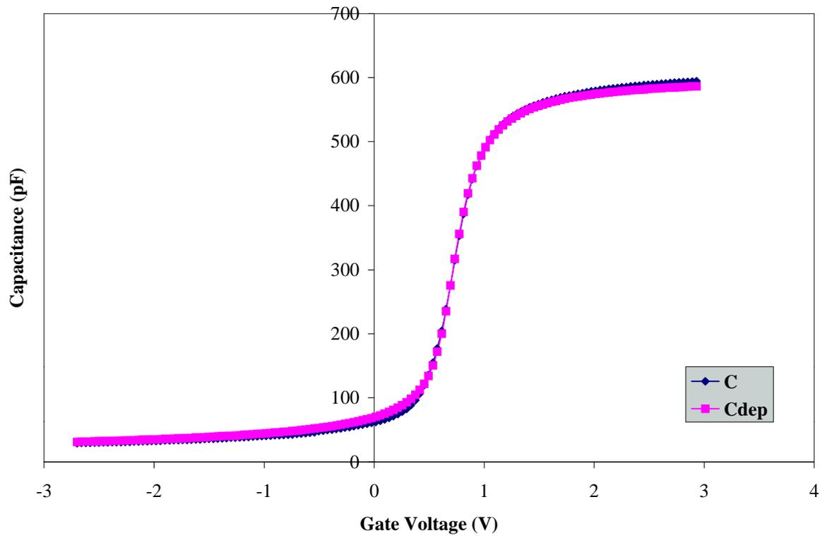
High Frequency CV Curve for Wafer A3 (800°C/20 min./N<sub>2</sub>)
