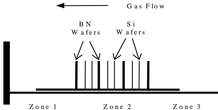
Figure 2.1 – Wafer arrangement in furnace for boron nitride solid source diffusion
