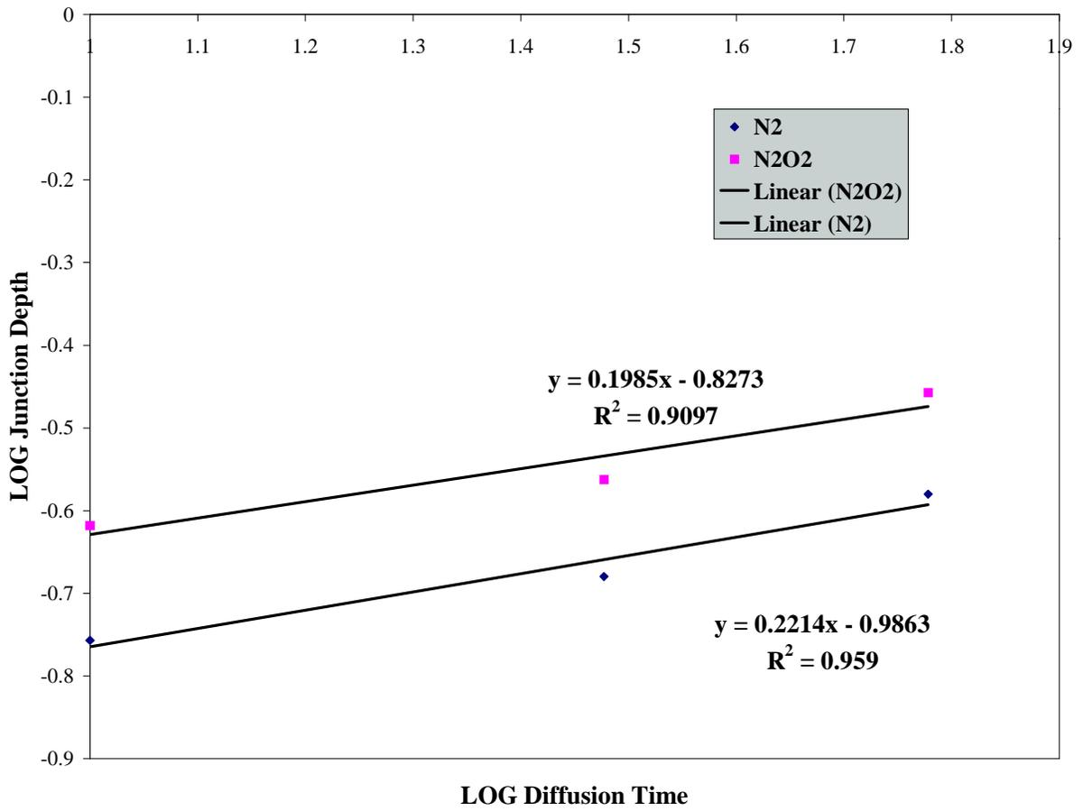
Figure 4.5 – Plot of log junction depth vs. log diffusion time for a 900°C diffusion temperature
