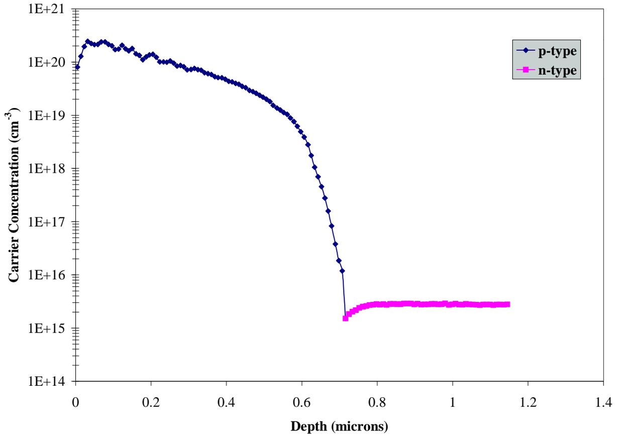
SRA Profile for Wafer C1 (1000°C/45 min./N<sub>2</sub>)
