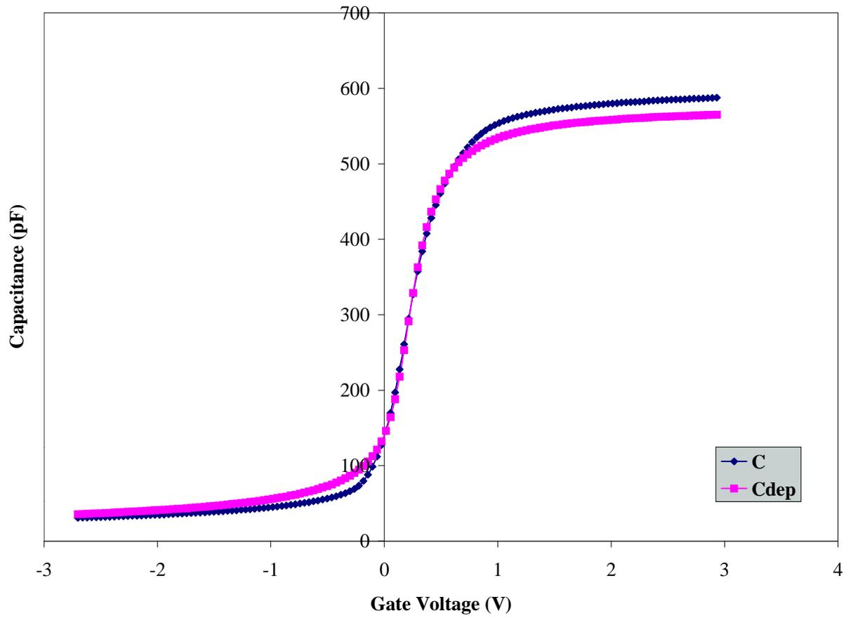
High Frequency CV Curve for Wafer B1 (900°C/60 min./N<sub>2</sub>)
