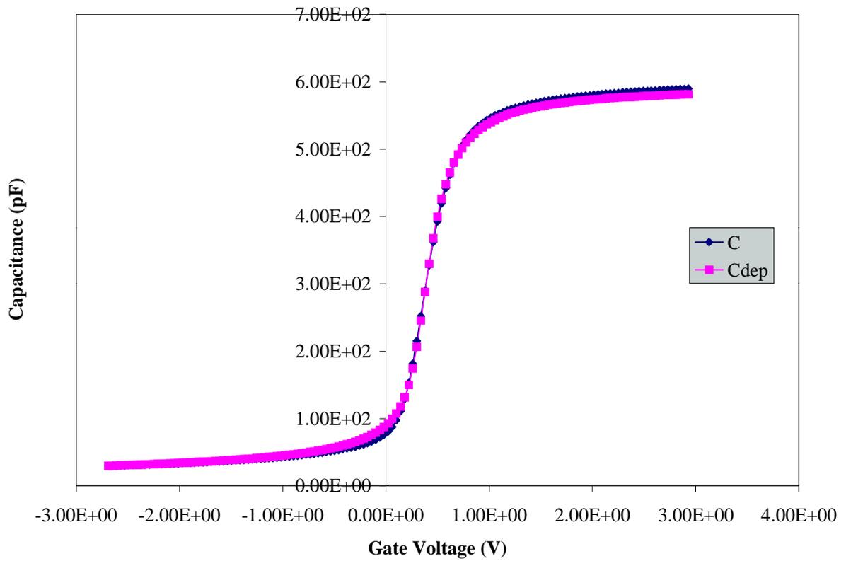
Figure 4.7 – High frequency CV curve for 900°C/30 min./N<sub>2</sub> doped wafer
