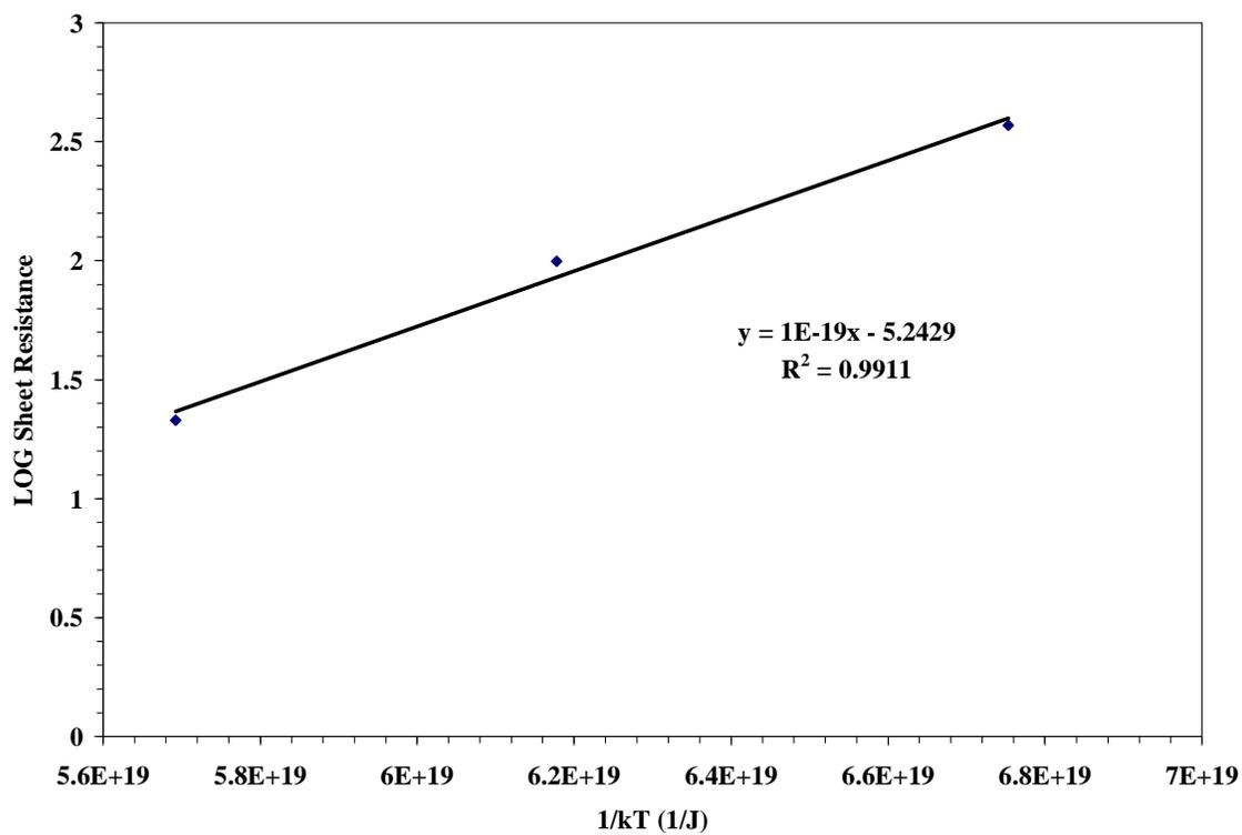
Figure 4.4 - Plot of log sheet resistance vs. 1/kT for a constant diffusion time of 45 minutes
