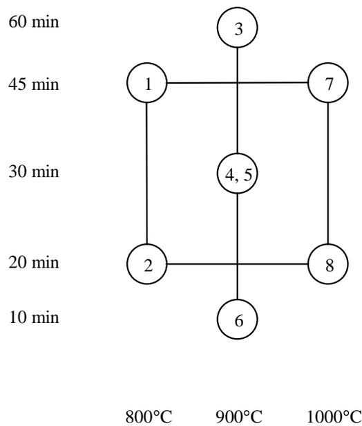
Figure 3.1 – Schematic of the chosen experimental points in the design
