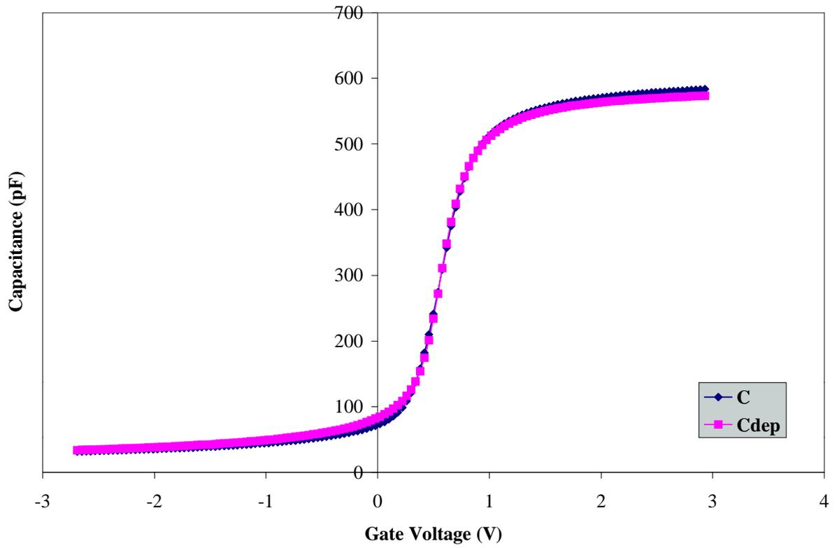
High Frequency CV Curve for Wafer A2 (800°C/45 min./N<sub>2</sub>O<sub>2</sub>)
