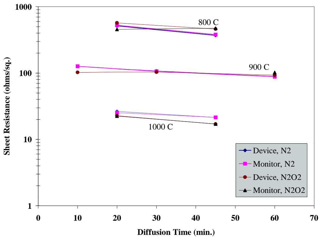
Figure 4.2 – Plot of four-point probe sheet resistance vs. diffusion time for all diffusion runs
