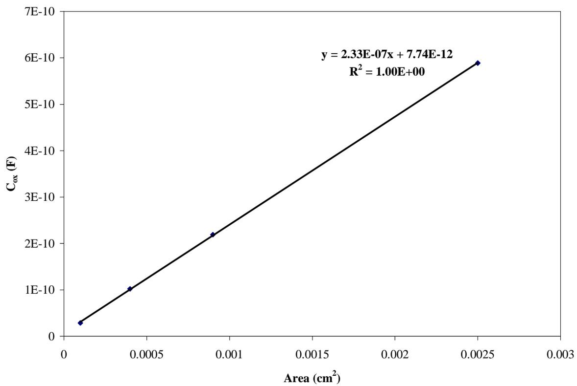
C<sub>ox</sub> vs. Capacitor Area Plot for Wafer B5 (900°C/30 min./N<sub>2</sub>)
