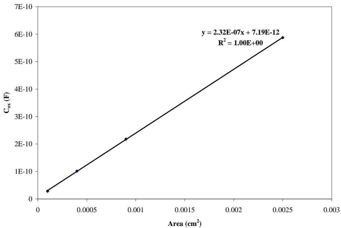
C<sub>ox</sub> vs. Capacitor Area Plot for Wafer B1 (900°C/60 min./N<sub>2</sub>)
