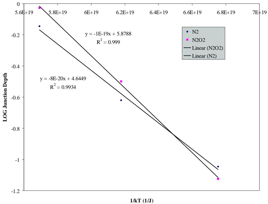
Figure 4.6 – Plot of log junction depth vs. 1/kT for a constant diffusion time of 45 minutes
