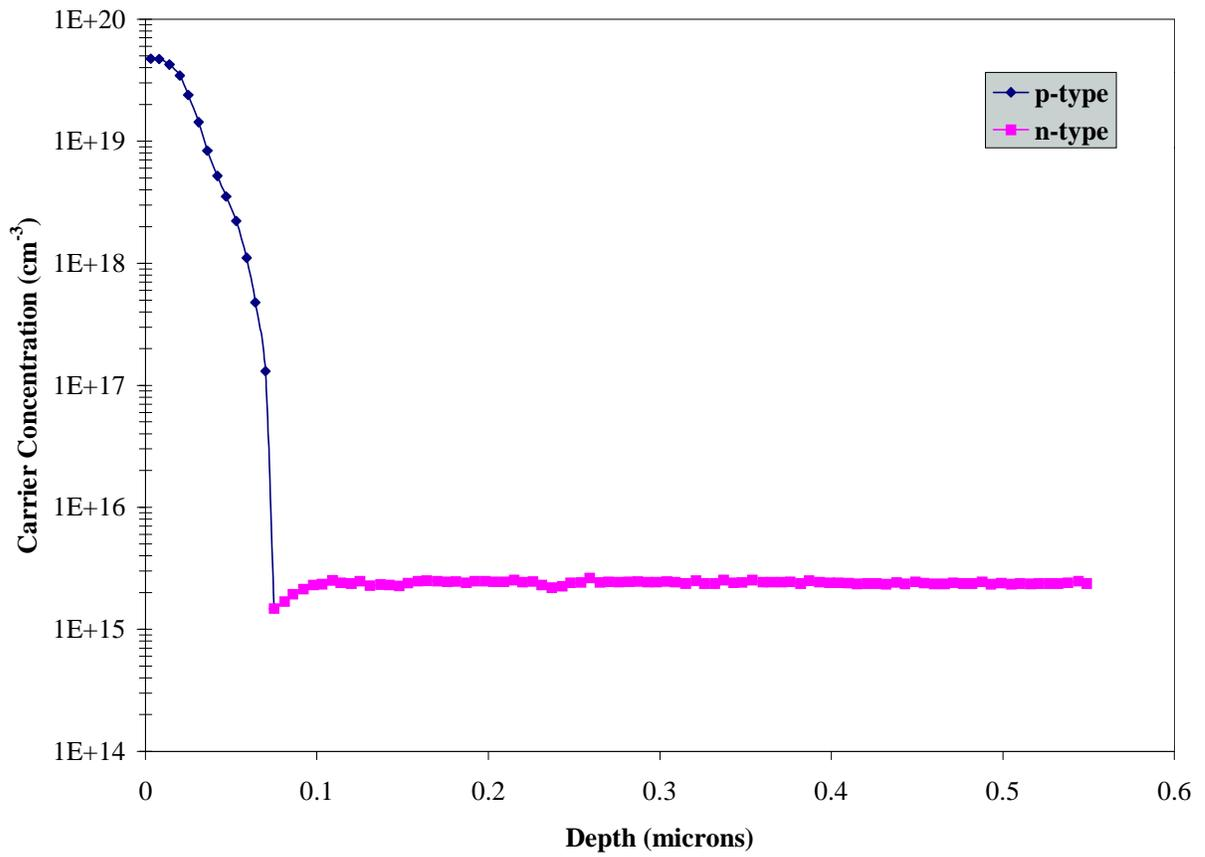
SRA Profile for Wafer A2 (800°C/45 min./N<sub>2</sub>O<sub>2</sub>)
