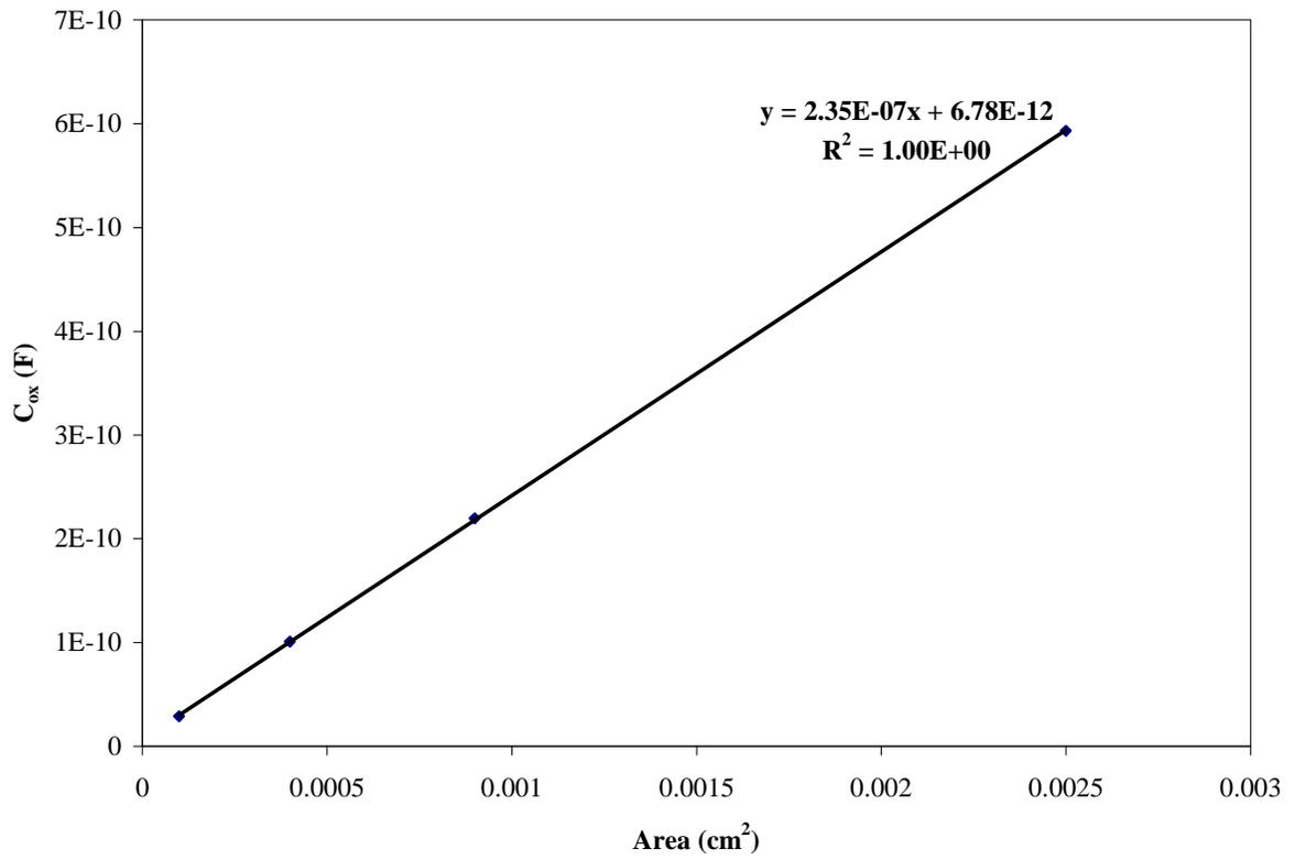
C<sub>ox</sub> vs. Capacitor Area Plot for Wafer B7 (900°C/10 min./N<sub>2</sub>)
