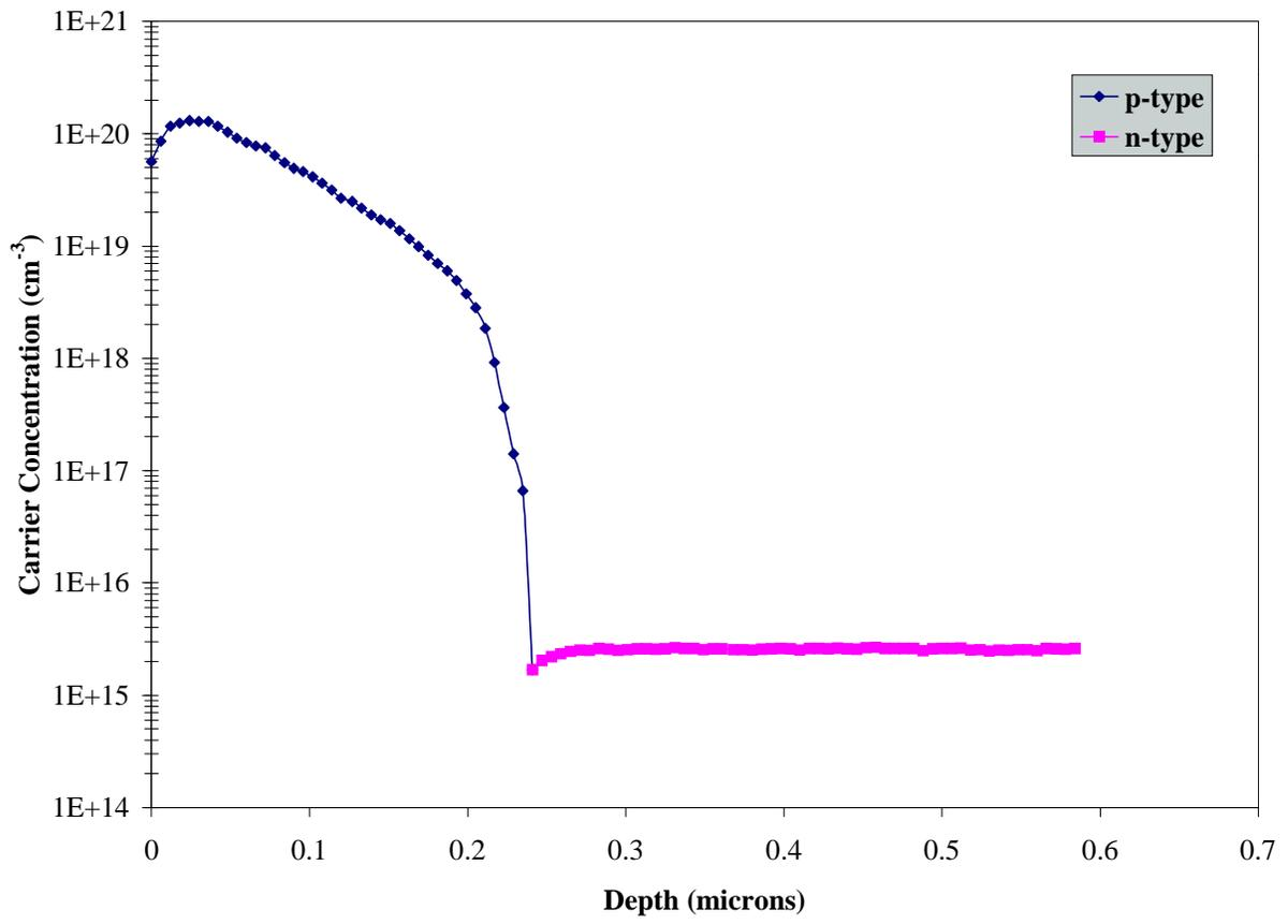
SRA Profile for Wafer B8 (900°C/10 min./N<sub>2</sub>O<sub>2</sub>)
