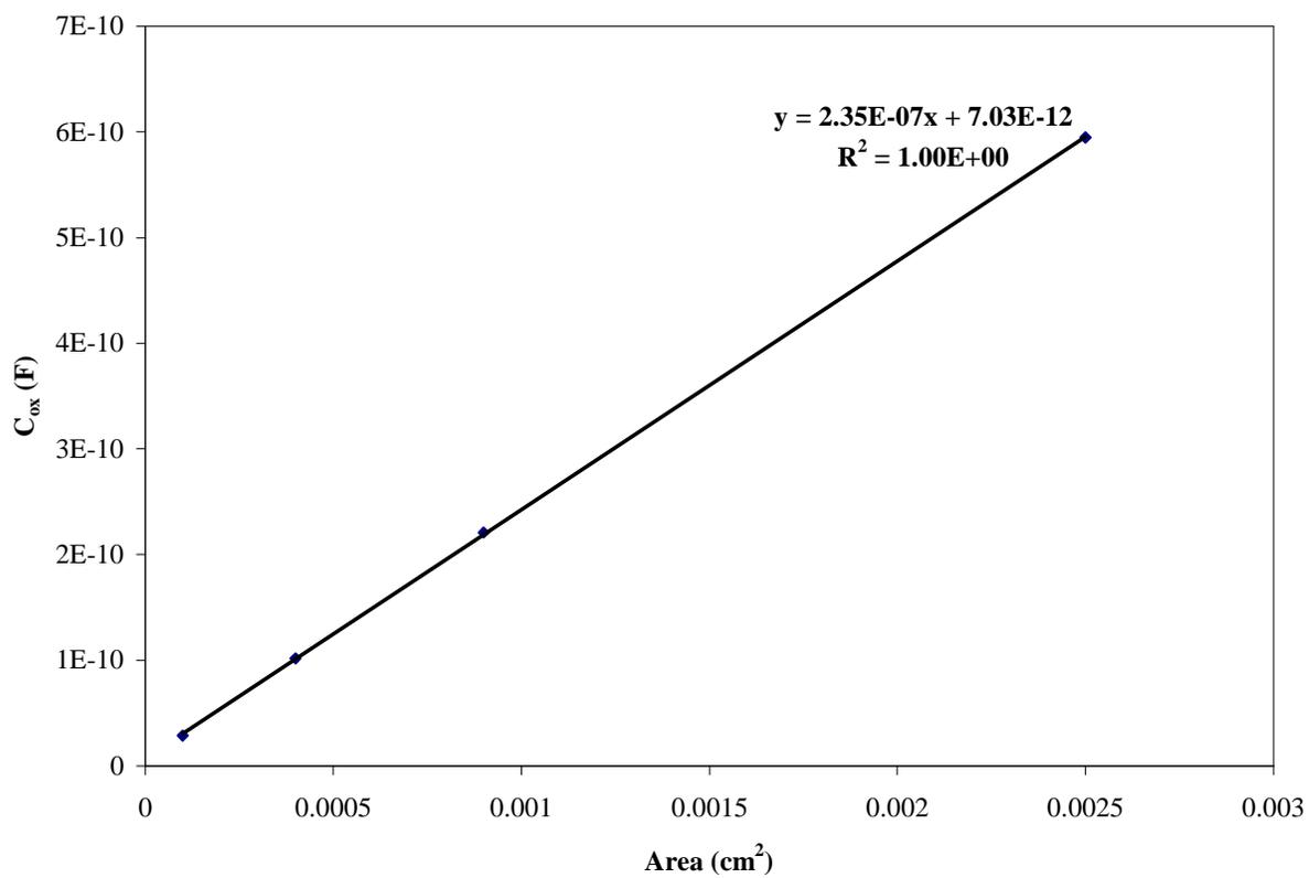
C<sub>ox</sub> vs. Capacitor Area Plot for Wafer A3 (800°C/20 min./N<sub>2</sub>)
