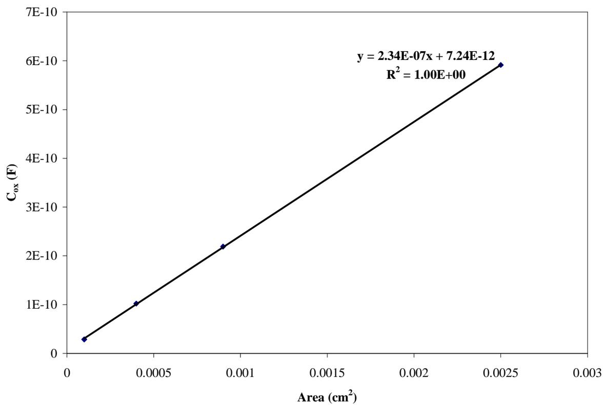
C<sub>ox</sub> vs. Capacitor Area Plot for Wafer B4 (900°C/30 min/N<sub>2</sub>O<sub>2</sub>)
