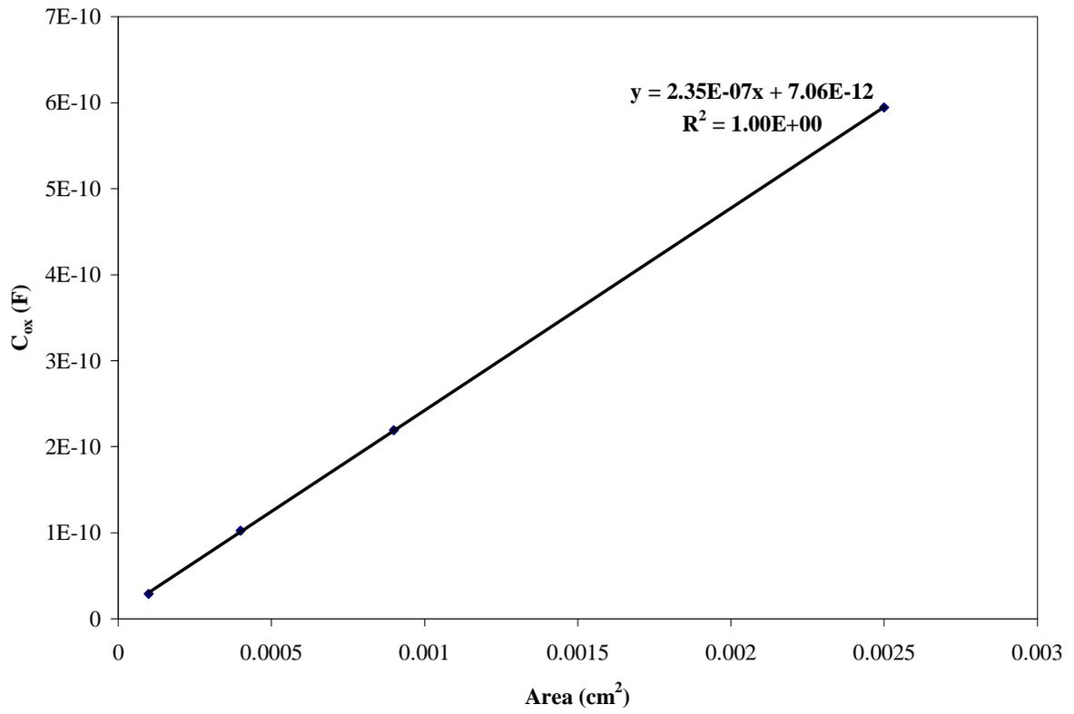
C<sub>ox</sub> vs. Capacitor Area Plot for Wafer B8 (900°C/10 min./N<sub>2</sub>O<sub>2</sub>)
