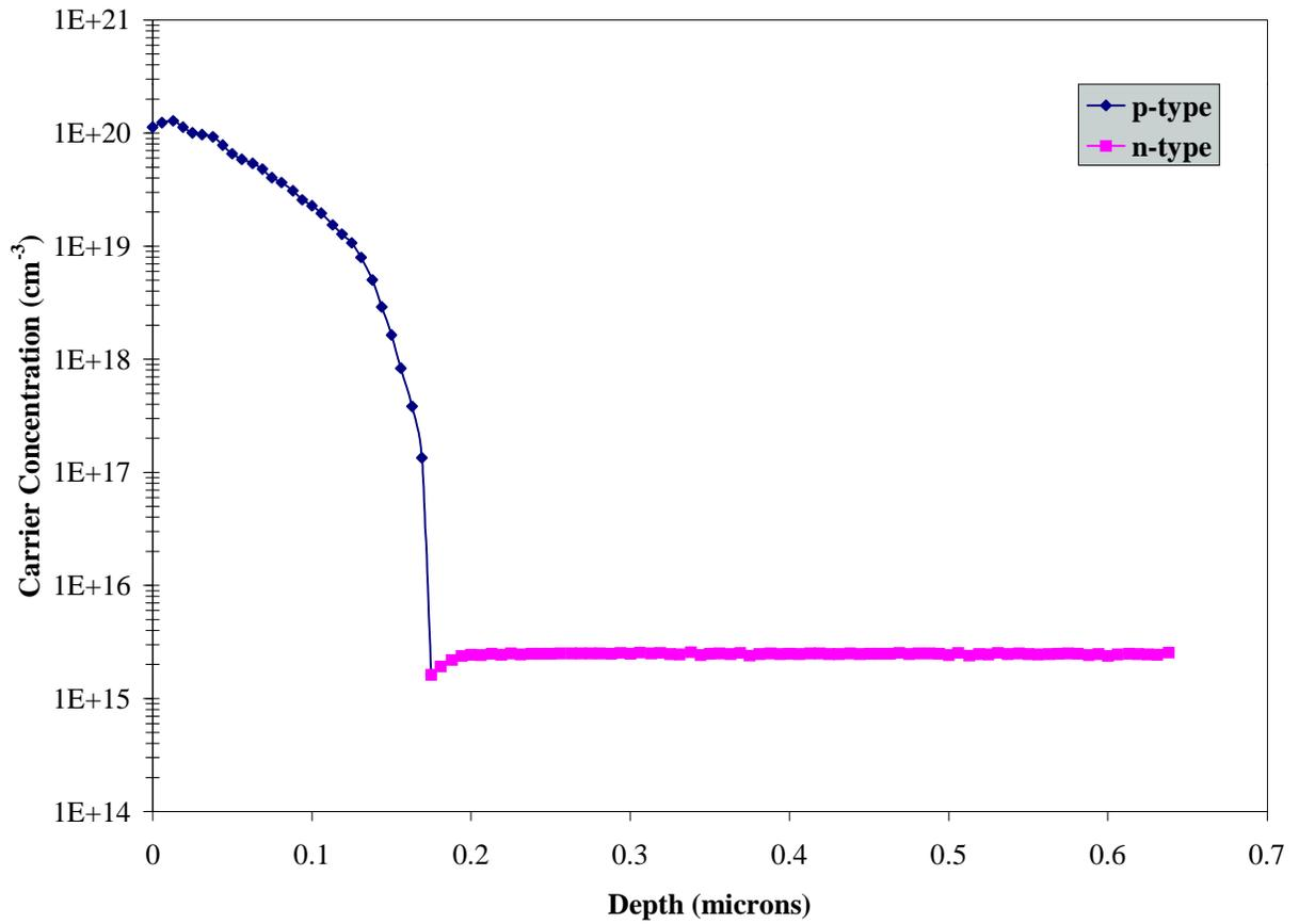
SRA Profile for Wafer B7 (900°C/10 min./N<sub>2</sub>)
