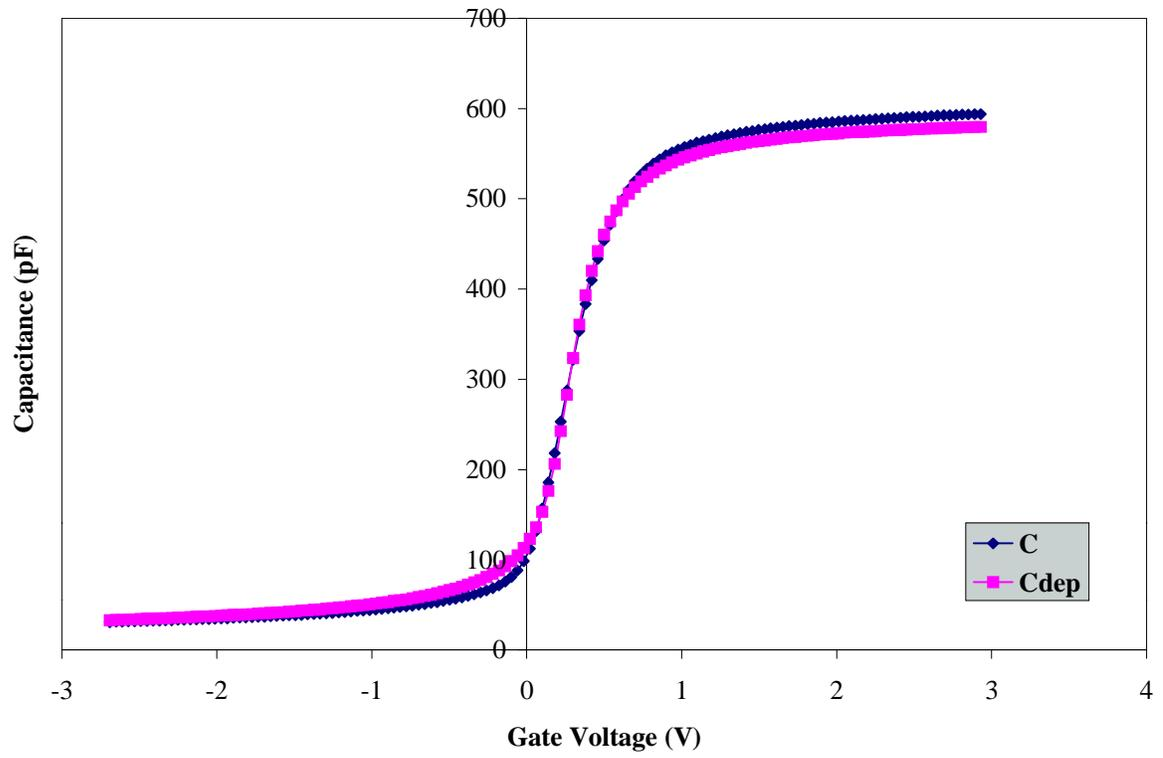
High Frequency CV Curve for Wafer B8 (900°C/10 min./N<sub>2</sub>O<sub>2</sub>)
