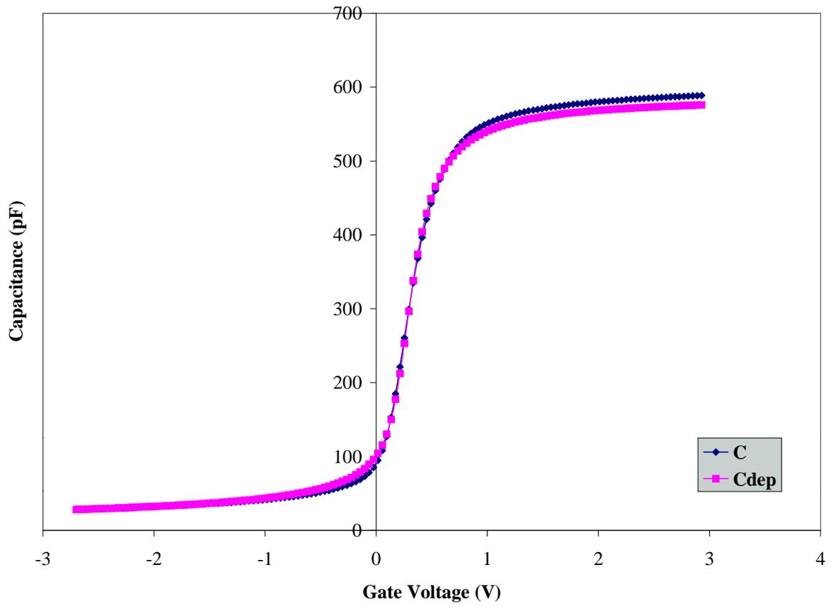
High Frequency CV Curve for Wafer B5 (900°C/30 min./N<sub>2</sub>)
