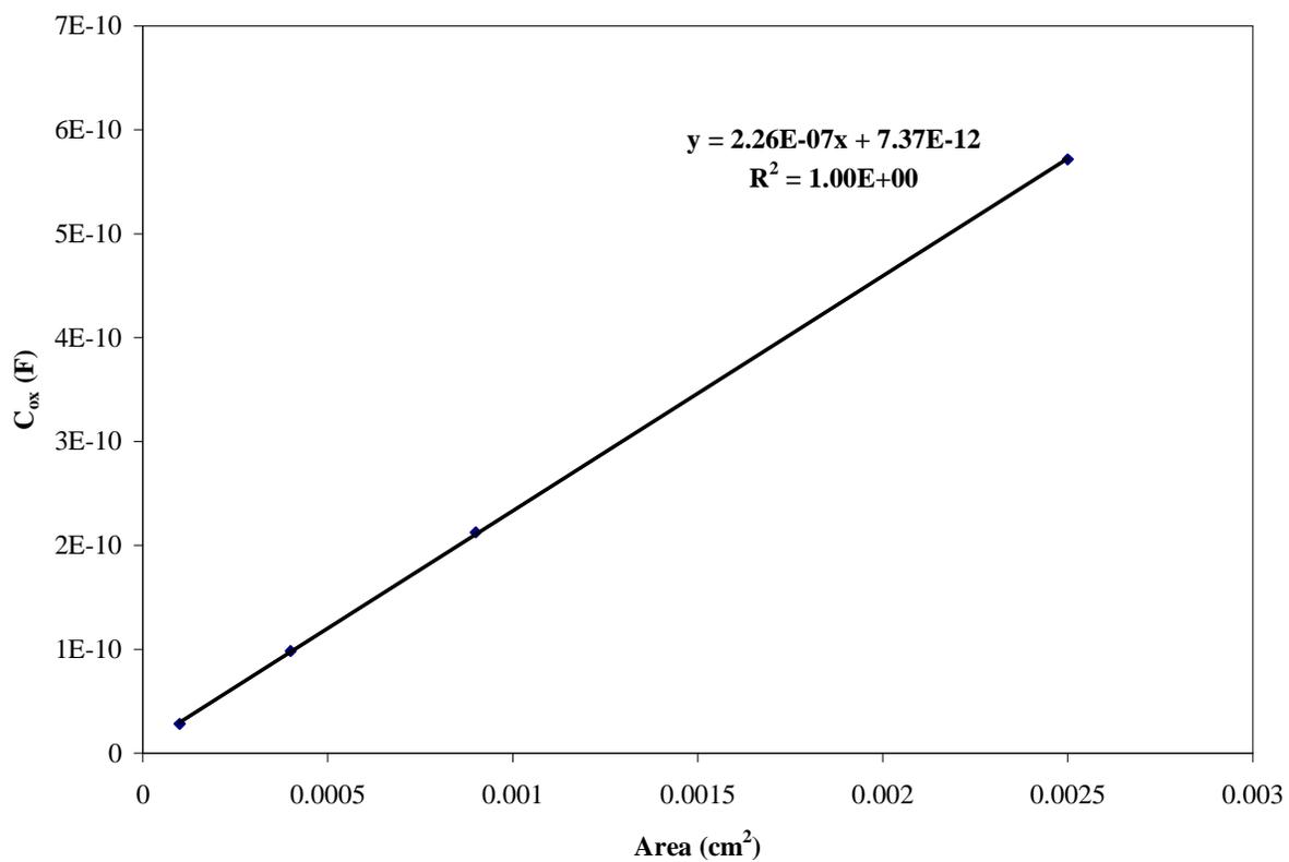
C<sub>ox</sub> vs. Capacitor Area Plot for Wafer A1 (800°C/45 min./N<sub>2</sub>)
