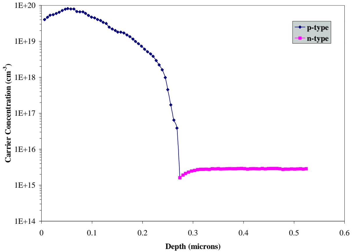
SRA Profile for Wafer B4 (900°C/30 min/N<sub>2</sub>O<sub>2</sub>)
