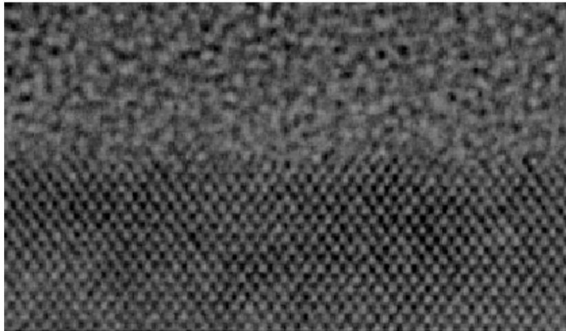
Cross-Sectional TEM Image for Sample A1 (800°C/45 min./N<sub>2</sub>)
