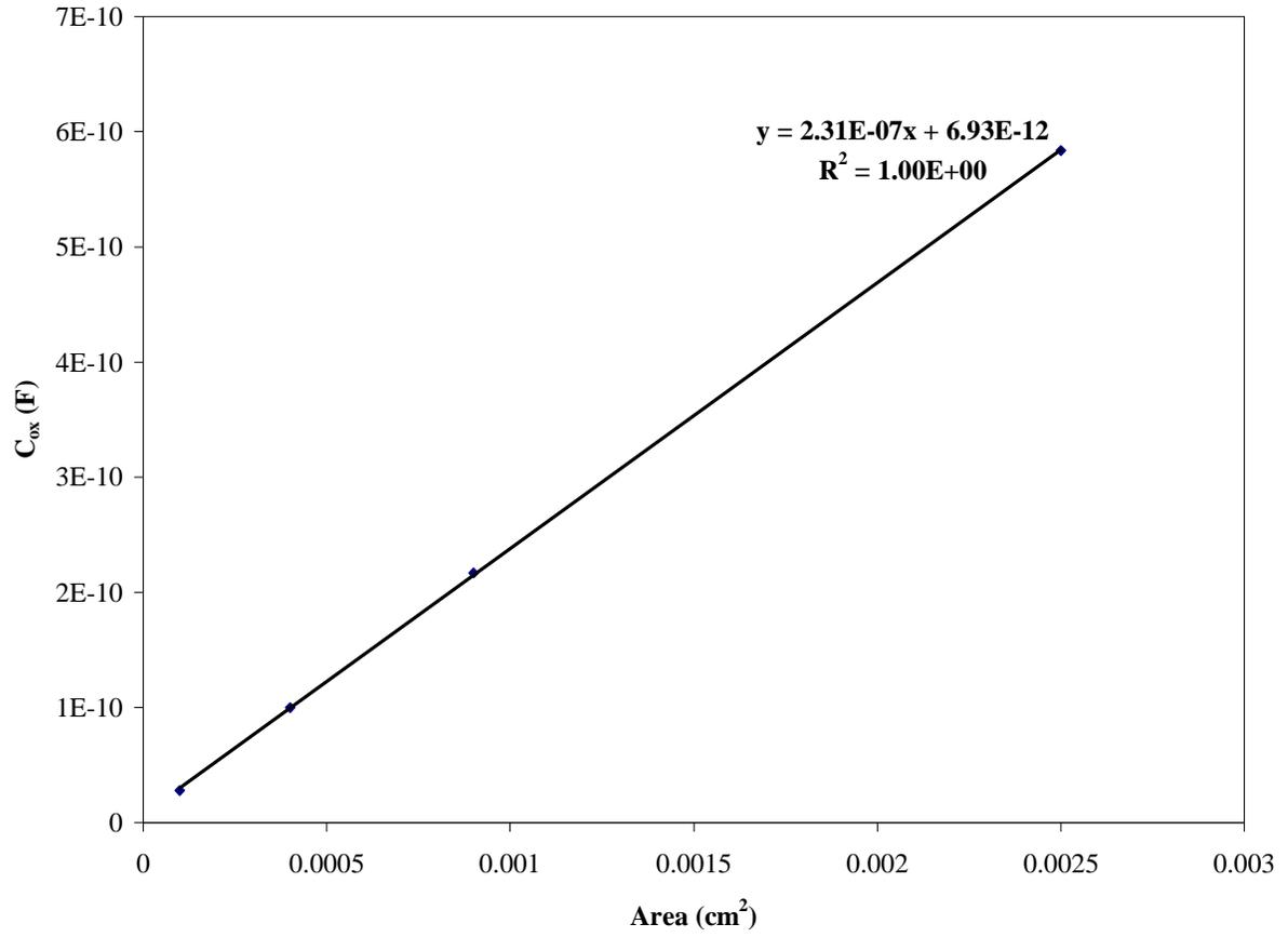
C<sub>ox</sub> vs. Capacitor Area Plot for Wafer A2 (800°C/45 min./N<sub>2</sub>O<sub>2</sub>)
