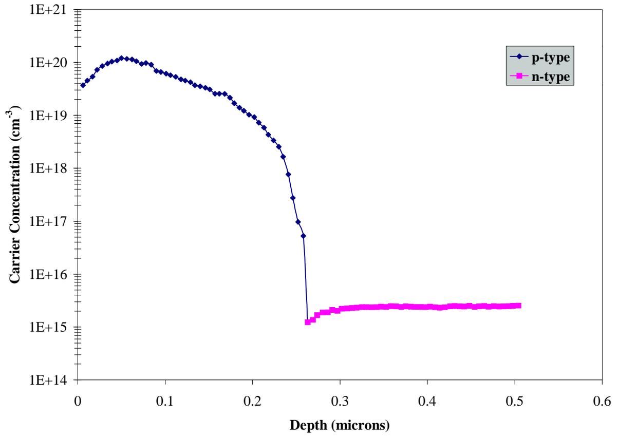
SRA Profile for Wafer B1 (900°C/60 min./N<sub>2</sub>)
