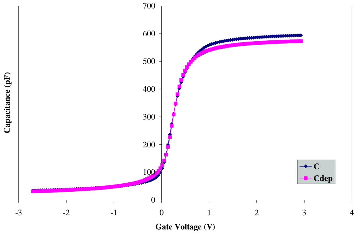
High Frequency CV Curve for Wafer B2 (900°C/60 min./N<sub>2</sub>O<sub>2</sub>)
