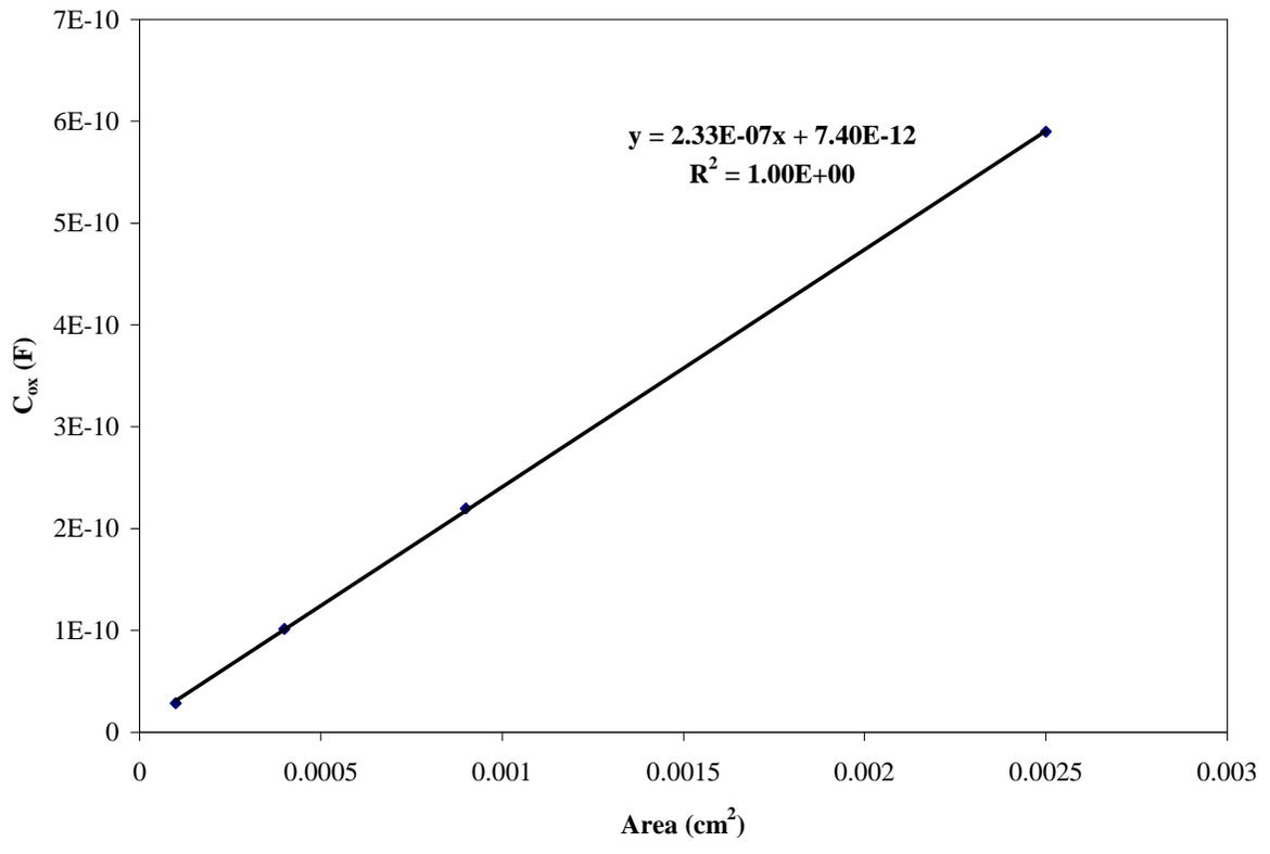
C<sub>ox</sub> vs. Capacitor Area Plot for Wafer A4 (800°C/20 min./N<sub>2</sub>O<sub>2</sub>)
