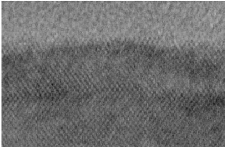
Cross-Sectional TEM Image for Sample C2 (1000°C/45 min./N<sub>2</sub>O<sub>2</sub>)
