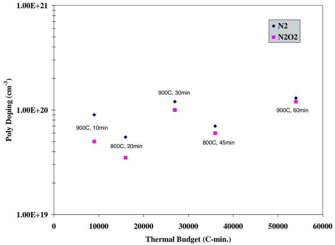
Figure 4.9 – Plot of poly doping level vs. thermal budget
