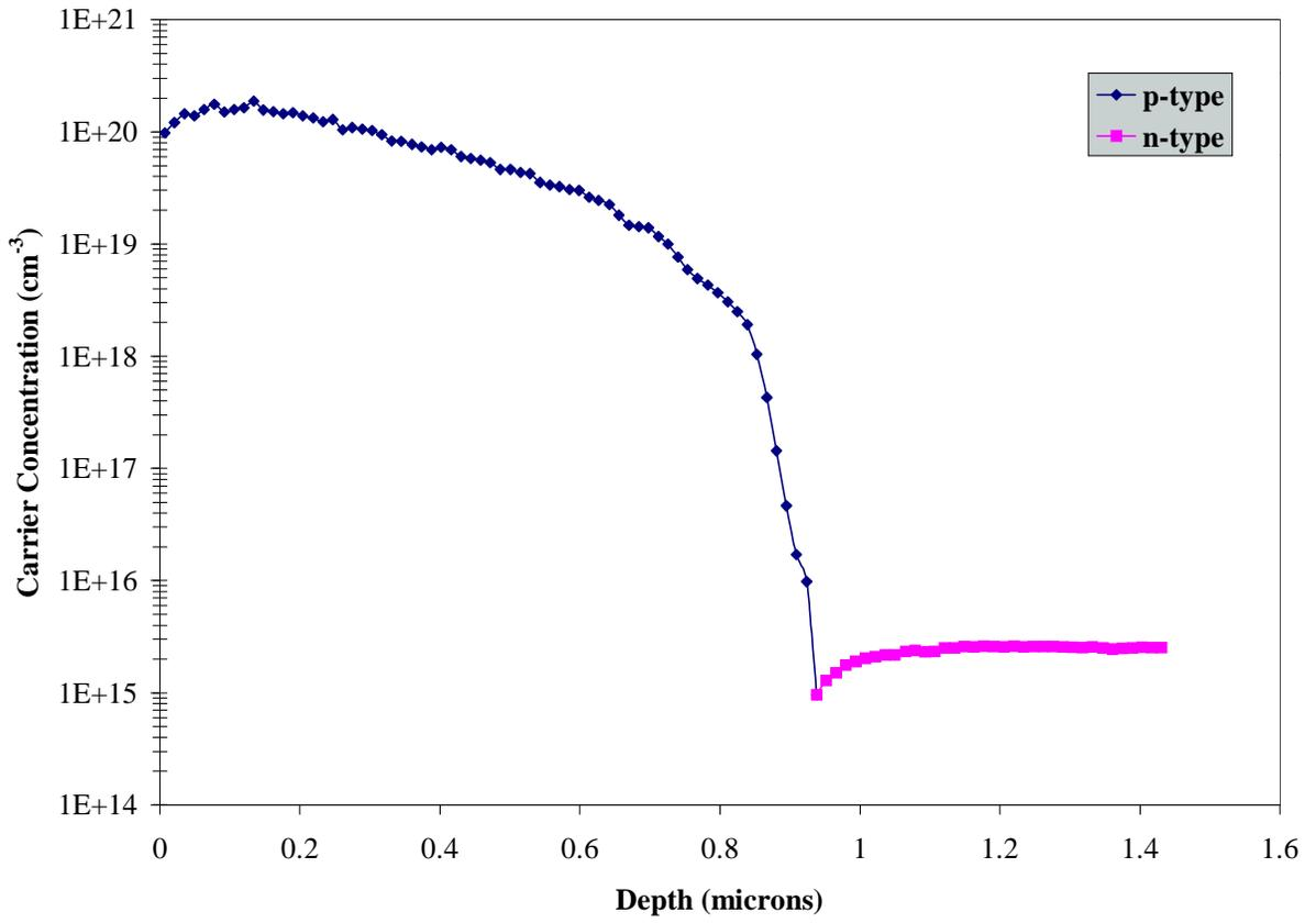
SRA Profile for Wafer C2 (1000°C/45 min./N<sub>2</sub>O<sub>2</sub>)
