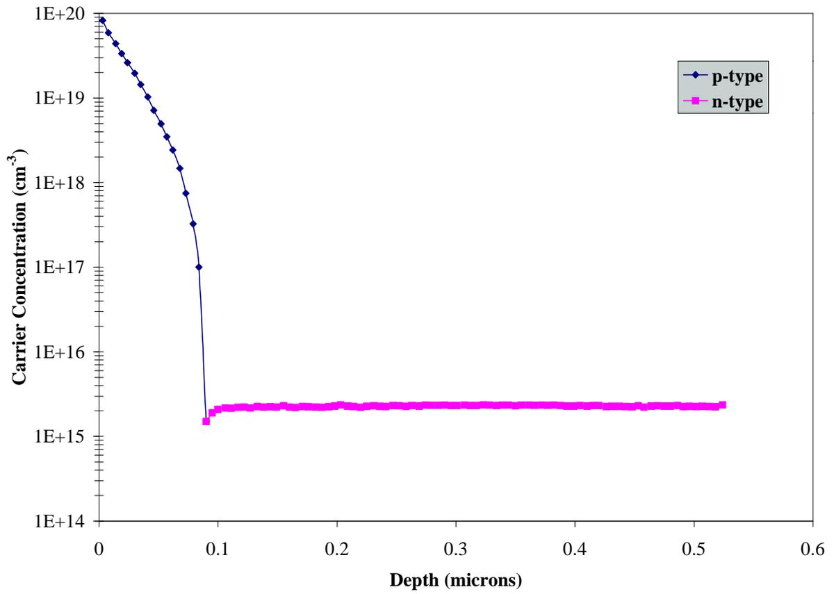
SRA Profile for Wafer A1 (800°C/45 min./N<sub>2</sub>)
