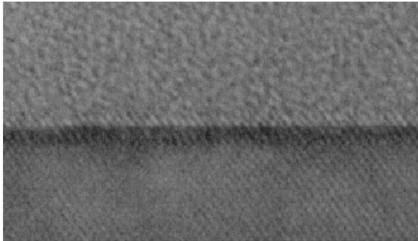
Cross-Sectional TEM Image for Sample A2 (800°C/45 min./N<sub>2</sub>O<sub>2</sub>)
