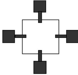
Figure 3.2 – Schematic of the van der Pauw structure tested for sheet resistance data
