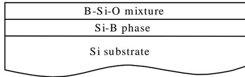
Figure 2.2 – Schematic of structure formed on Si wafer during boron diffusion
