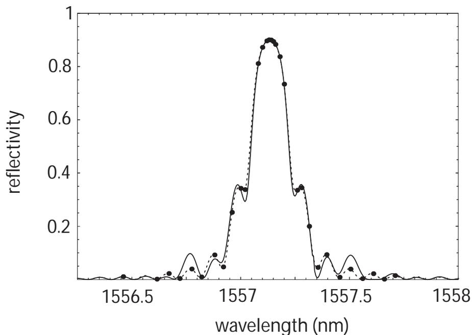
Figure 4.2: Reflected spectrum of Bragg grating subjected to the linear strain field  $\epsilon_z = \{10^{-10}/m\} z$ , obtained through T-matrix calculation of grating response (dashed line). Also plotted is the reflected spectrum of optimal solution from GA (solid line). Properties of grating are defined in table 4.1. Points used to calculate fitness function are highlighted.
