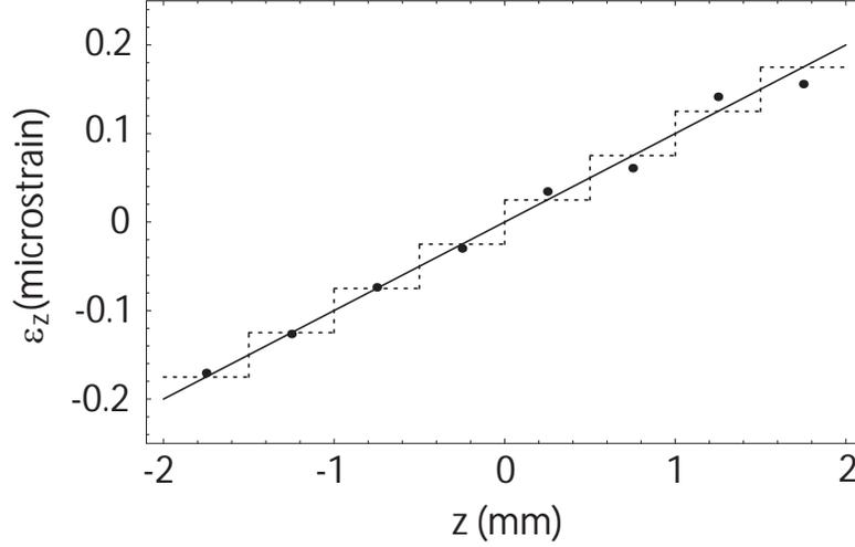
Figure 4.5: Axial strain distribution obtained from modified GA,  $\epsilon_z$ : solid line plots applied linear strain distribution; dashed line piecewise constant approximation used as input for measured spectrum calculation; points represent strain in each segment obtained from GA optimal solution.
