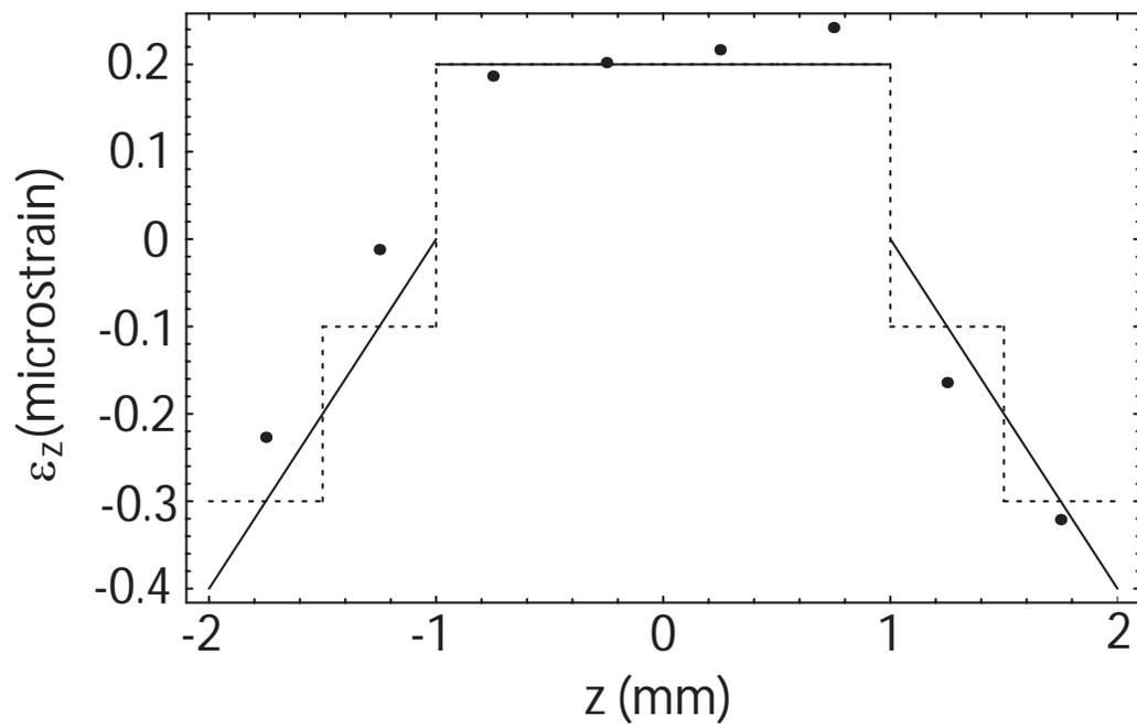
Figure 4.10: Applied strain distribution,  $\epsilon_z$ : (solid line) applied linear strain distribution; (dashed line) piecewise constant approximation used as input for measured spectrum calculations; (points) strain in each segment obtained from GA optimal solution.
