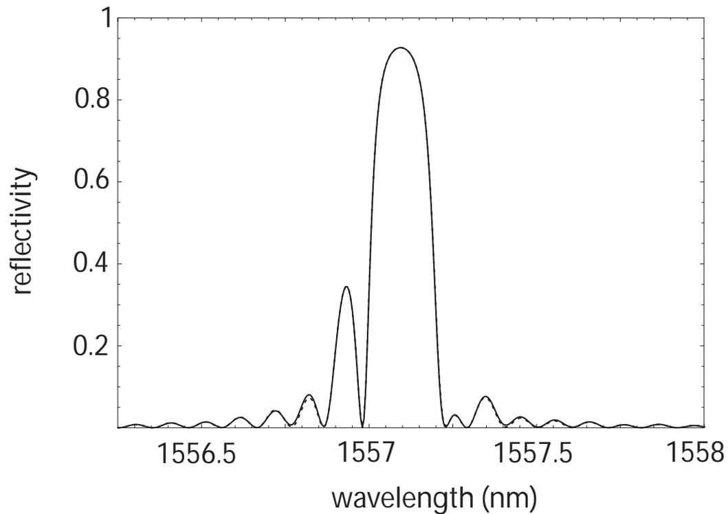
Figure 4.7: Reflected spectrum of Bragg grating subjected to the discontinuous strain field of figure 4.6, obtained through T-matrix calculation of grating response (dashed line). Also plotted is the reflected spectrum of optimal solution from GA (solid line). Properties of grating are defined in table 4.1.
