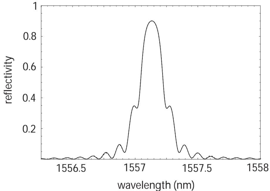
Figure 4.4: Reflected spectrum of optimal solution from GA with modified parameters of table 4.3 (solid line). Also plotted is input reflected spectrum of Bragg grating subjected to linear strain field (dashed line).
