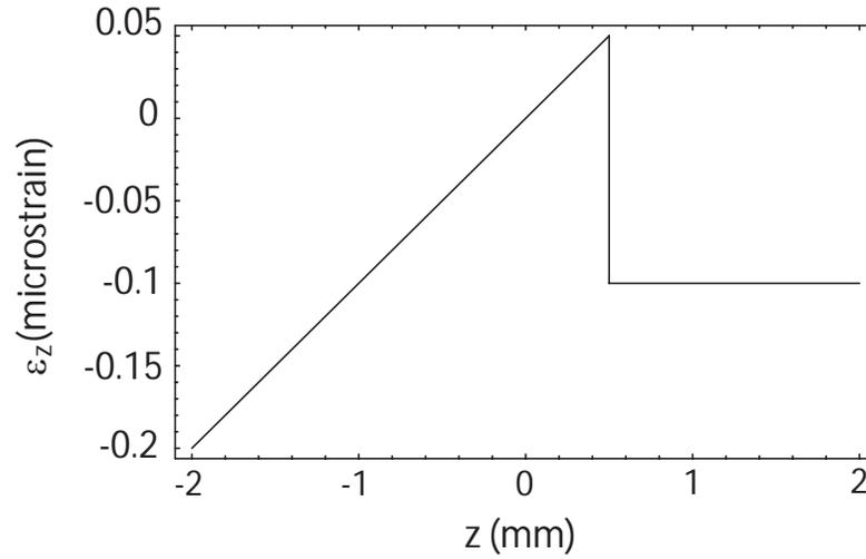
Figure 4.6: Discontinuous strain distribution,  $\epsilon_z$ , applied to Bragg grating.
