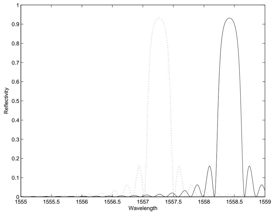
Figure 3.2: Wavelength shift in reflected spectrum of fiber Bragg grating. Reflected spectrum of unloaded grating (zero strain) is plotted by dashed line. Solid line plot gives reflected spectrum of grating as result of applied constant strain.
