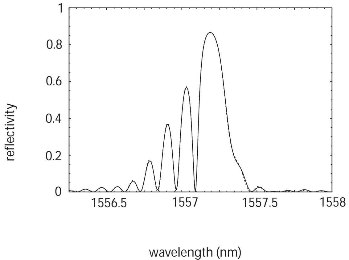
Figure 4.9: Reflected spectrum of Bragg grating subjected to discontinuous strain field of figure 4.10, obtained through numerical solution of Bragg grating coupled mode equations (dashed line). Also plotted is the reflected spectrum of optimal solution from GA (solid line).
