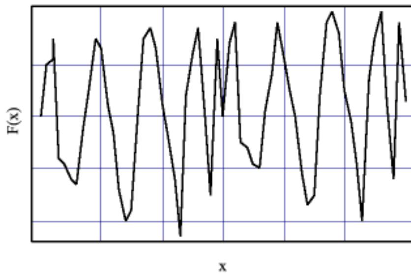
Figure 2.3: Function not suitable for derivative based optimization methods.
