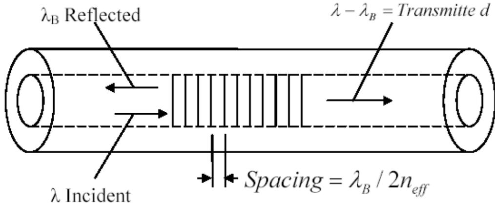
Figure 3.1: Bragg rasonance for the reflection of incident mode occurs at the wavelength for which grating period along the fiber axis is equal to one-half of the modal wavelength within the fiber core. The back scattering from each crest in the periodic perturbation will be in phase and the scattering intensity will accumulate as the incident wave is coupled to a backward propagating wave [7].
