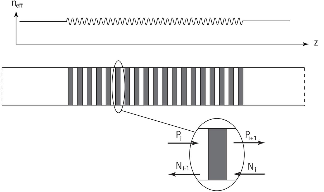
Figure 4.1: Parameters for T-matrix formulation of Bragg grating spectral response. Also shown is effective mode index of refraction of optical fiber.
