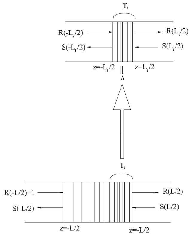
Figure 3.3: Bragg grating Transfer matrix model.
