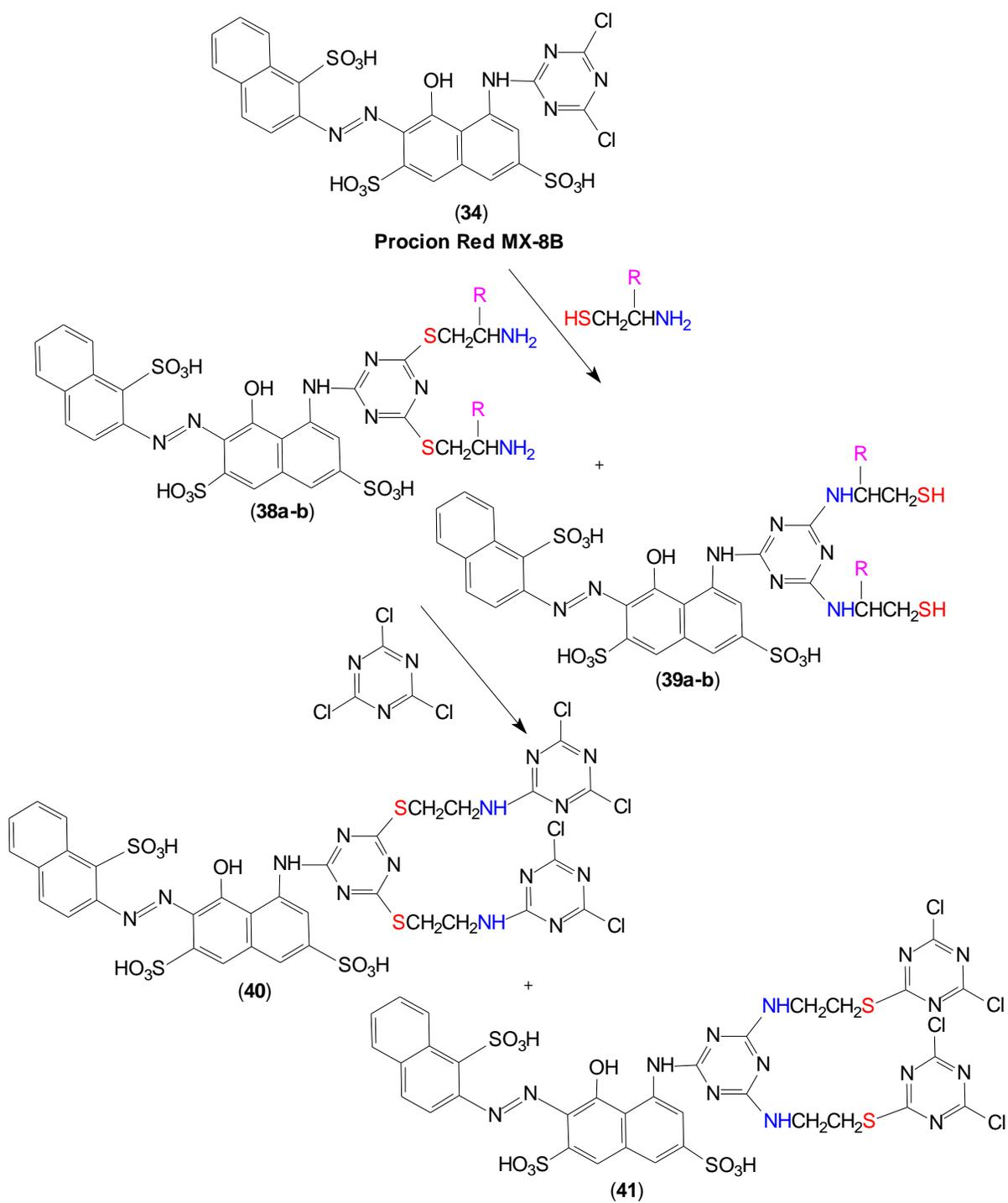
**Figure 1.10.** Potential Teegafix red dye structures from varying the pH of synthesis (R = H, CO<sub>2</sub>H).
