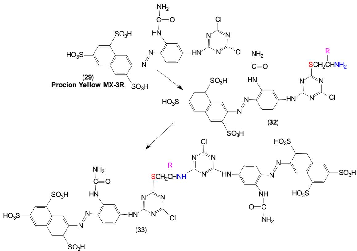
**Figure 1.8.** Synthesis of types 3 (R = CO<sub>2</sub>H) and 4 (R = H) Teegafix yellow dyes.
