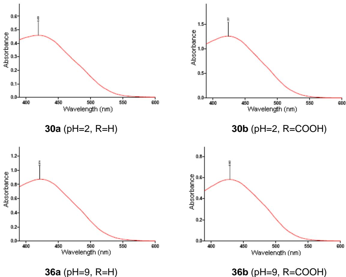
**Figure 3.1.** Visible absorption spectra for yellow dye intermediates (**30a-b**, **36a-b**) synthesized at pH 2 and pH 9.
