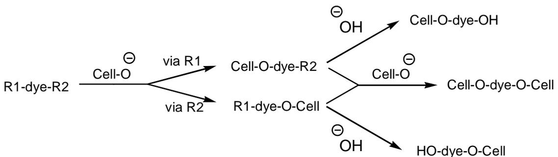
**Figure 1.6.** Fixation of a bifunctional reactive dye to cellulose in the presence of alkali.
