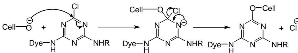
**Figure 1.5.** Mechanism of reaction of a monochlorotriazine dye with the cellulosate ion.
