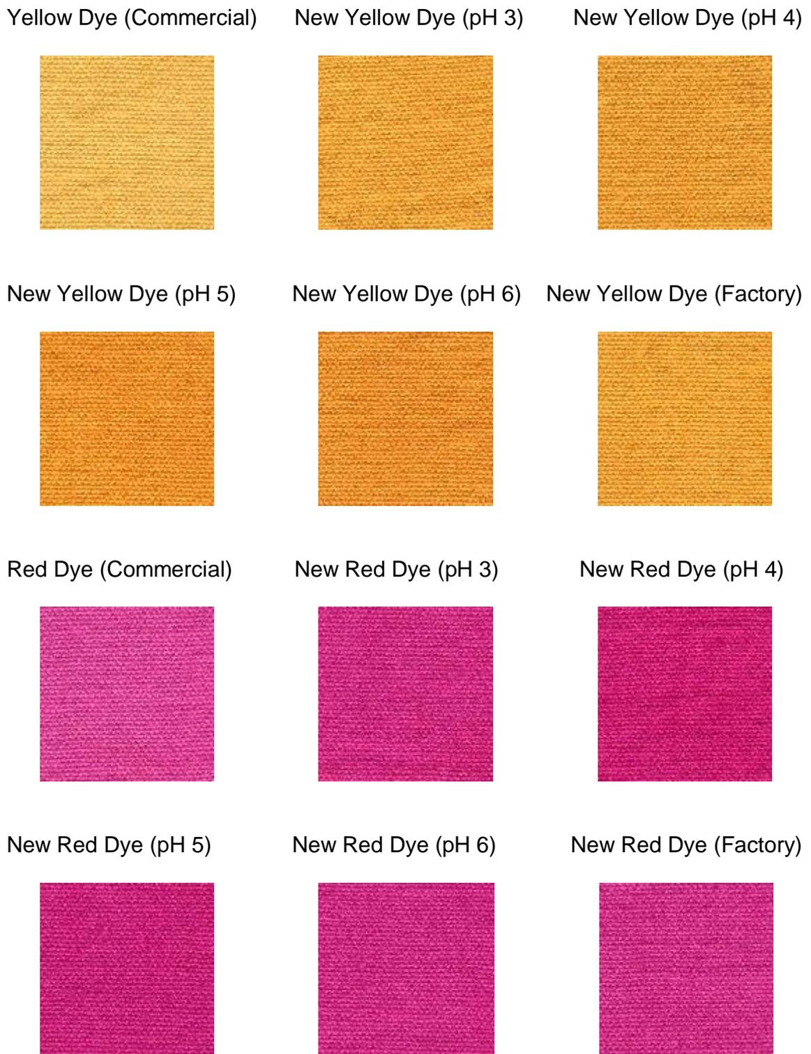
**Figure 3.60.** Fabrics dyed with commercial and new dyes.
