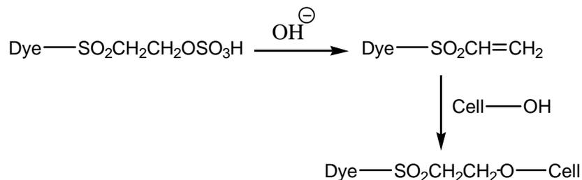
**Figure 1.4.** Reaction of Remazol dyes with cellulose.
