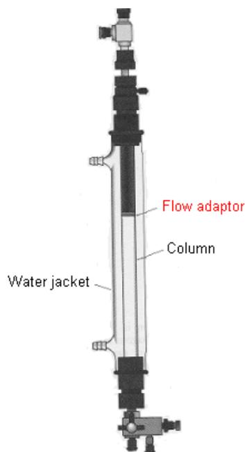
**Figure 1.2.** Glass chromatography column with a flow adaptor at the top.
