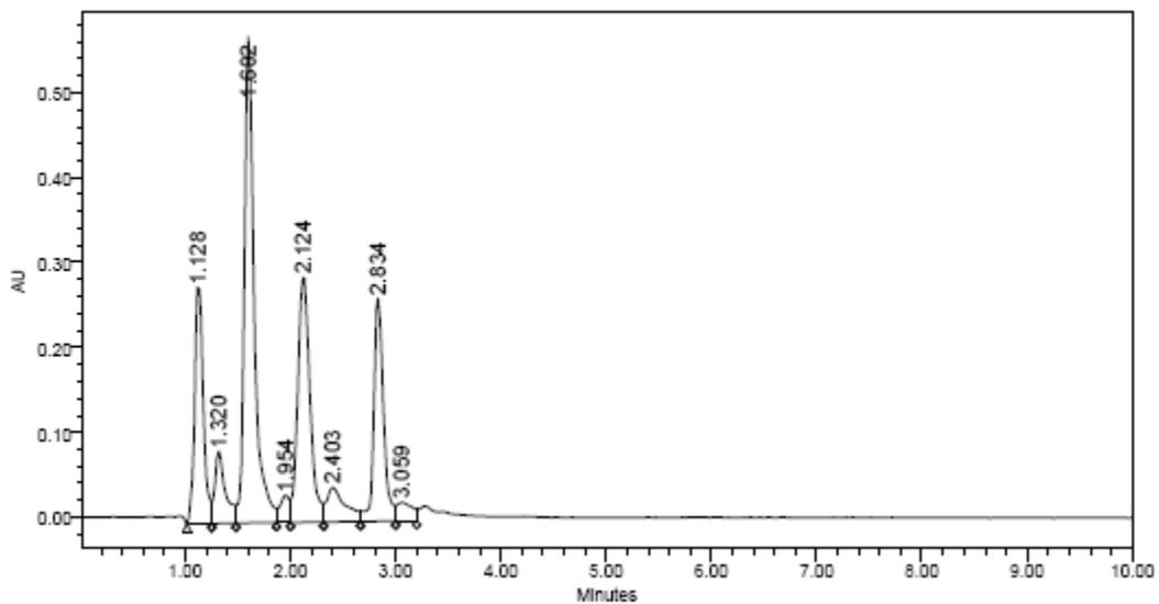
**Figure 3.45.** Chromatogram of **38a/39a** (pH 5) using gradient system 1.
