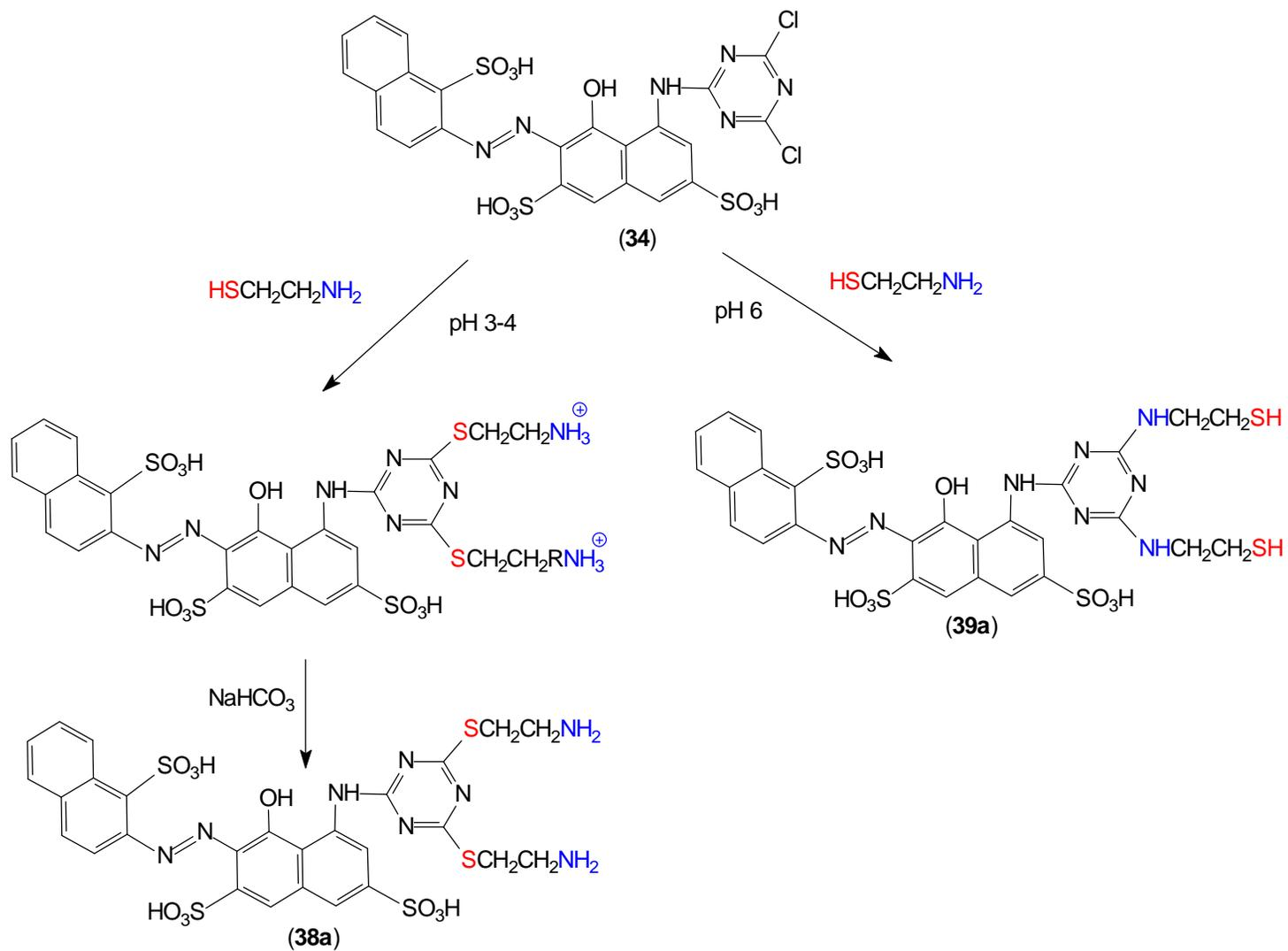
**Figure 3.34.** Synthesis of red dye intermediates from cysteamine at different pH levels.
