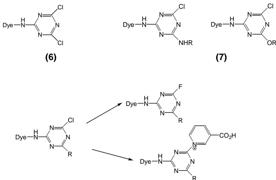
**Figure 1.3.** Conversion of an MCT reactive dye to fluoro and ammonium counterparts.
