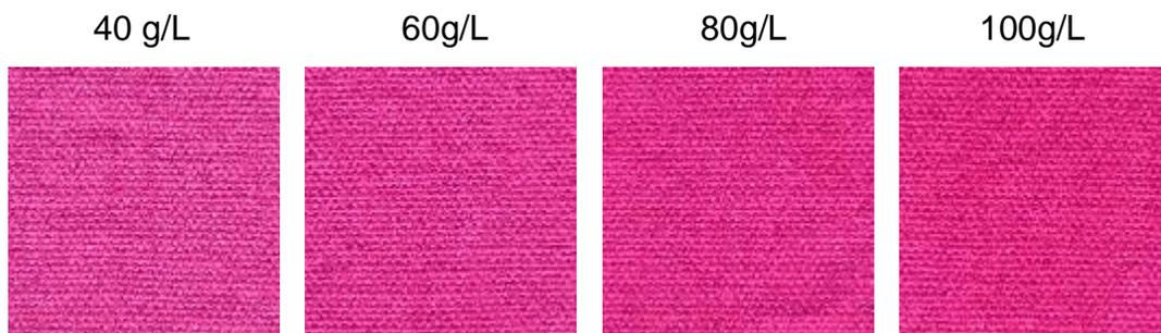
**Figure 3.59.** Fabrics dyed with commercial red dye at different salt levels.
