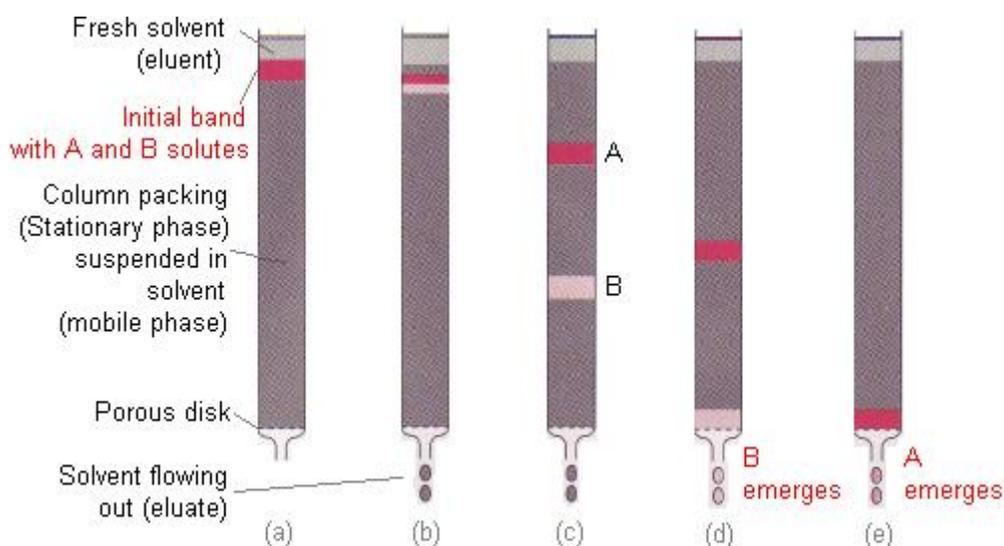
**Figure 1.1.** Schematic representation of column chromatography.
