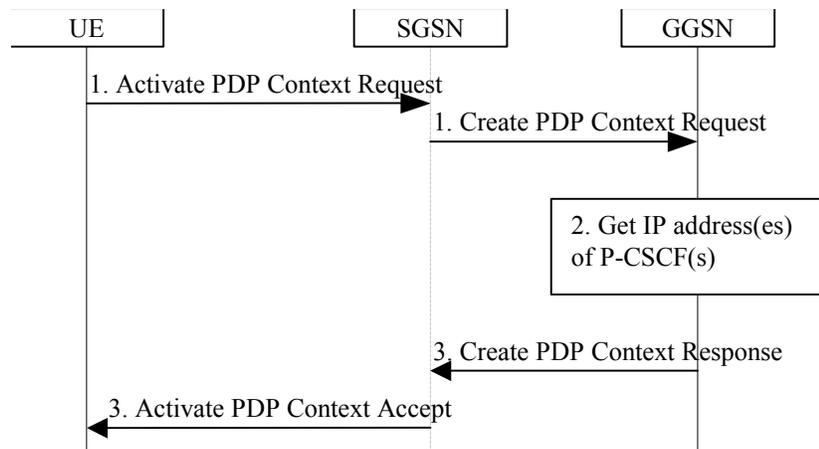
Figure 4: P-CSCF Discovery Using PDP Context Activation Signaling [18]
