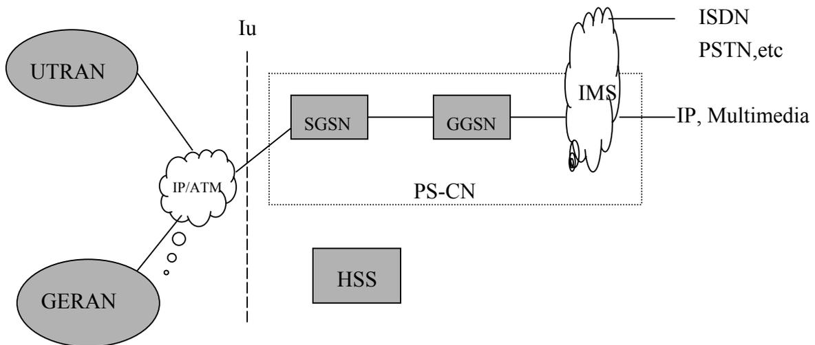
Fig 5. Vision of 3GPP Release 5 (All IP)
