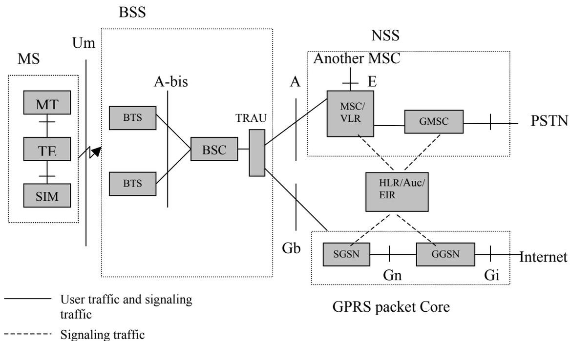
Fig 1: Simplified GSM/GPRS Architecture
