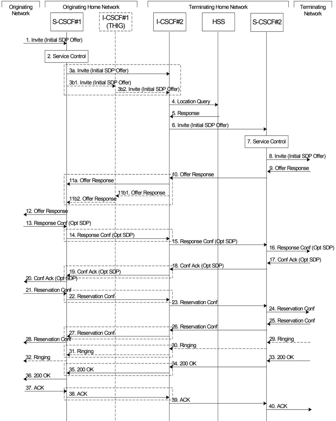
Fig 8. S-CSCF to S-CSCF Procedure – Different Operators [18]
