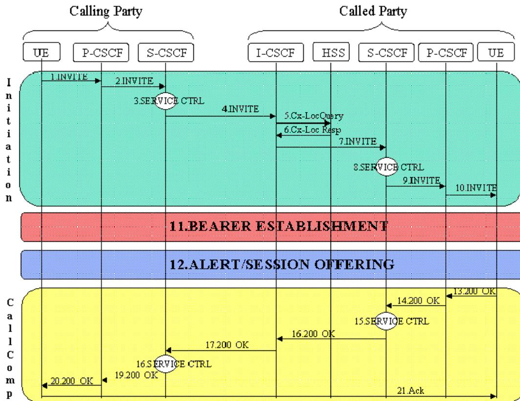
Figure 10: Simplified Mobile-to-Mobile Call flow
