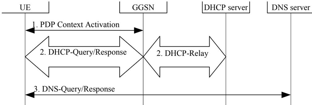
Figure 3: P-CSCF Discovery Using DHCP and DNS [18]
