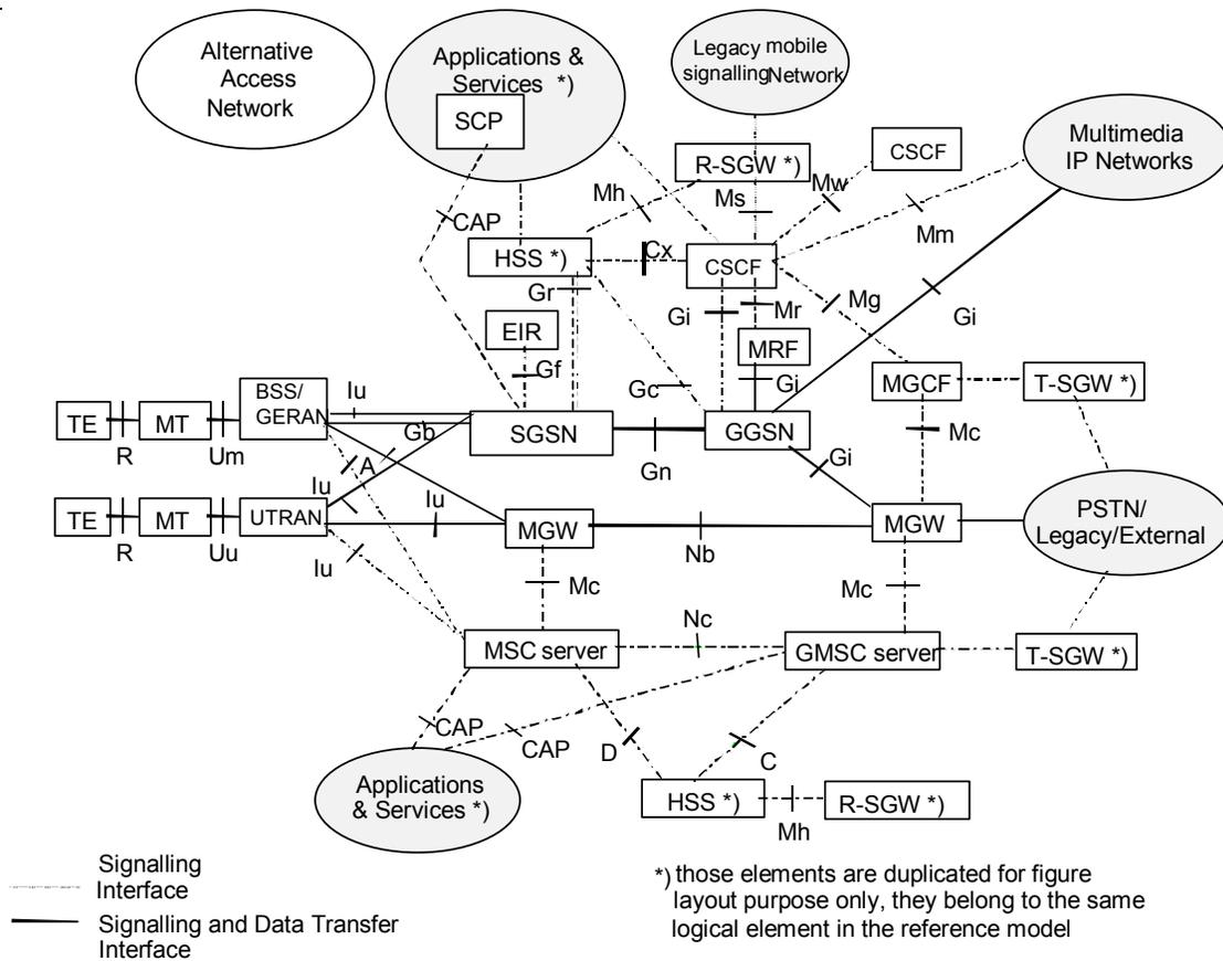
Fig 6. 3GPP R4/5 Reference Logical Architecture [21]
