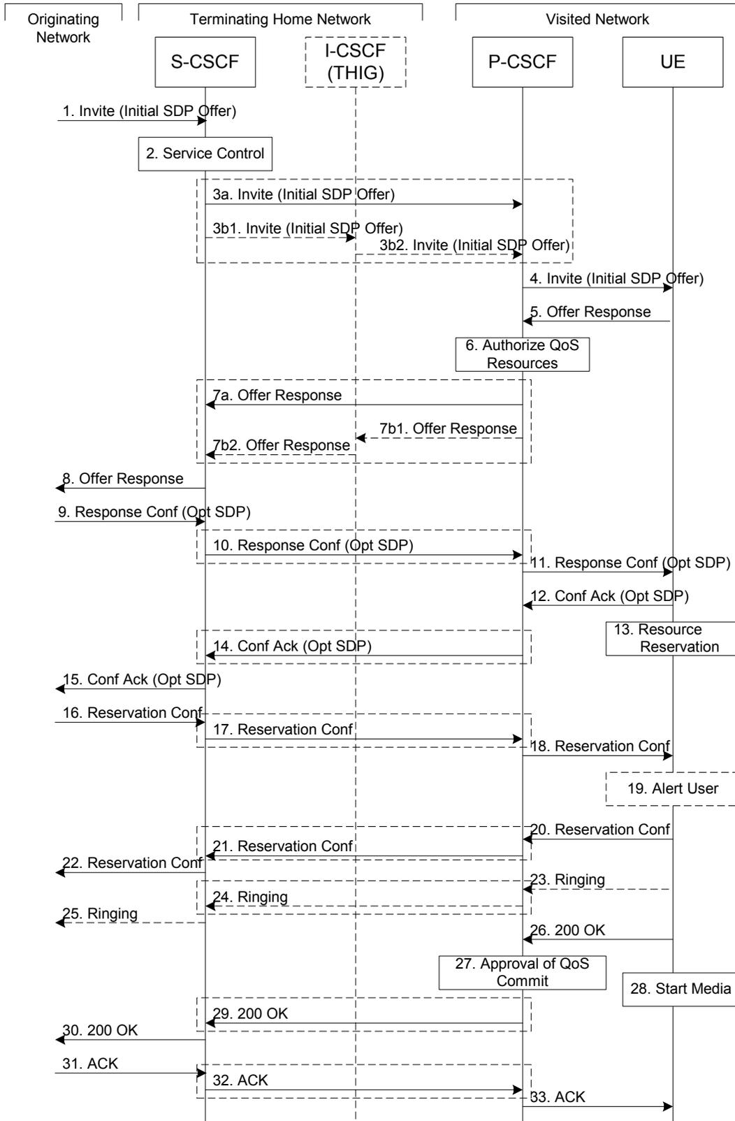
Figure 9: Mobile termination procedure – roaming [18]
