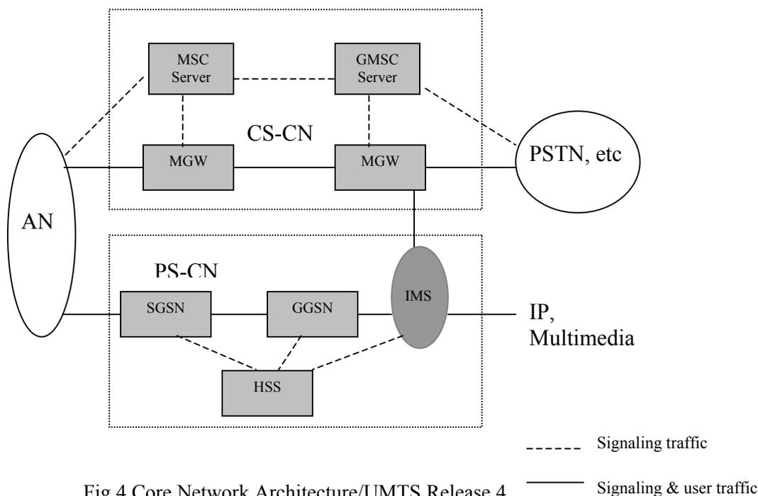
Fig 4. Core Network Architecture/UMTS Release 4
