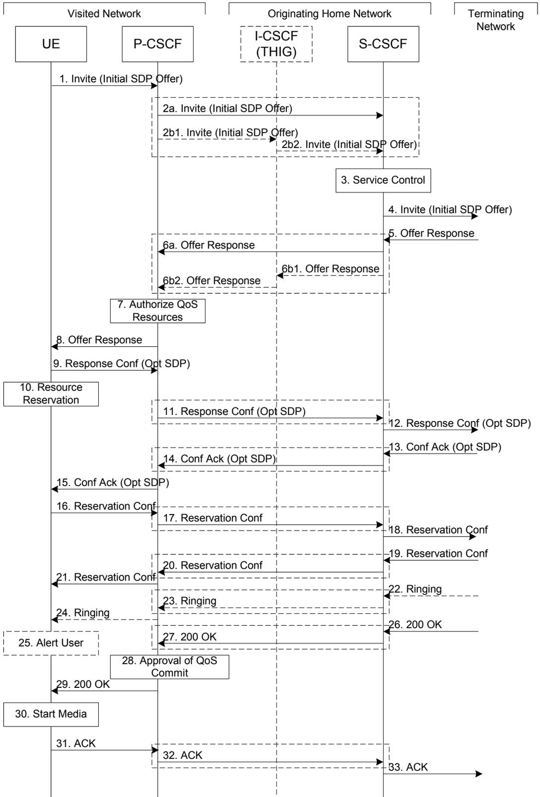
Figure 7: Mobile origination procedure - Roaming [18]
