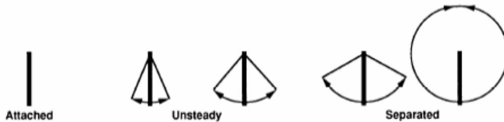
Figure 24: Flow Condition Criteria for Tufts 19
