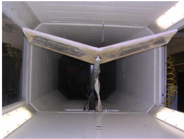
Figure 16: Pressure Port Test in NCSU Wind Tunnel
