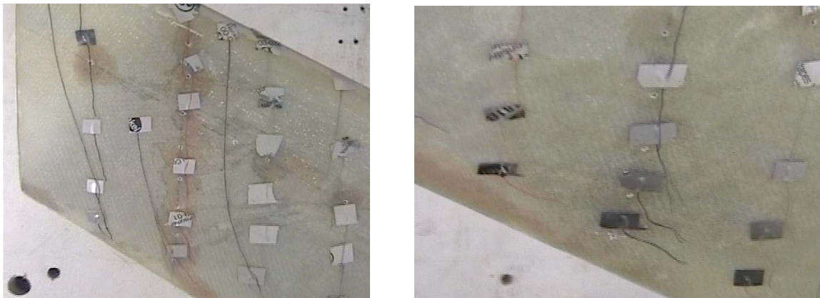
Figure 26: Flow Visualization on the Upper Surface at an Alpha of 10 Degrees
