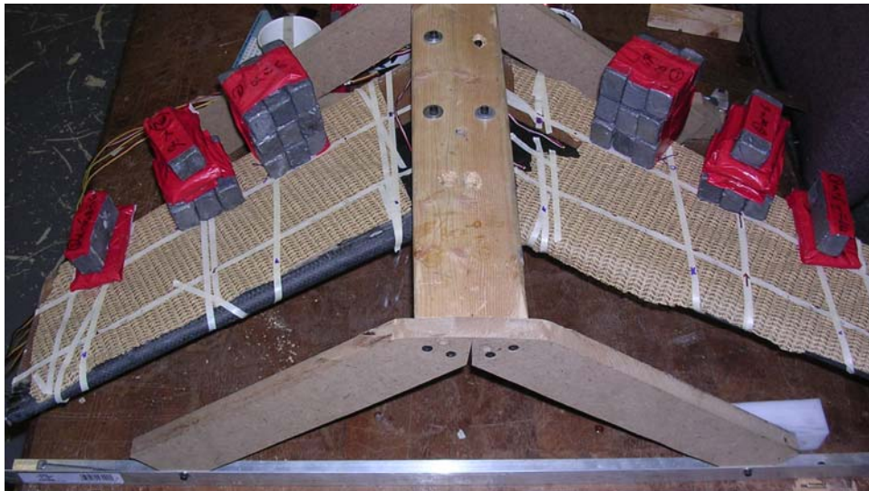
Figure 40: Load Test at a Simulated Alpha of 6 Degrees and q of 30 psf.
