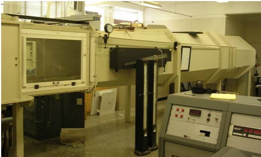
Figure 2: NC State Closed-Circuit Wind Tunnel
