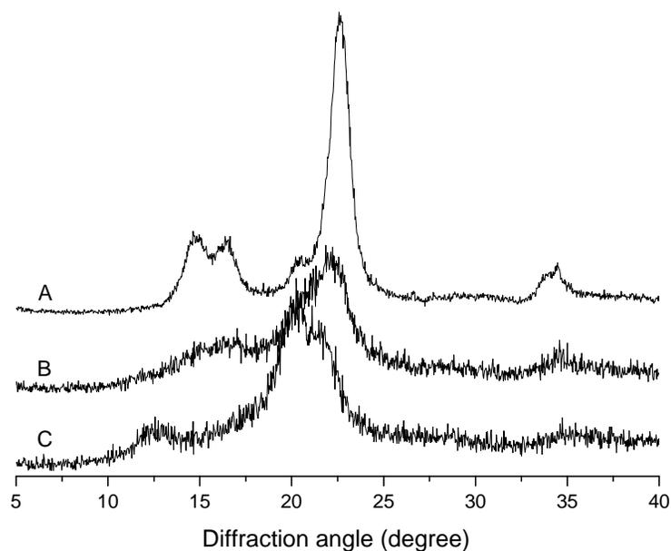
**Figure 3.7 X-ray Diffractograms for CC41 Cellulose: (A) Pure CC41 Cellulose, (B) CC41 Cellulose Recovered from Cellulose Swollen in ED, (C) CC41 Cellulose Recovered from a 5 wt% of Cellulose Solution with a ED/KSCN Solvent (77/23, w/w) [21]**
