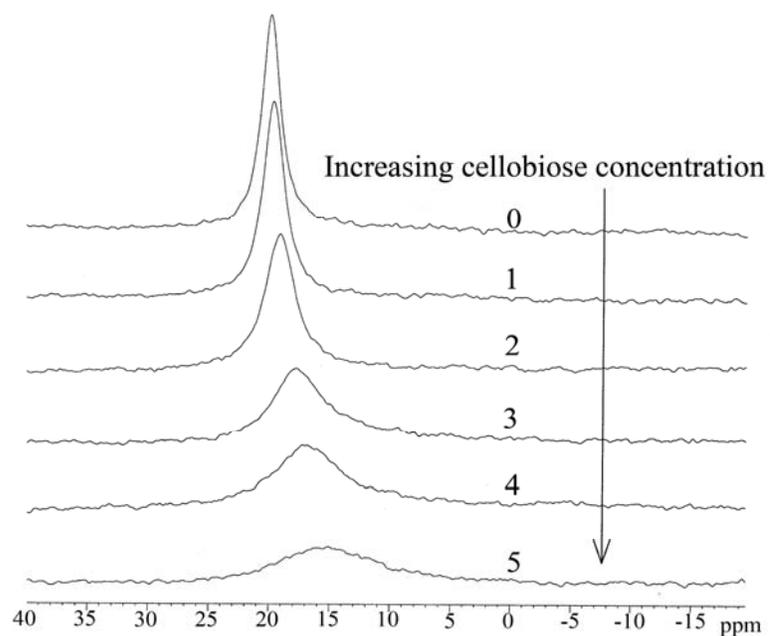
**Figure 3.4  $^{39}\text{K}$  NMR Spectra of Cellobiose (DP 2) Solution in ED/KSCN (92.3/7.7, w/w) Solvent [21]**
