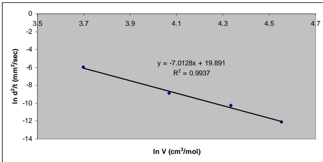
**Figure 6.7 Dependence of coagulation rate at 120 min on the molecular volume of the coagulants for cellulose/ED/KSCN (7/65/35)**
