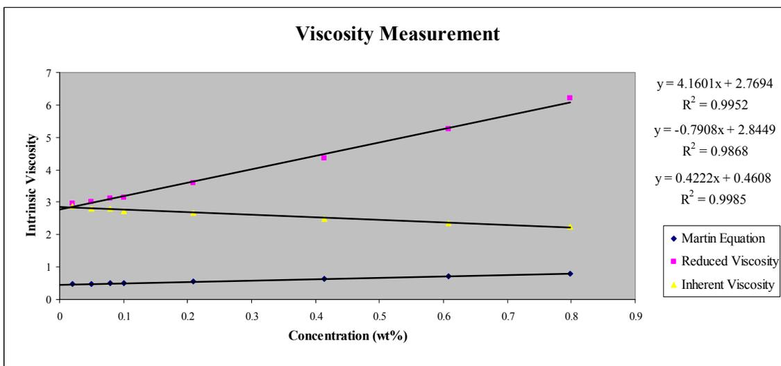
**Figure 6.2 Viscosity Measurement of VFC Cellulose**
