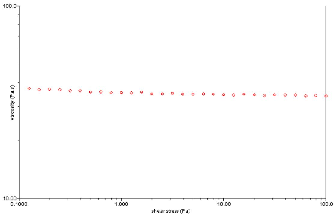
**Figure 6.8 Viscosity of Cellulose/ED/KSCN (7/65/35) Solution at 60°C**
