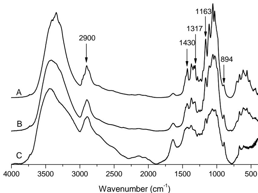
**Figure 3.3 FTIR Spectra of Cellulose; (a) Pure CC41 Cellulose (DP 210), (b) CC41 Cellulose recovered from cellulose swollen in ED, (c) CC41 Cellulose recovered from cellulose/ED/KSCN (5/77/23) solution [21]**
