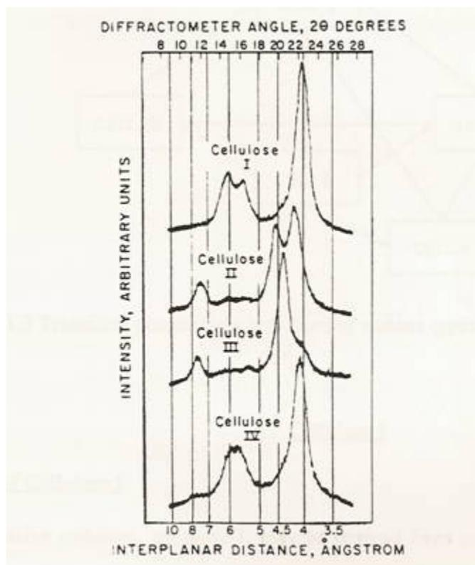
**Figure 2.1 X-ray diffractograms of four cellulose polymorphs [5]**
