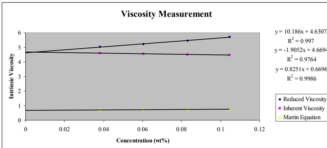
**Figure 6.1 Viscosity Measurement of AV Cellulose**
