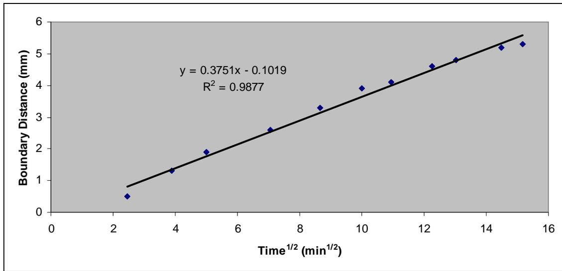
**Figure 6.6 Boundary Movement in the Coagulation Process of Cellulose/ED/KSCN (7/65/35) Solution**
