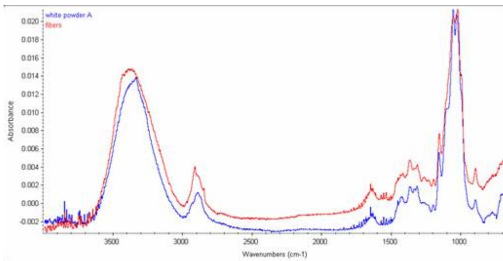
**Figure 6.11 FTIR Spectra of VFC Cellulose Pulp and Cellulose fibers spun by ED/KSCN Solvent System.**
