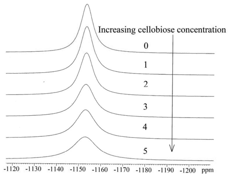
**Figure 3.6  $^{19}\text{N}$  from EDA NMR Spectra of Cellobiose Solution in ED/KSCN (92.3/7.7 w/w) Solvent [21]**
