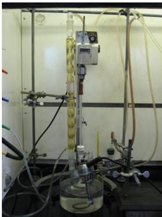
**Figure 5.1 Experimental Set-up for Cellulose Dissolution Process**
