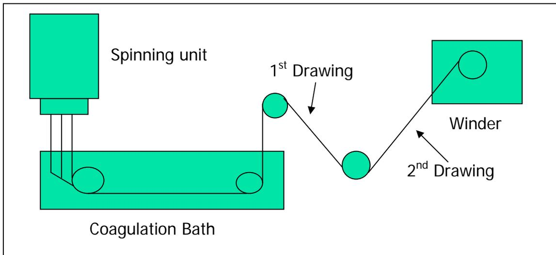
**Figure 5.3 Schematic of the Dry Jet-Wet Spinning System of Cellulose Fibers**
