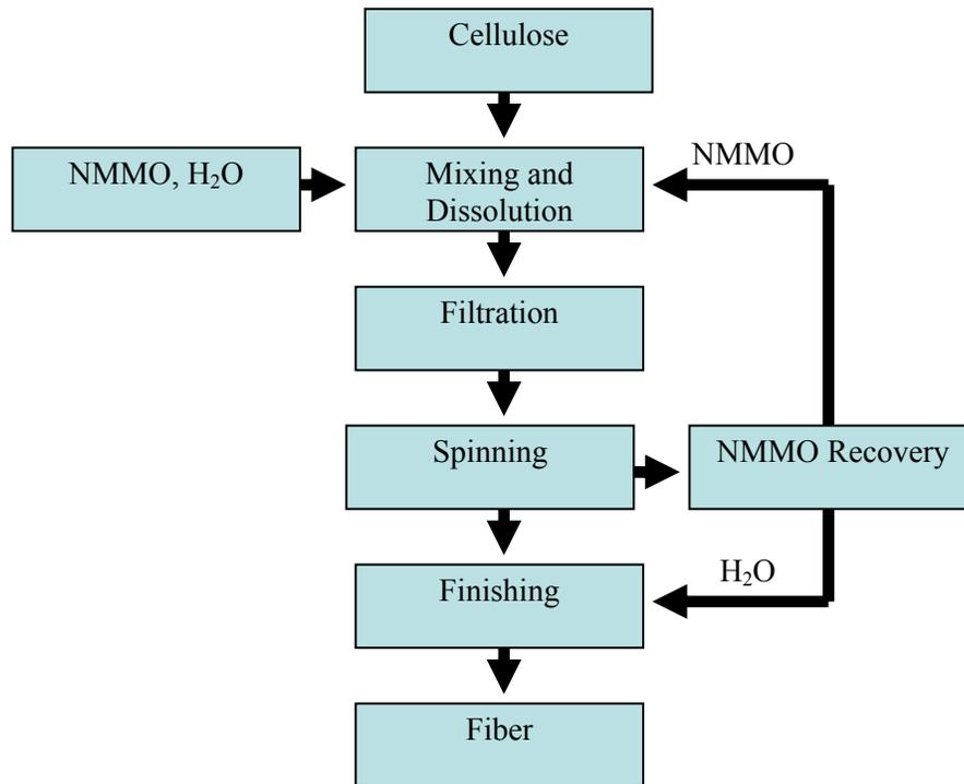
**Figure 4.1 Schematic of NMMO Process [6]**
