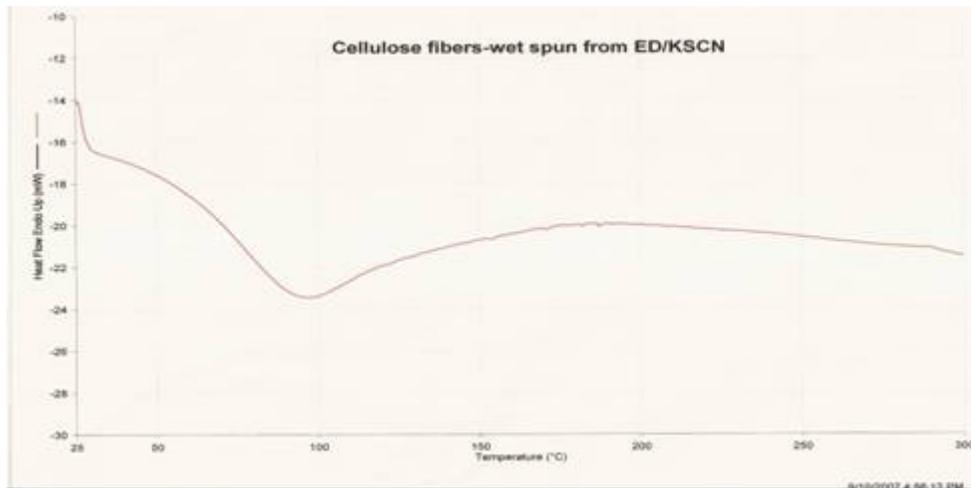
**Figure 6.12 DSC Thermogram of Cellulose/ED/KSCN (7/65/35) Solution and Cellulose Fibers via ED/KSCN Solvent system**
