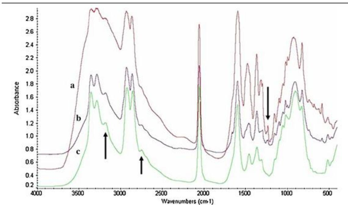
**Figure 3.2 FTIR spectra of; (a) Cellulose/ED/KSCN mixture, (b) Mixture after one temperature cycling, (c) Cellulose/ED/KSCN solution [22]**
