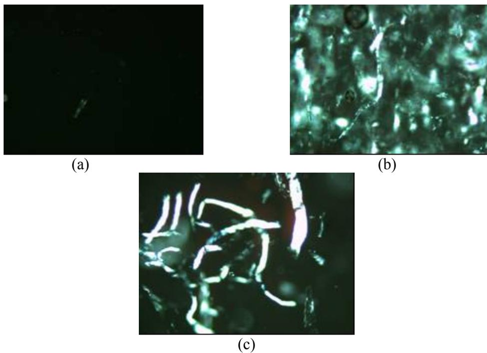
**Figure 6.3 Polarized Light Microscopy Images of 5 wt% VFC Cellulose Dissolved in (a) ED/KSCN (65/35), (b) ED/KSCN (85/15), (c) ED/NaSCN (60/40)**
