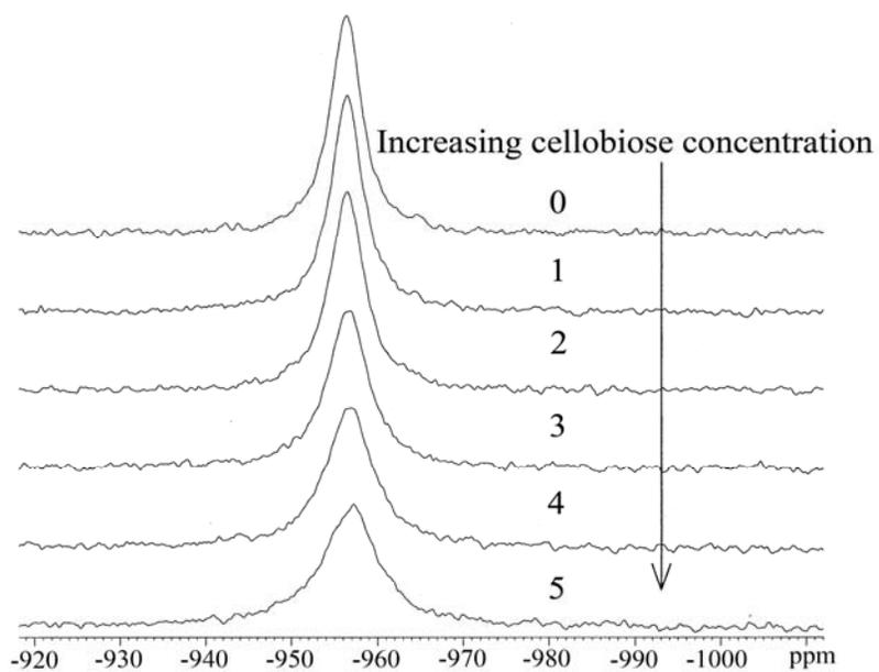
**Figure 3.5  $^{14}\text{N}$  from KSCN NMR Spectra of Cellobiose Solution in ED/KSCN (92.3/7.7) Solvent [21]**
