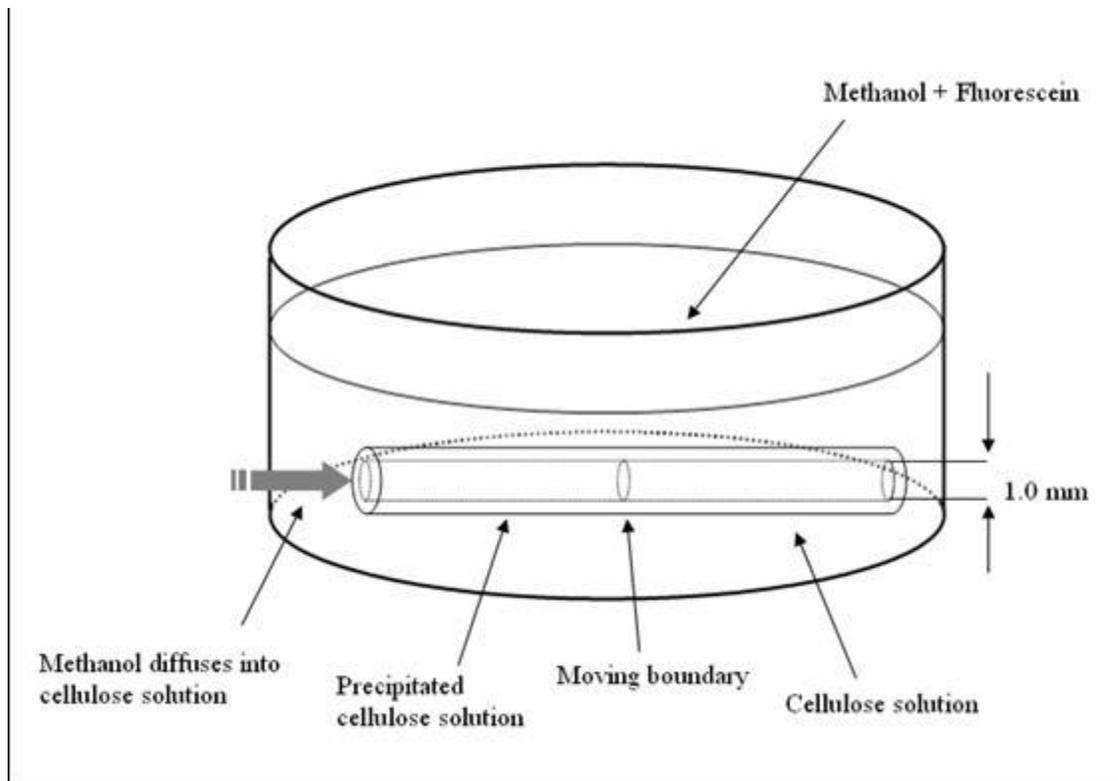
**Figure 5.2 Schematic of Coagulation Rate Experiment Set-up**
