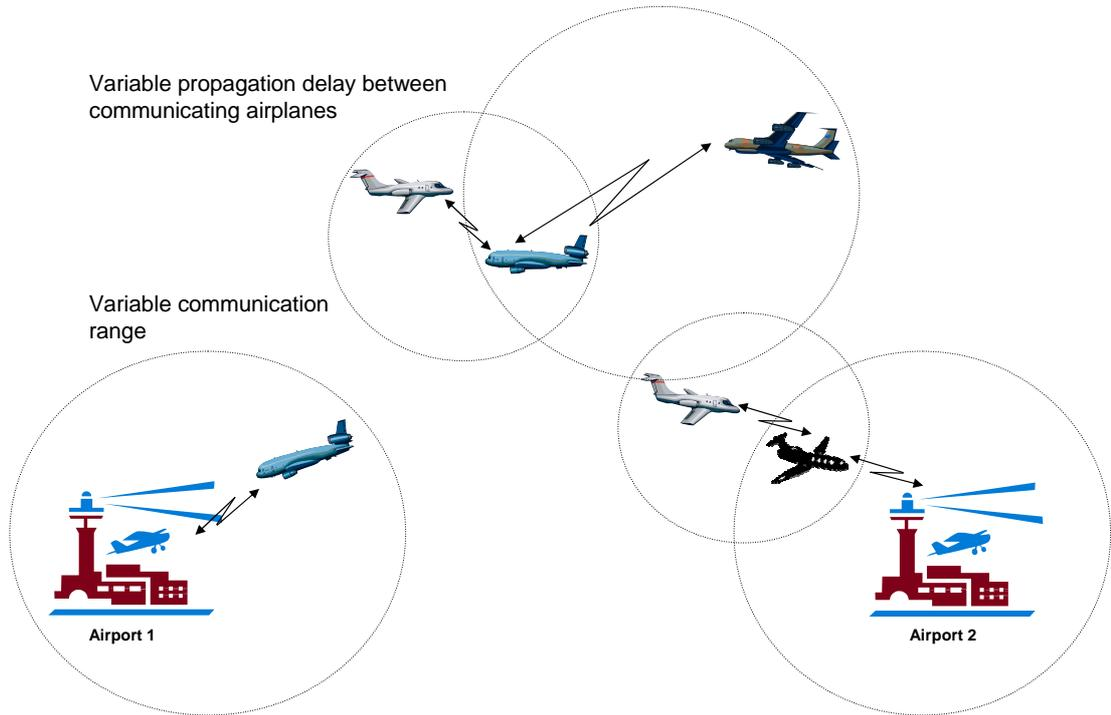
Figure 3.1: A2A communication environment for black box data replication.
