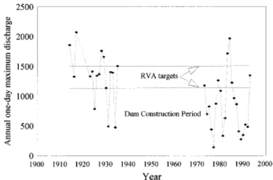
**Figure 1:** RVA Target Establishment and the Frequency of Data Points that Fall within the three Ranges. (Source Richter et. al 1998)
