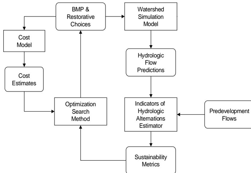
**Figure 3 :** Design Procedure for Simulation-Optimization Method
