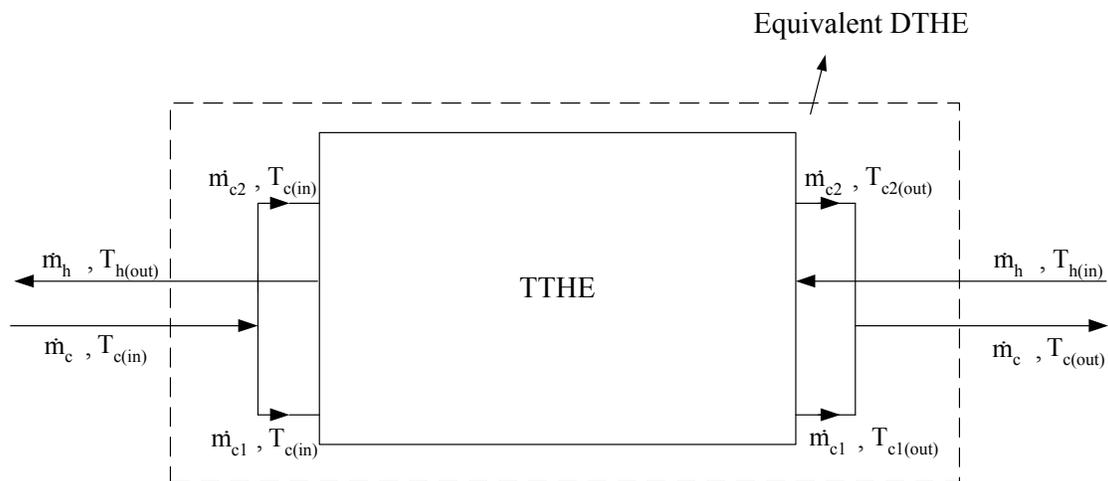
Figure 2. Converting a TTHE into an equivalent DTHE
