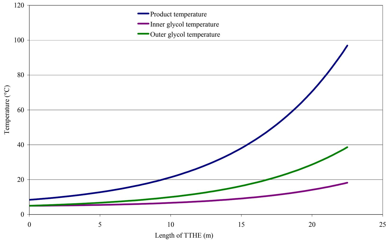
Figure 3. Axial temperature distribution of fluids in counter-current arrangement
