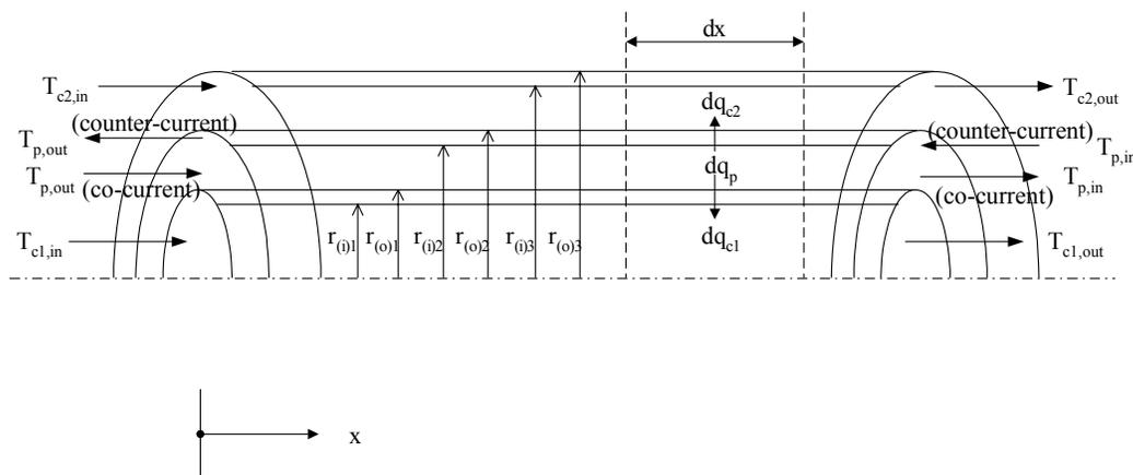
Figure 1. Counter-current and co-current arrangements in a TTHE
