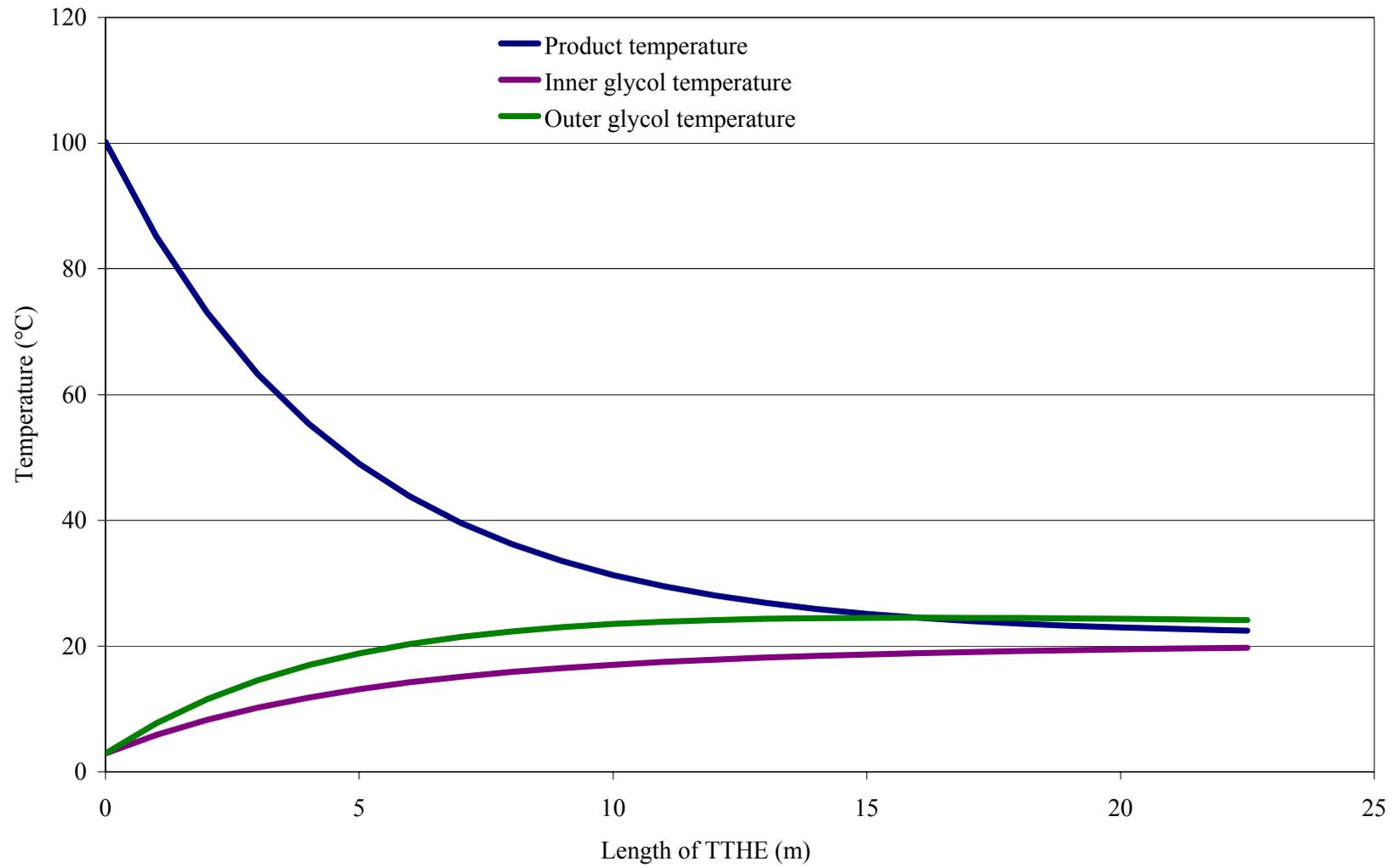
Figure 4. Axial temperature distribution of fluids in co-current arrangement
