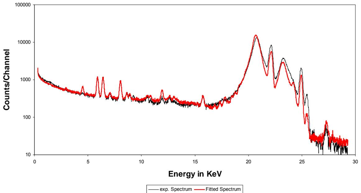
Figure 6.8 Experimental spectrum and fitted spectrum for AA3004
