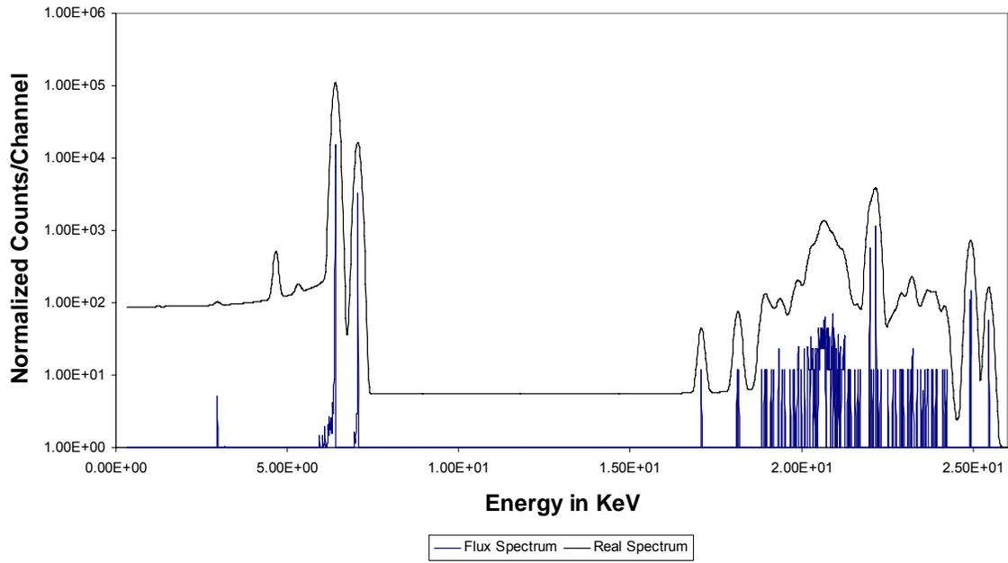
Figure 6.5 Simulated library spectrum of Iron (Fe, 26)
