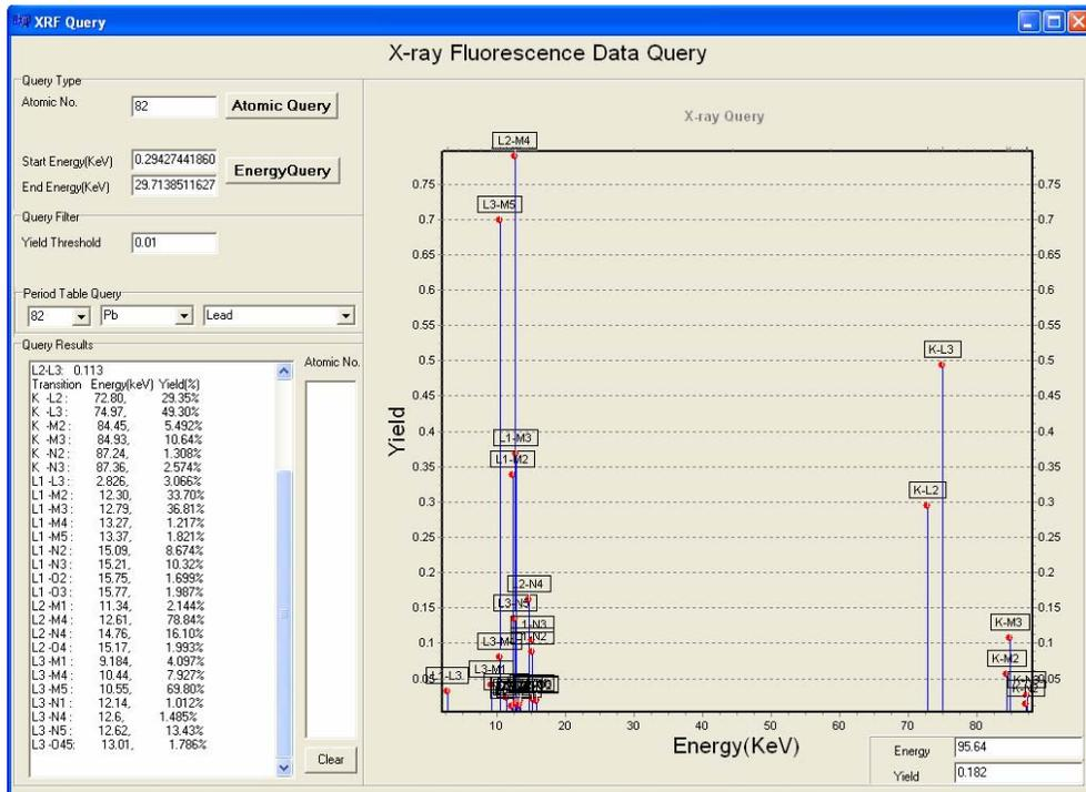
Figure 5.3 XRF Query results for Pb (82)
