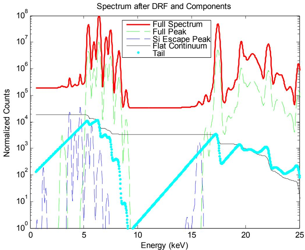
Figure 4.8 Detector Response Function (DRF) and its components
