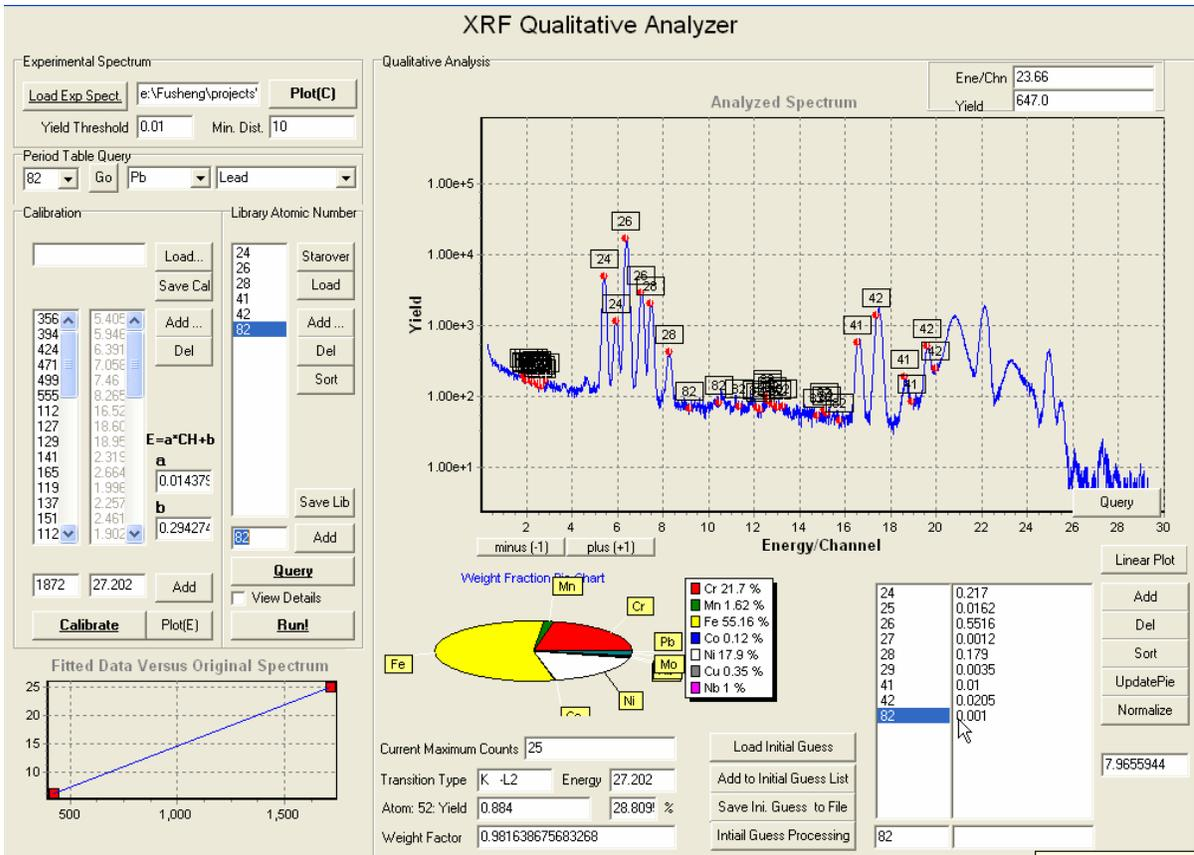
Figure 5.2 Preliminary results for C1152A with <sup>109</sup>Cd source from Qualitative Analyzer
