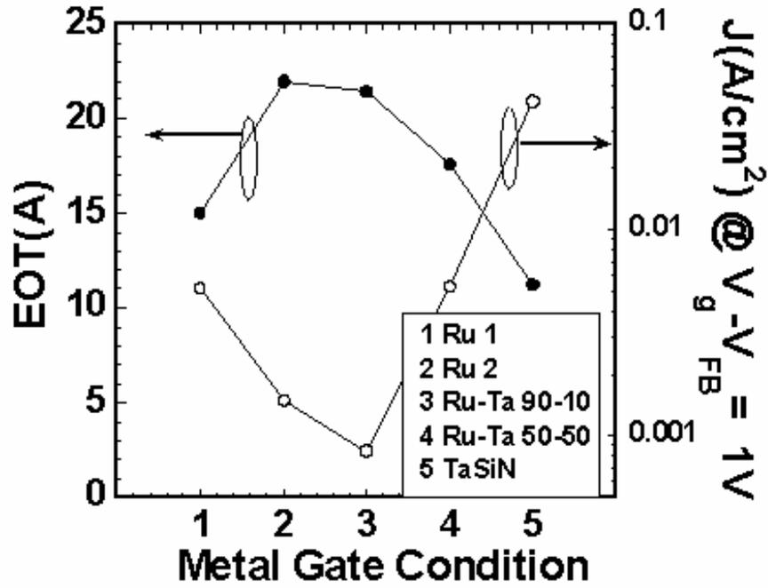
Figure 2. 14 Leakage current plot for various metal gates on HfO<sub>2</sub> gate dielectrics taken at 1V beyond V<sub>FB</sub>.
