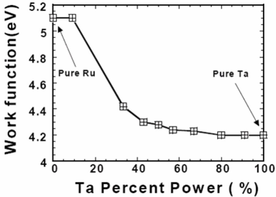
Figure 4. 5 Work function extracted from C-V curves for various compositions of Ru-Ta alloys. Non-linear behavior as a function of content is observed
