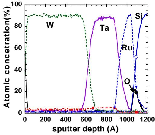
Figure 4. 11 (a) Auger Depth Profile of as deposited Si/SiO<sub>2</sub>/Ru 100Å/Ta 200Å/W 500Å
