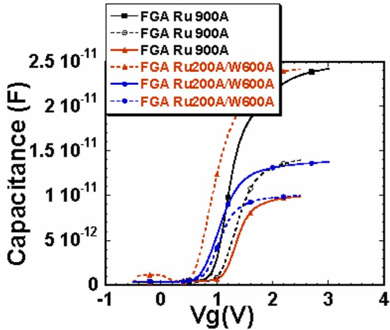
Figure 3. 1 C-V curves of Ru 200A with W 600A films and Ru 900A film on SiO<sub>2</sub> forming gas annealed at 400°C
