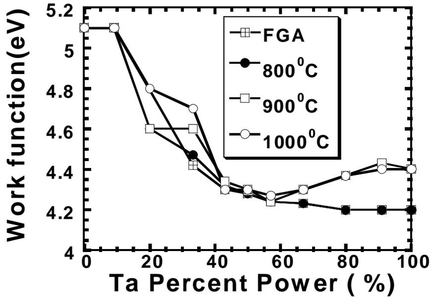
Figure 2. 3 Work function extracted from CV curves vs. Ta percent power annealed at 800°C, 900°C and 1000°C. The alloys with Ta percent power less than 60% remain stable under high temperature anneals [3]
