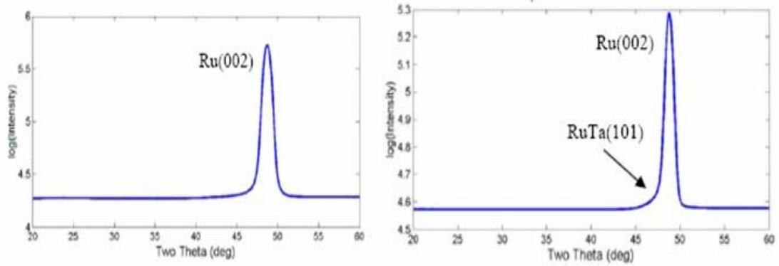
Figure 4. 24 The in-situ XRD data of 500A Ru / 30A RuTa / SiO2 (a) As-deposited (b) after 1100°C anneal
