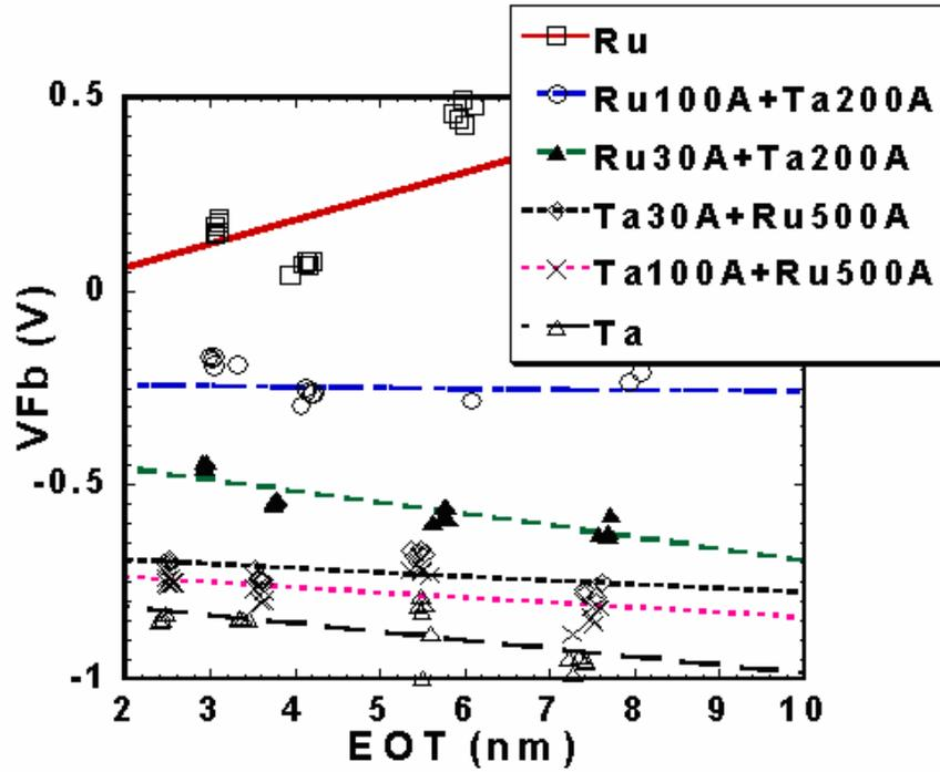
Figure 4.3 Vfb vs. EOT for various metal gate stack conditions
