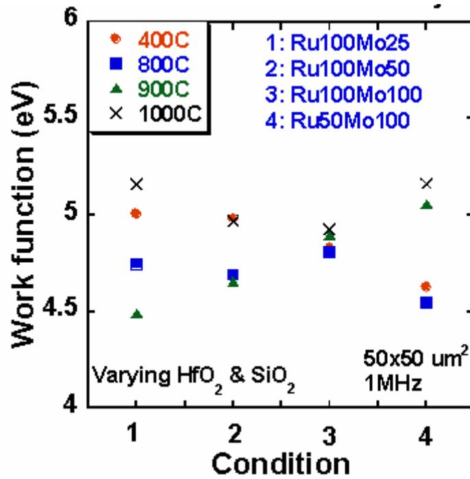
Figure A. 10 1<sup>st</sup> exp. Work functions of as Ru-Mo on varying HfO<sub>2</sub>/SiO<sub>2</sub> after different temperature anneal
