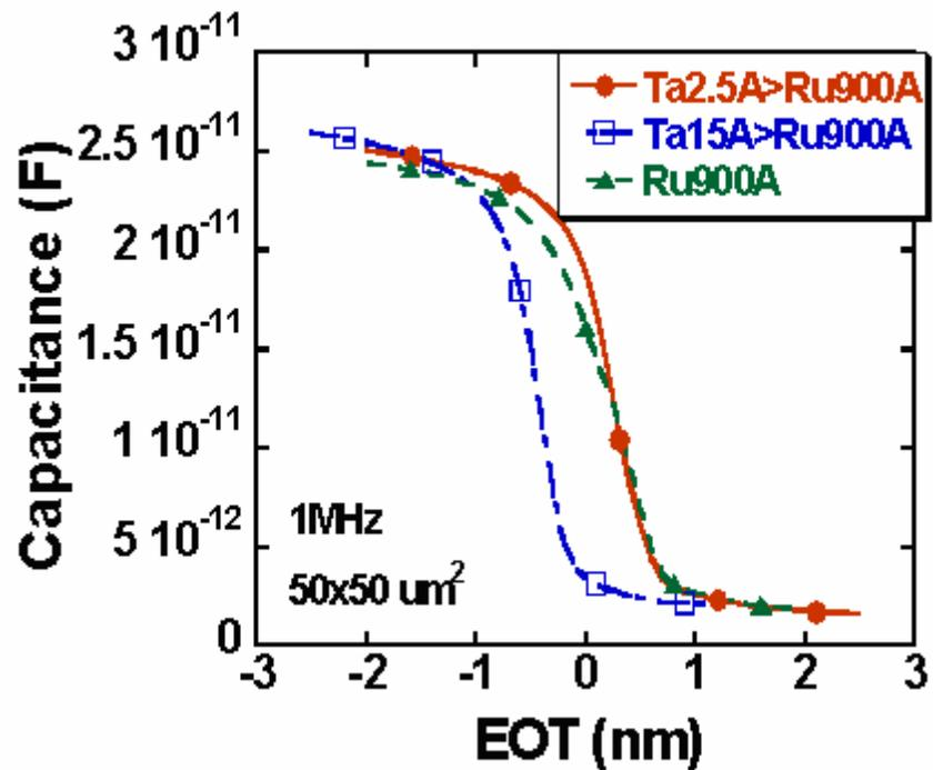
Figure 4. 26 C-V curves for Ta with Ru overlayer gate stacks forming gas annealed at 400°C
