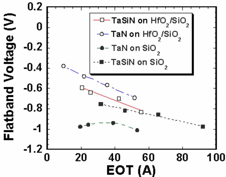
Figure 2. 16  $V_{FB}$  vs. EOT for TaN and TaSiN on  $\text{SiO}_2$  and  $\text{SiO}_2/\text{HfO}_2$  stack. The N diffusion is suppressed through  $\text{HfO}_2/\text{SiO}_2$  stack. The work function of TaN is midgap.
