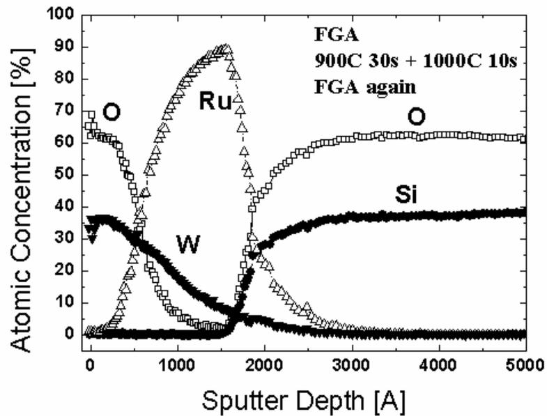
Figure 3. 6 AES Depth profile of Ru 700A with W 600A films on  $\text{SiO}_2$  with pre-FGA at 400°C and subsequent 900°C and 1000°C anneal in Ar followed by FGA at 400°C. Shows how much oxygen diffuse Ru film at high temperature
