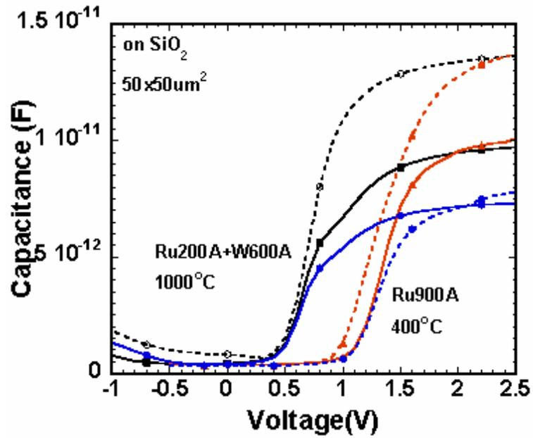
Figure 3.4 C-V curves of Ru 200A with W 600A films on SiO<sub>2</sub> annealed at 1000°C with pre-FGA at 400°C and Ru 900A film forming gas annealed at 400°C
