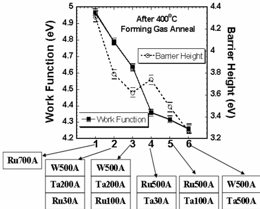
Figure 4.4 Work function extracted from C- V curves for various conditions of Ru and Ta stacks.
