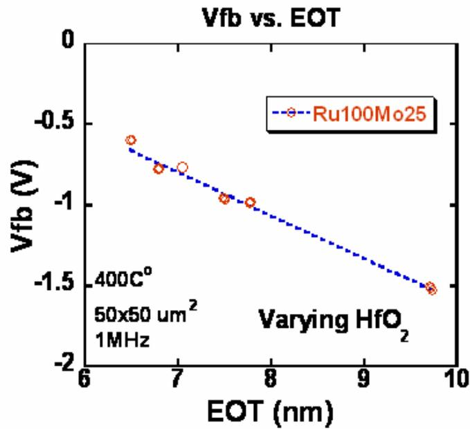
Figure A.3  $V_{FB}$  vs. EOT of as Ru100W-Mo25W on varying SiO<sub>2</sub> with 40Å HfO<sub>2</sub> after 400°C FGA
