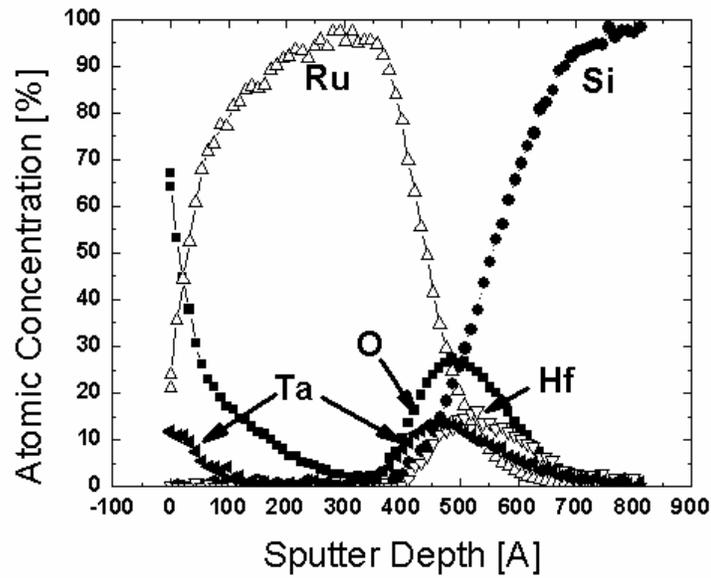
Figure 5. 14 AES depth analysis of Ru 500A with the underlayer of Ru<sub>50</sub>Ta<sub>50</sub> 100A on HfO<sub>2</sub>/SiO<sub>2</sub> after annealing at 800°C for 10min.
