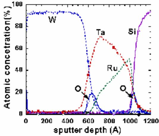
Figure 4. 12 (a) Auger Depth Profile after annealing of Si/SiO<sub>2</sub>/Ru 100Å/Ta 200Å/W 500Å
