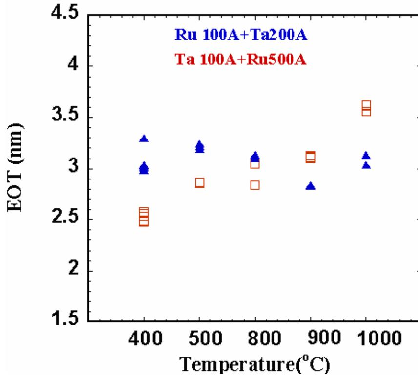
Figure 4. 7 EOT Stability Under High Temperature
