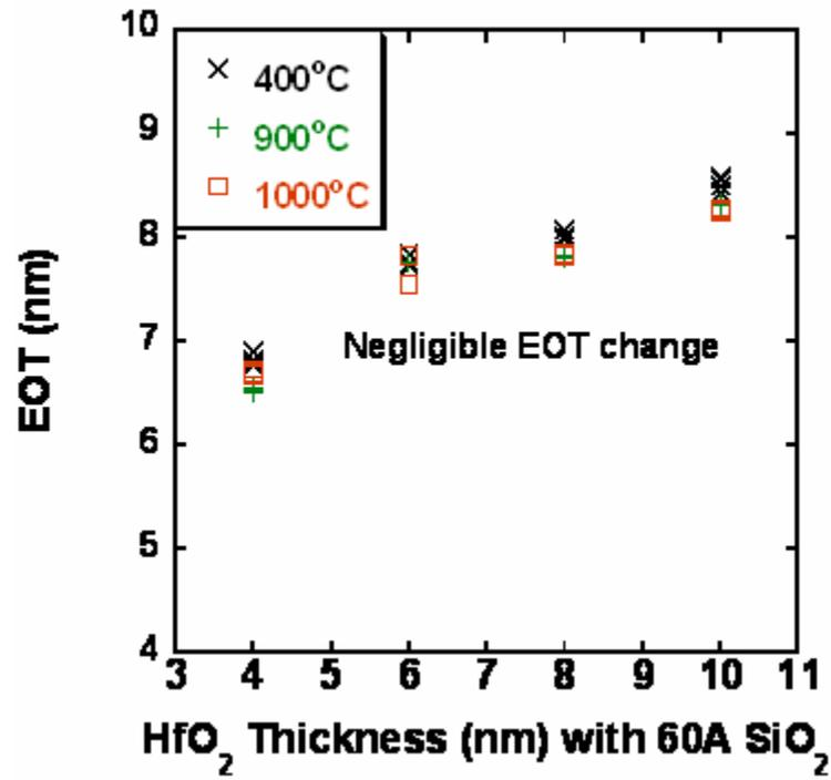
Figure A. 9 change of as Ru 100W Mo 25W on varying HfO<sub>2</sub> after different anneal
