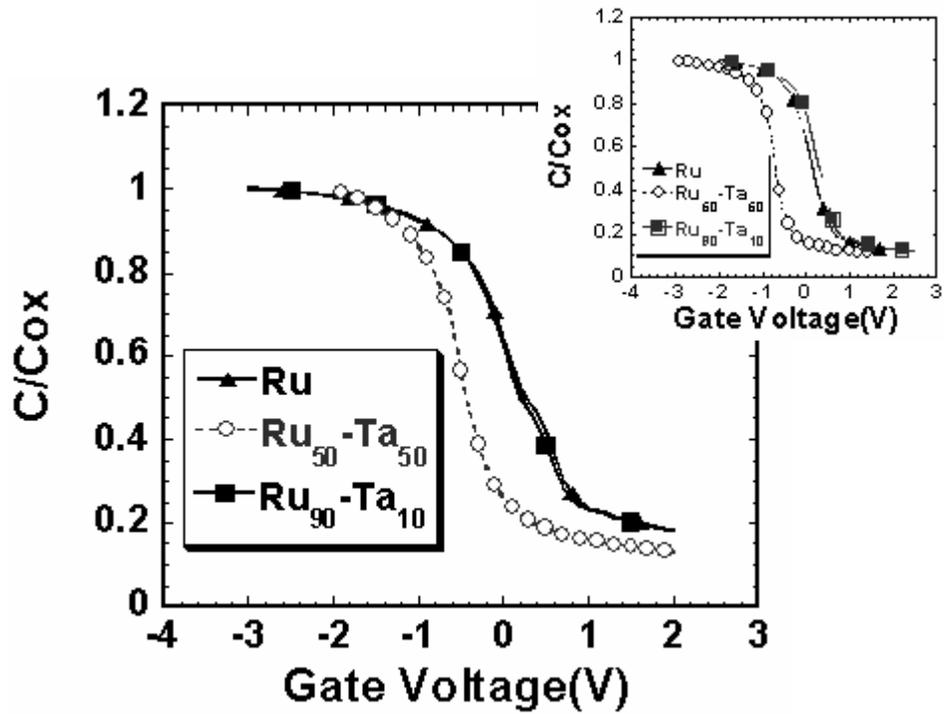
**Figure 2. 7 1 MHz C-V curves of Ru based metal electrodes on  $\text{HfO}_2$  gate Dielectrics. EOT down to  $11\text{\AA}$  have been obtained. Inset shows the same electrodes on  $\text{SiO}_2$ .**
