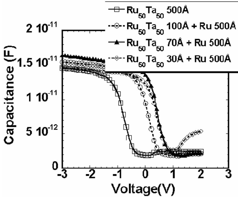
Figure 4. 19 C- V curves of Ru<sub>50</sub>Ta<sub>50</sub>/Ru stacks annealed at 800°C for 10min.
