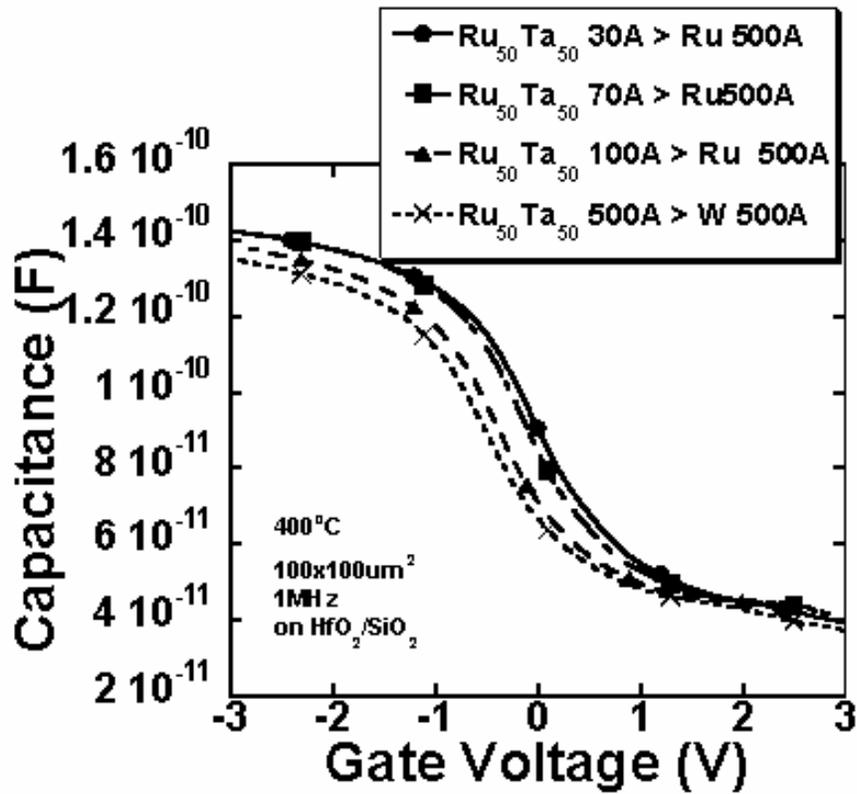
Figure 5. 2 C - V curves of stacked metal gates on HfO<sub>2</sub>/SiO<sub>2</sub> after annealing at 400°C
