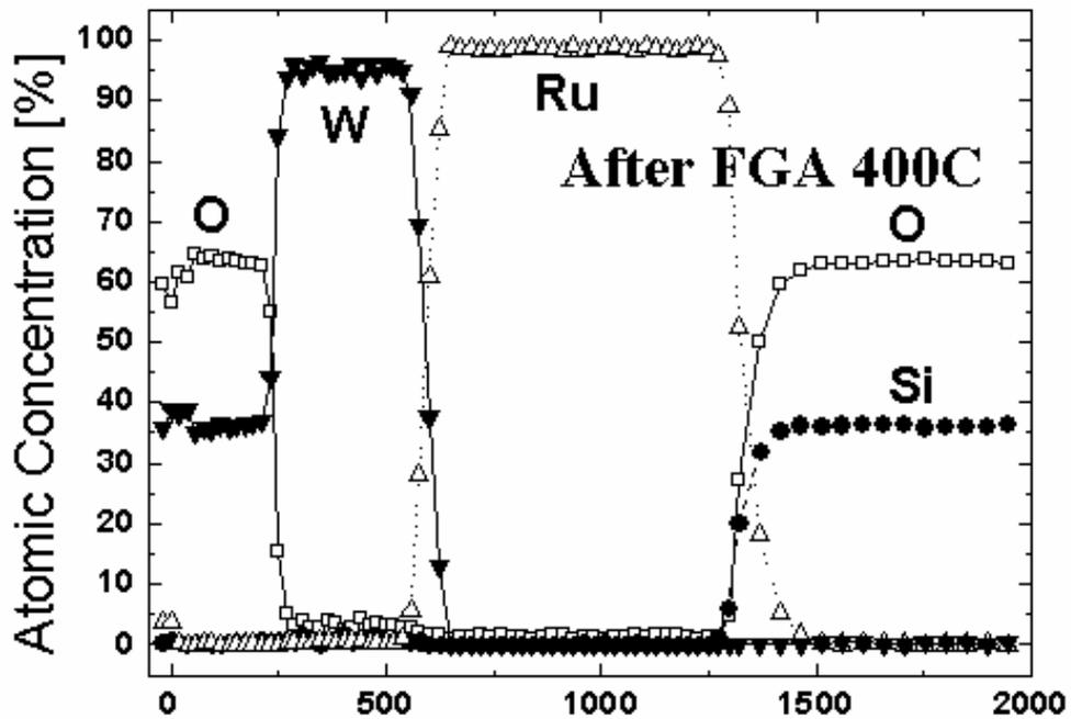
Figure 3. 2 AES depth profile of Ru 700A with W 600A films on SiO<sub>2</sub> after forming gas anneal at 400°C
