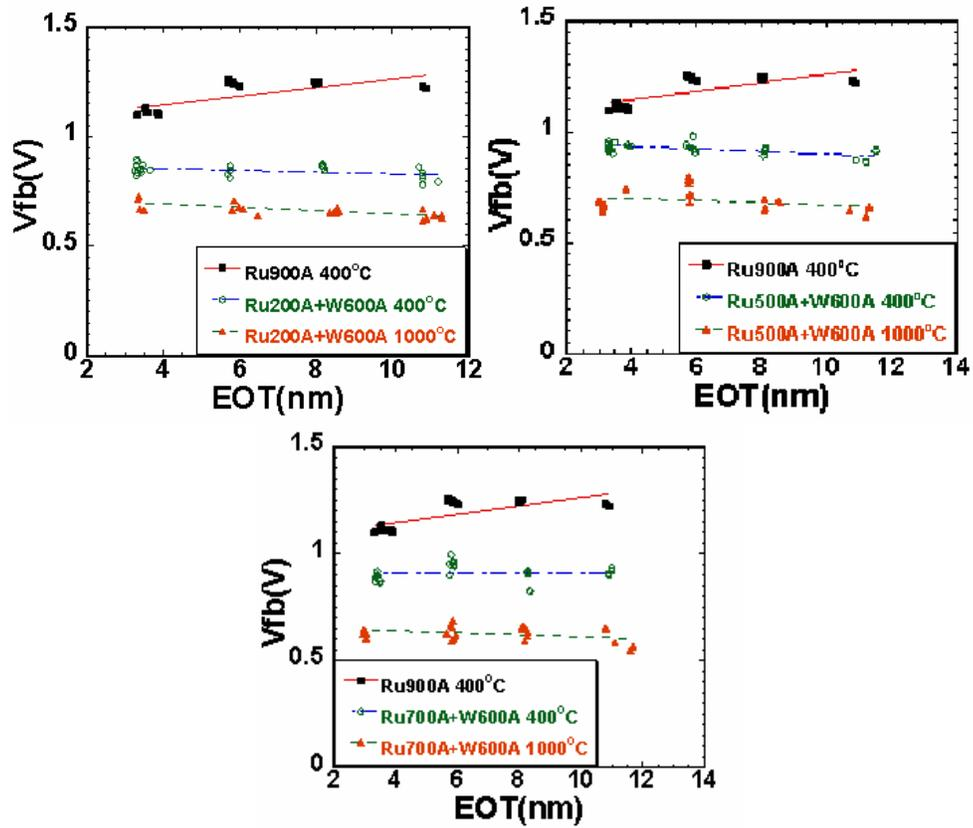
Figure 3. 5  $V_{fb}$  vs. EOT for various metal stack conditions FGA at 400°C and subsequent 1000°C anneal in Ar.
