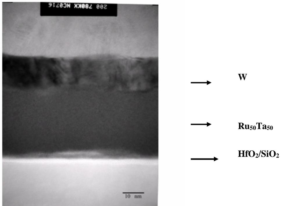
Figure 5. 12 TEM image of Ru<sub>50</sub>Ta<sub>50</sub> 100A with W capping layer on HfO<sub>2</sub>/SiO<sub>2</sub> after annealing at 400°C
