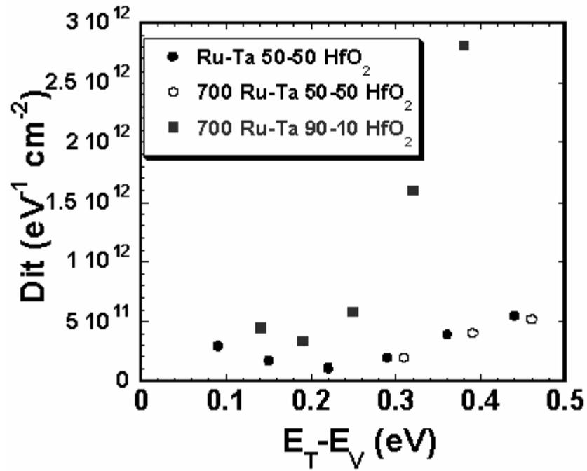
Figure 2. 23 Interface state density via conductance method as a function of anneal temperature for metal gates on  $\text{HfO}_2$
