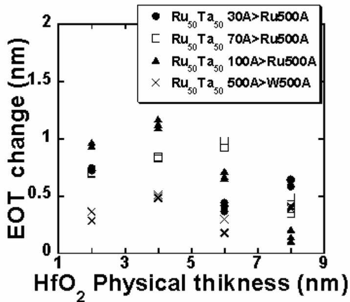
Figure 5. 7 EOT change vs. HfO<sub>2</sub> physical thickness curve of stacked metal gates on HfO<sub>2</sub>/SiO<sub>2</sub> after annealing at 400°C
