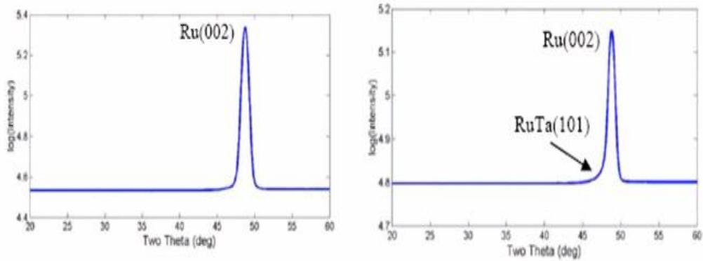
Figure 4. 22 The in-situ XRD data of 500A Ru / 100A RuTa / SiO<sub>2</sub> (a) As-deposited (b) after 1100°C anneal
