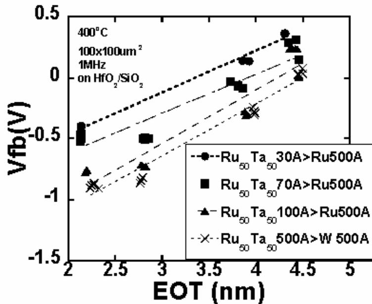
Figure 5. 5 Vfb vs. EOT curves of stacked metal gates on HfO<sub>2</sub>/SiO<sub>2</sub> after annealing at 400°C
