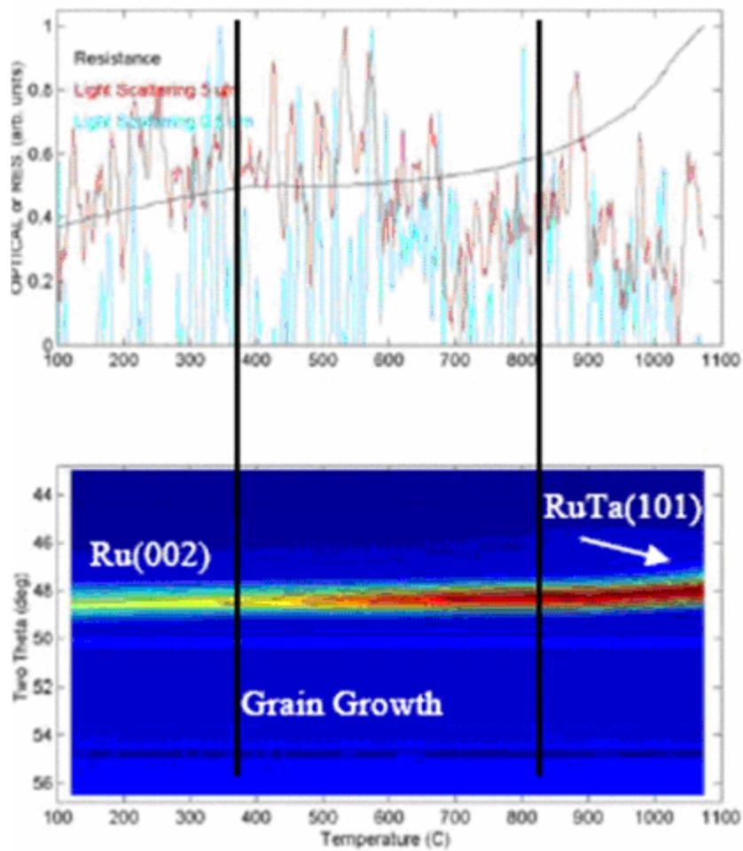
Figure 4. 15 In-situ XRD data of 500A Ru / 100A Ta on SiO<sub>2</sub> annealed from 100°C to 1100°C
