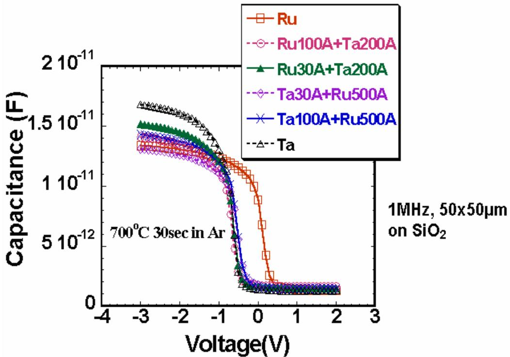
Figure 4. 6 C-V curves for stacked metal gates on SiO<sub>2</sub> after annealing 700°C 30s
