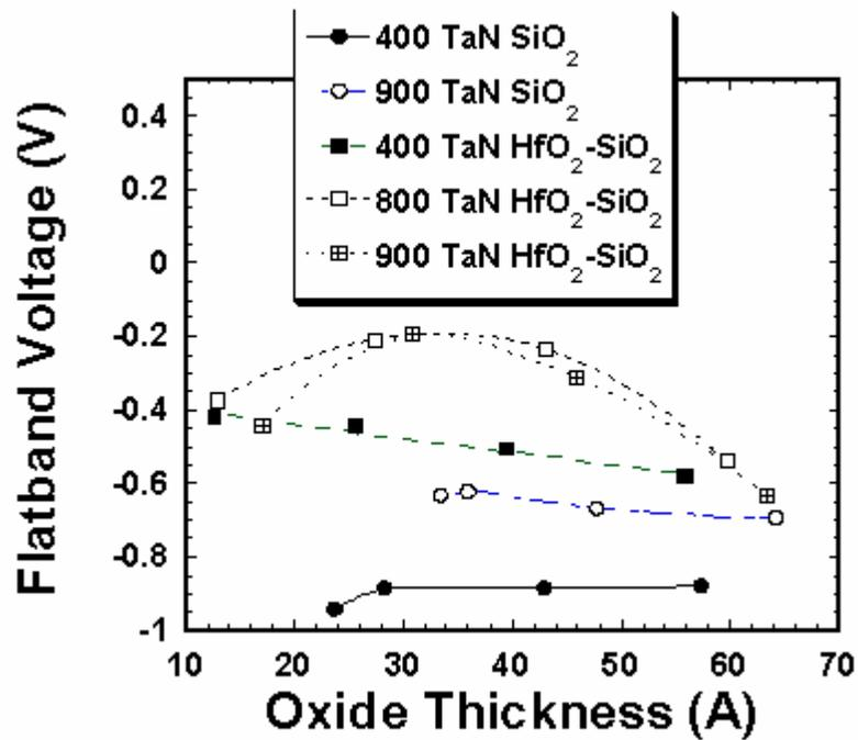
Figure 2. 22  $V_{FB}$  vs. EOT for TaN on  $HfO_2/SiO_2$  and  $SiO_2$  as a function of anneal temperature showing the improvement and charge.
