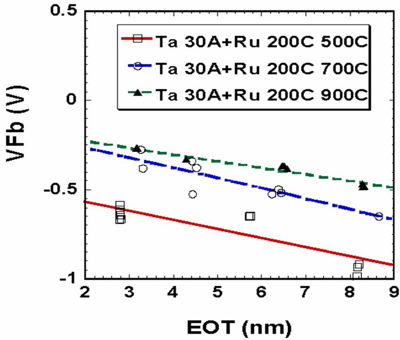
Figure 4. 9 Vfb vs. EOT of Ta/Ru stack for various temperature
