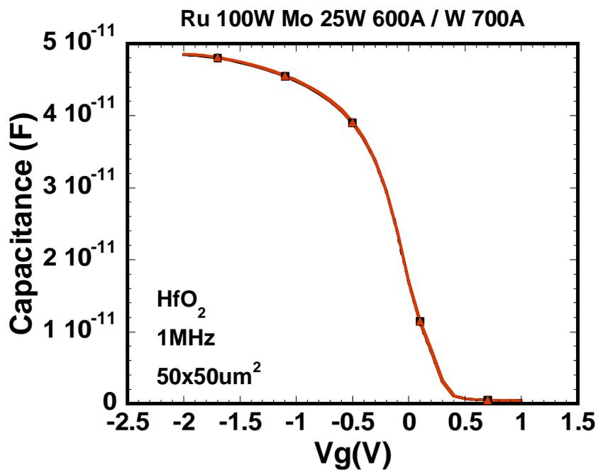
Figure A. 2 C-V curve of as Ru100W-Mo25W on varying HfO<sub>2</sub> after 400°C FGA
