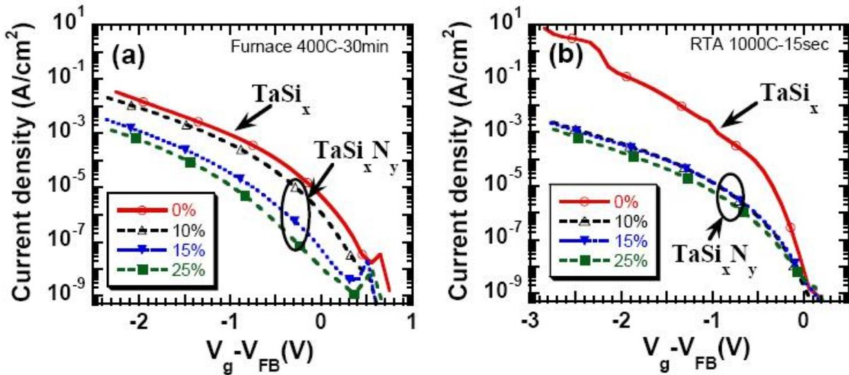
Figure 2. 6 Typical I-V curves of TaSixNy electrode capacitor with the N2 flow rate. (a) Furnace annealing at 400°C for 30min and (b) RTA at 1000 °C for 30sec.[9]
