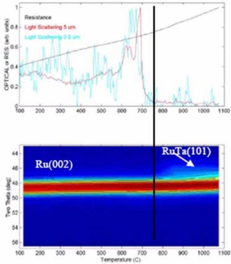
Figure 4. 23 The in-situ XRD data of 500A Ru / 100A RuTa / SiO<sub>2</sub> annealed from 100°C to 1100°C
