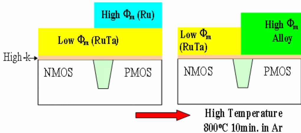
**Figure 5. 1 Integration approach for dual metal gate CMOS on high-k**
