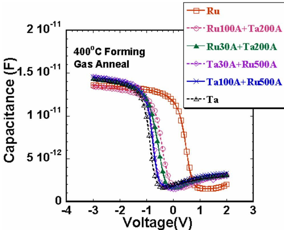
Figure 4. 2 C-V curves of stacked metal on  $\text{SiO}_2$
