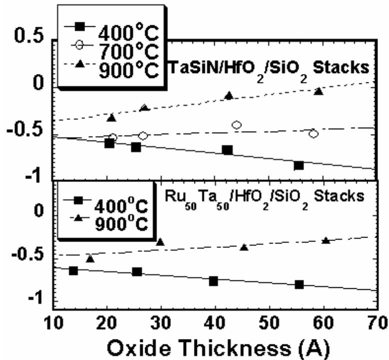
Figure 2. 20  $V_{FB}$  vs. EOT for  $\text{Ru}_{50}\text{Ta}_{50}$  and TaSiN on  $\text{HfO}_2/\text{SiO}_2$  as a function of anneal temperature showing the improvement and charge.
