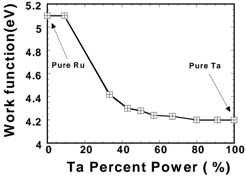
Figure 2. 1 Work function extracted from C-V curves for various compositions of Ru-Ta alloys. Non-linear behavior as a function of content is observed [3]
