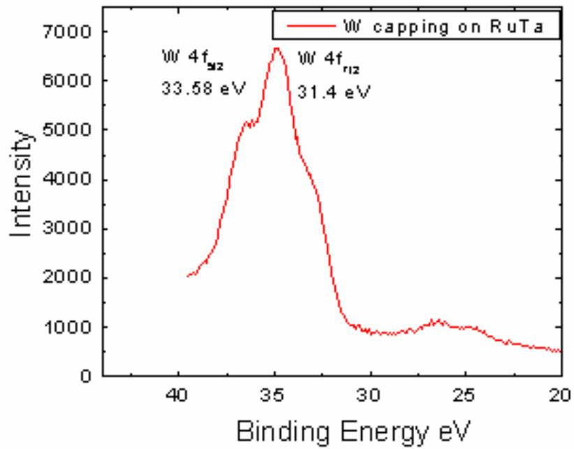
Figure 5. 11 XPS results of W 500A/RuTa 500A stacked metal gates after annealing at 800°C
