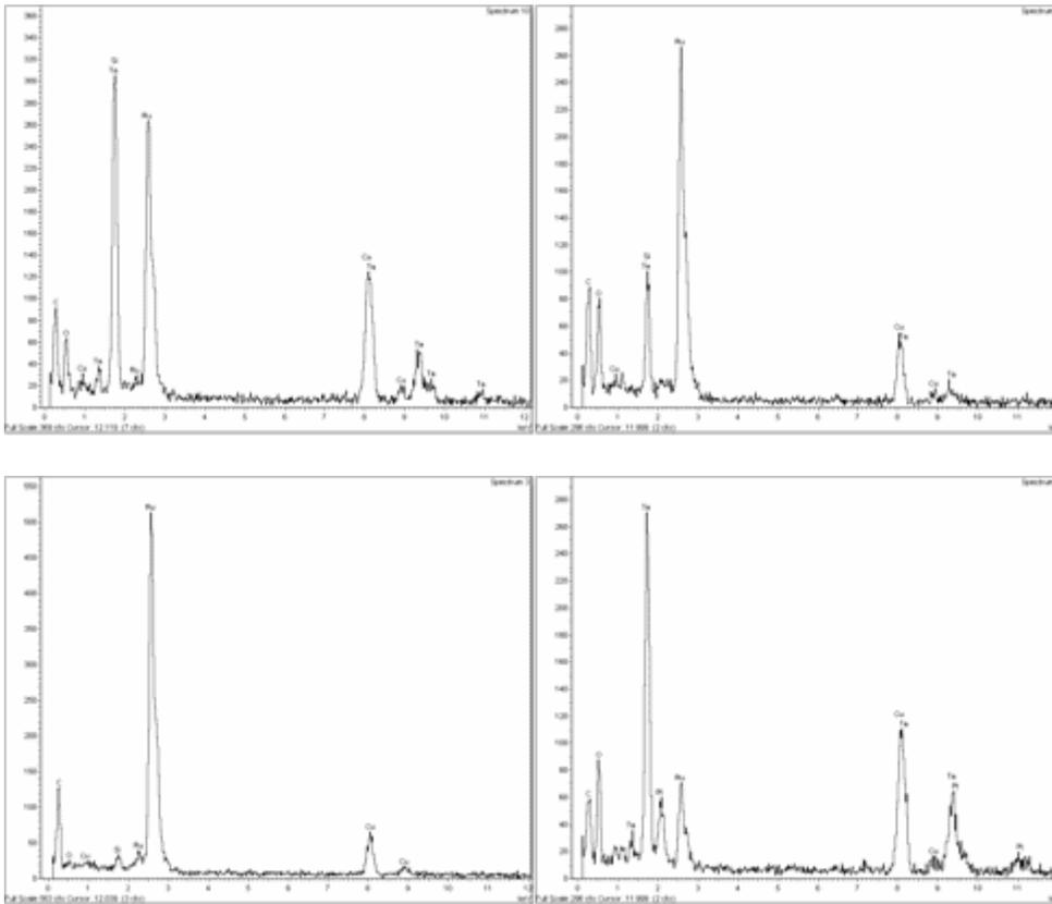
**Figure 5. 16 EDX/STEM analysis of Ru 500A with the underlayer of Ru<sub>50</sub>Ta<sub>50</sub> 100A on HfO<sub>2</sub>/SiO<sub>2</sub> after annealing at 800°C for 10min.**
