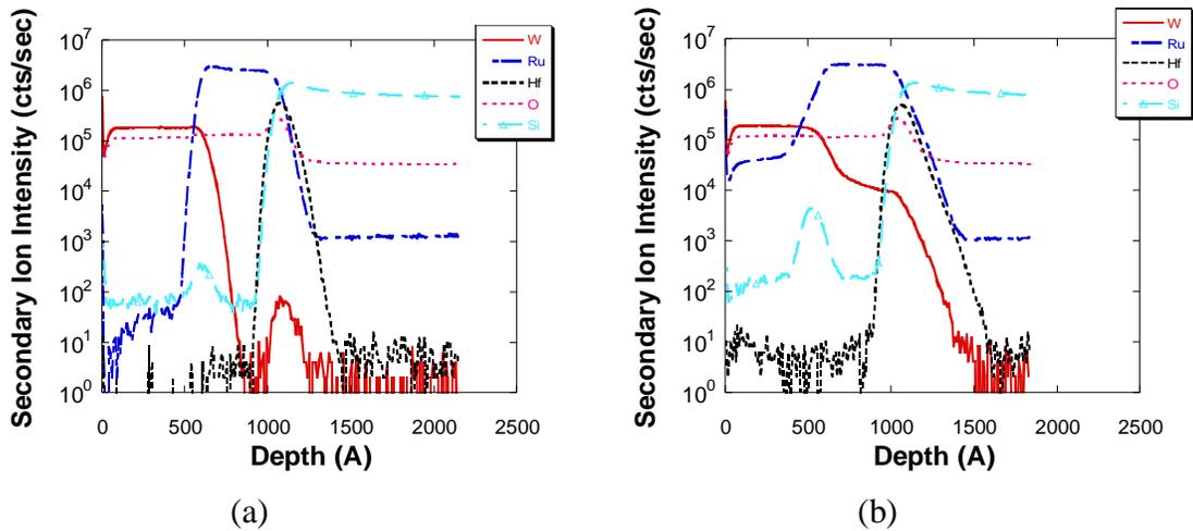
Figure 2. 24 SIMS profile analysis (a) as-deposited (b)  $900^\circ\text{C}$  anneal of W/Ru/ $\text{SiO}_2$
