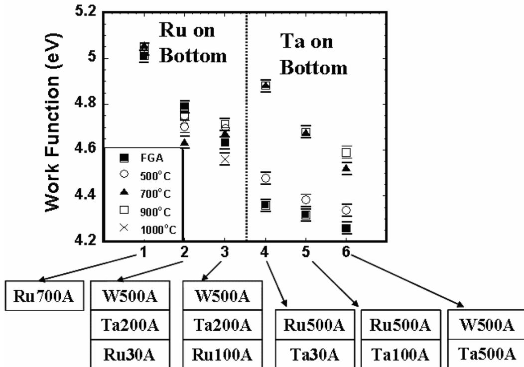
Figure 4. 10 Work function extracted from CV curves vs. Ta percent power annealed at 500°C, 700°C, 900°C and 1000°C.
