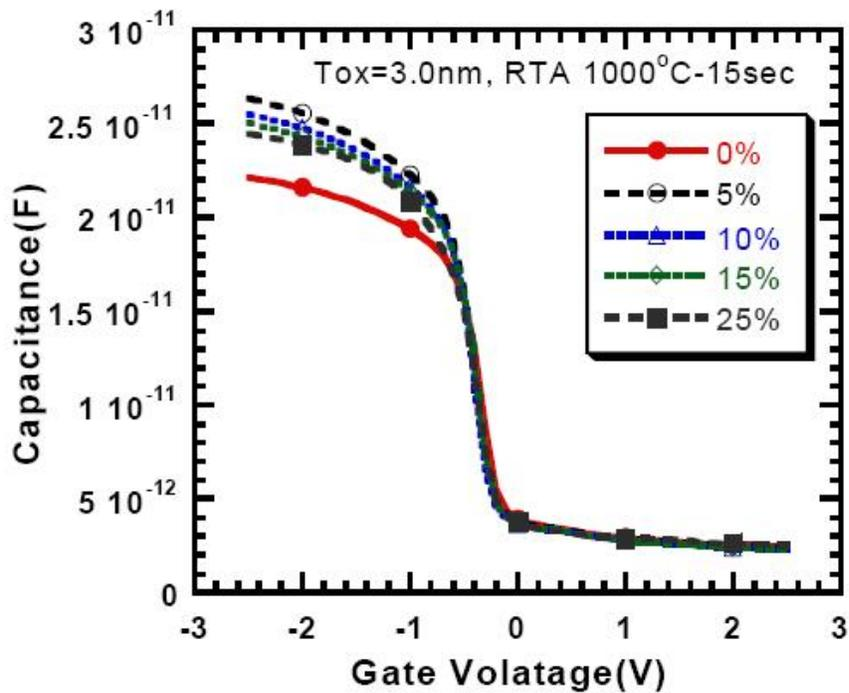
Figure 2. 4 Typical C-V curves of TaSixNy electrode capacitor with the N2 flow rate, after annealing at 1000°C for 30min. Capacitor area =2.5E-5cm<sup>2</sup> [8]
