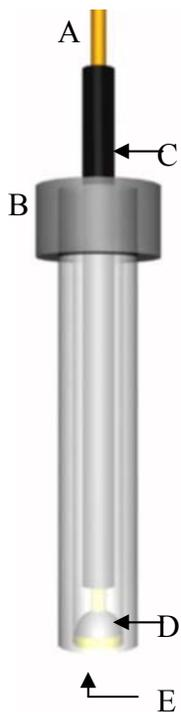
**Figure AII.2.** Silver Conductive Ink Electrode. A) Copper wire used to make electrical contact. B) Tygon tubing used to secure electrode to cell setup. C) Glass casing used to deliver conductive ink and shield wiring. D) Conductive ink creating interface between substrate and copper wiring. E) Substrate.
