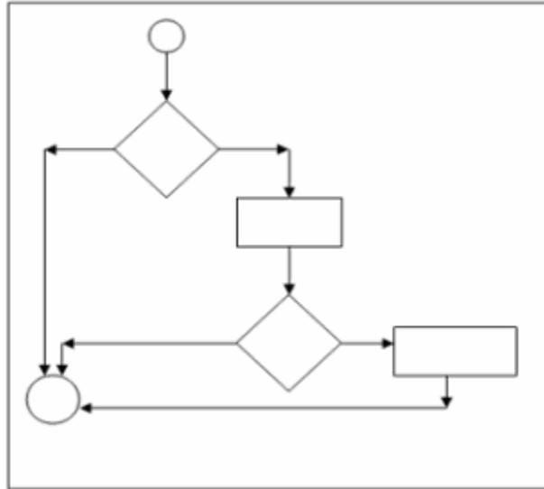
**Figure 4.3: Example cyclomatic complexity computation**
