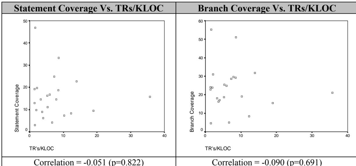
**Figure 7.5: Statement and Branch Coverage with TRs/KLOC**
