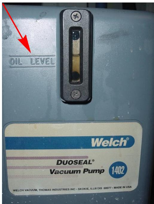
Step 33: Refill with clean vacuum pump oil to the top oil level mark shown above. Monitor the oil level between changes. If the oil level falls below the bottom mark, the vacuum capability of the pump will drop precipitously.
