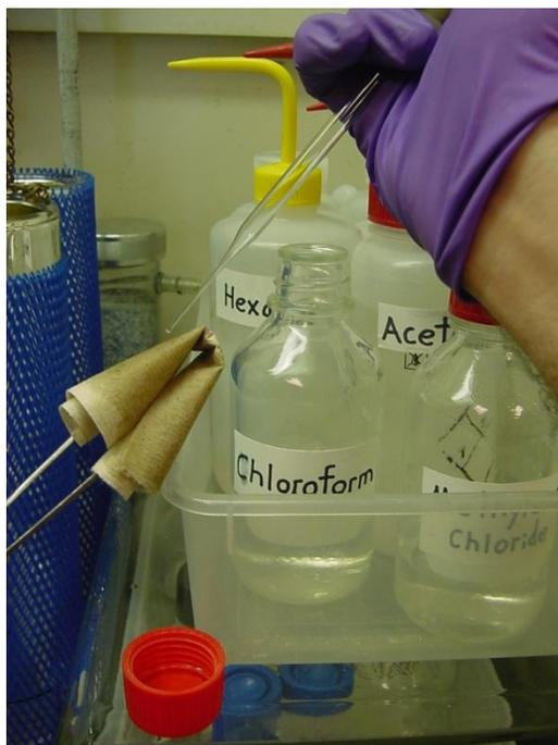
Step 13: Soak the paper towel with halogenated solvent. Chloroform works well for removing high vacuum silicon grease.
