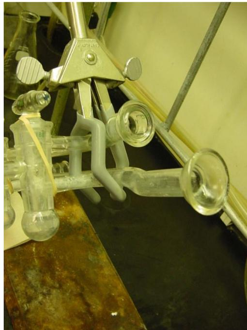
Step 2: Tighten a three-prong clamp on the manifold at the first set of joints from the open end of the vacuum line such that the two-pronged side of the clamp sandwiches the joints leading to the stopcock as illustrated.
