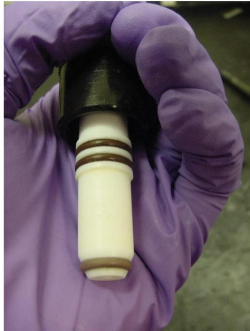
Step 36: Inspect the Teflon plugs. Replace the O-rings if they appear cracked or worn. Applying a very thin coating of Apiezon M grease to each O-ring is recommended, as doing so will allow the O-ring to slide on the glass with less friction.
