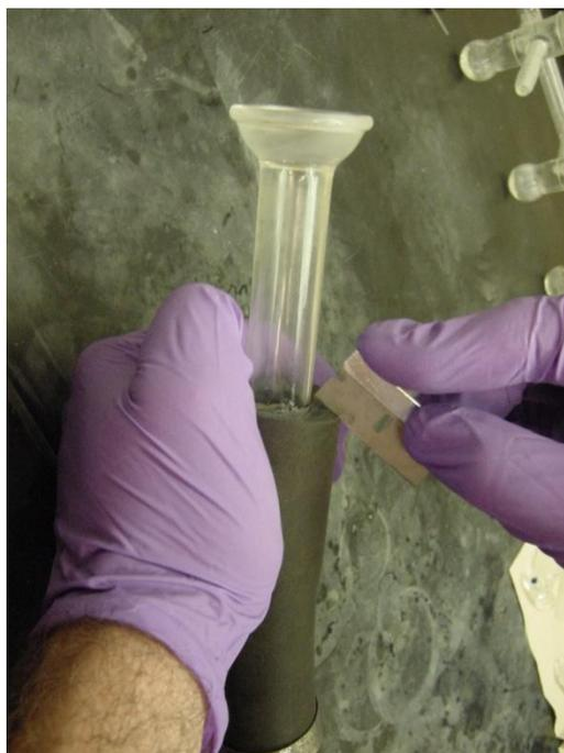
Step 21: Cleaning and applying a fresh coat of grease to the manifold / tube connection require removing the tubing from the glass. While taking care not to scratch the glass, cut along the length of the tubing with a razor blade until the glass stem can be pulled free.
