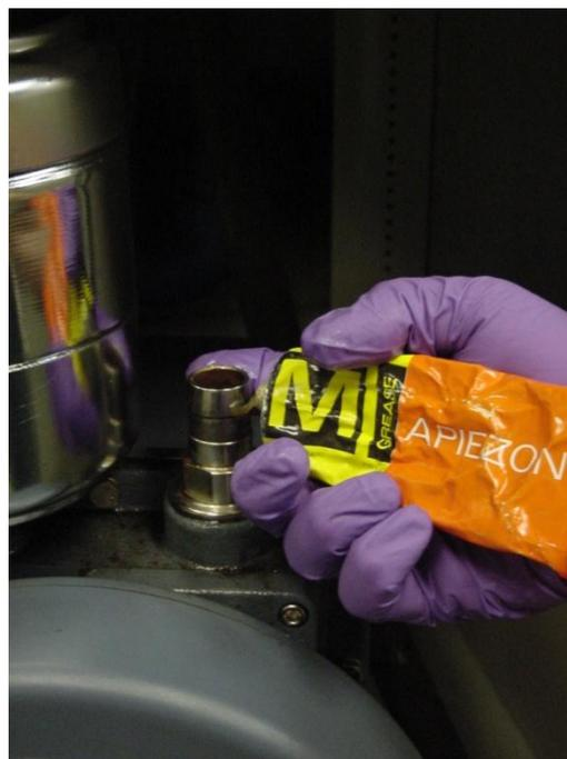
Step 34: Apply a fresh coat of Apiezon grease to the vacuum pump / tube connector and to the inside of the rubber tubing.
