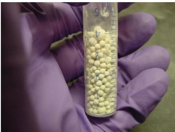
Step 9: Fill the syringe to the 4 mL mark with molecular sieves that have been oven dried overnight at 220 °C and cooled to room temperature in a desiccator.
