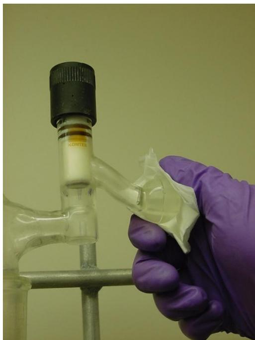
Step 17: Clean the ball and socket ends of each ball-and-socket joint with a solvent-soaked Kimwipe. Hexanes work well for removing Apiezon brand hydrocarbon greases.
