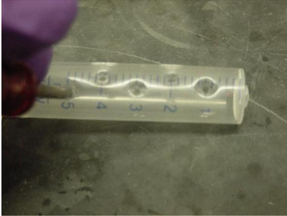
Step 5: Make a series of staggered puncher holes at the 2, 3, 4, & 5 mL marks as illustrated.
