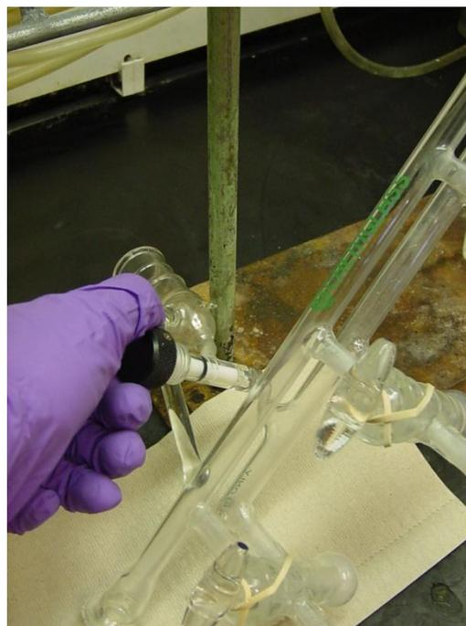
Step 4: Tighten the Teflon stopcock leading to the vacuum gauge joint until closed. [Don't forget to reopen this valve for a vacuum gauge reading upon reassembling the manifold and turning on the vacuum pump.]
