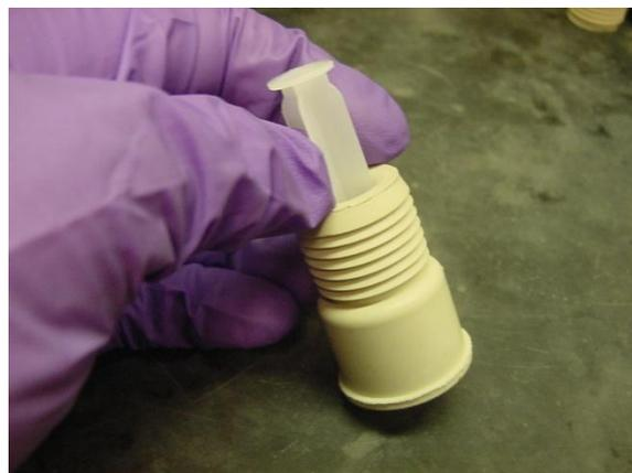
Step 10: Insert the cut end of the plunger into the underside of a Suba-Seal #45 Rubber Septum.
