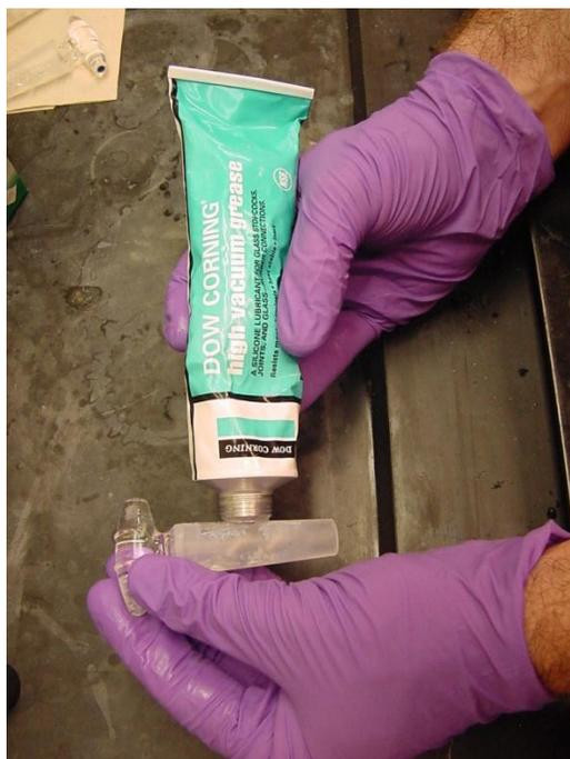
Step 15: Apply a fresh coat of silicon grease to each stopcock before returning it to its respectively-numbered joint. Dow Corning high vacuum grease is recommended for mobile joints such as stopcocks.
