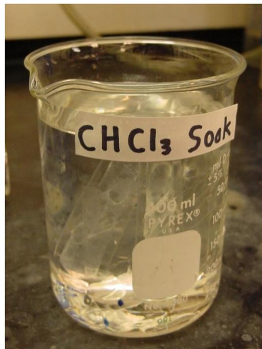
Step 8: Submerge each stopcock, handle down, in a beaker of halogenated solvent. For particularly difficult grease deposits, boil the solvent to facilitate the cleaning process. As with the vacuum line, soaking the stopcocks in aqua regia or a base bath for a few minutes may be advisable alternatives, depending on the contaminants to be removed.
