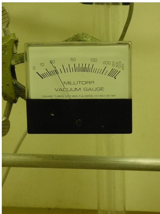
The manifold pressure should quickly fall to less than 100 mtorr. Without the use of liquid nitrogen in the cold traps, it may take several hours to reach maximum vacuum as the volatile components of the Apiezon grease off-gas, creating a virtual leak in the system. The pressure should drop steadily during this time. Once the pressure stabilizes, twist and press each stopcock, each cold trap, and each ball-and-socket joint again to ensure a maximum seal.
