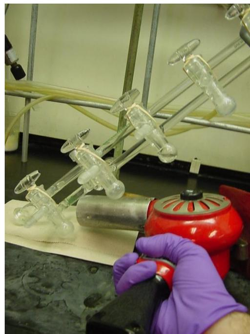
Step 6: Utilizing a heat gun to reflux the solvent in the vacuum line is a particularly effective way to dissolve large grease deposits. It is especially important that the valve leading to the air space within the stopcock is open to the vacuum line while heating, as vaporization of solvent and expansion of heated air within the stopcock might otherwise lead to a violently blowout.
