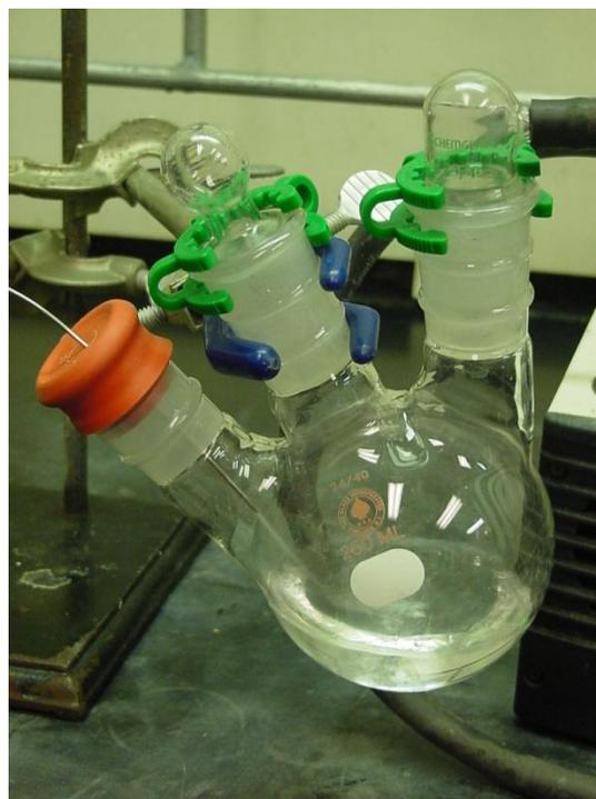
Step 16: The supernatant is sucked from the flask containing the precipitate to the 3-neck flask.
