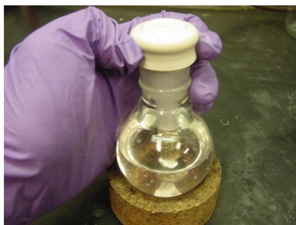
Step 12: Insert the molecular sieve holding device into the reaction flask and secure the septum.
