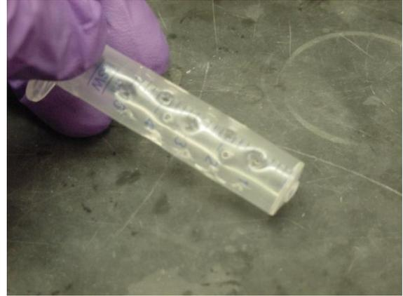
Step 6: Rotate the syringe 120° and repeat steps 4 & 5 to make a second line of staggered puncher holes. Repeat step 6 again to create a total of 15 puncher holes in the plastic syringe.
