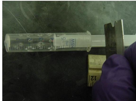
Step 8: Insert the plunger to the 4 mL mark. Measure and cut the end of the plunger as needed to fit the depth of the flask to be used.
