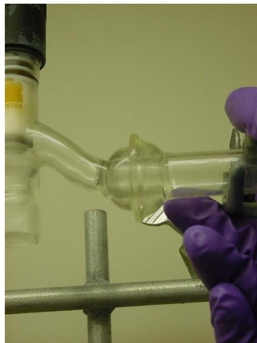
Step 42: Align each ball-and-socket joint. Twist the connection back and forth under vacuum to ensure a uniform coating of grease and a proper seal.
