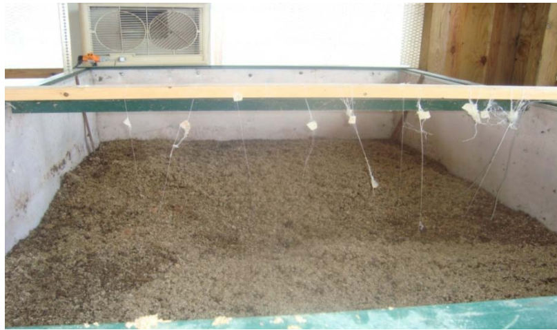
Figure 2.4. Vermicomposting bin with polypropylene samples hanging from the strings.
