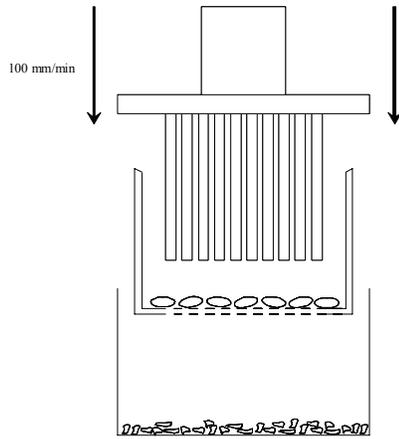
**Figure 2.2** Diagram of Kramer Shear Cell for oilseed textural analysis.
