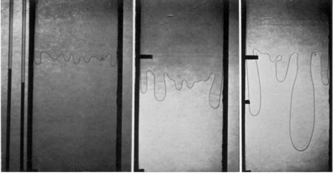
Figure 1.2: Development of the Saffman-Taylor viscous fingering instability for interface between air and glycerine in a Hele-Shaw cell, taken from [52]
