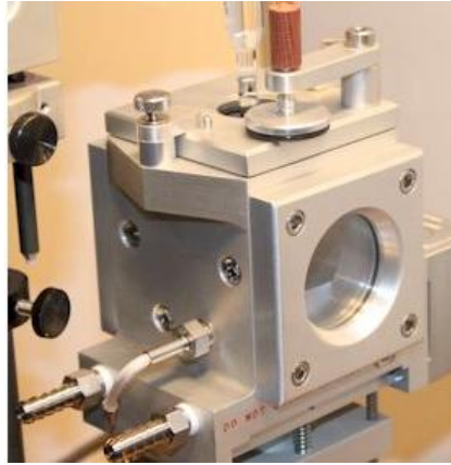
Figure 3.2: Environmental cell used to control environment during pendant drop method [3.14]
