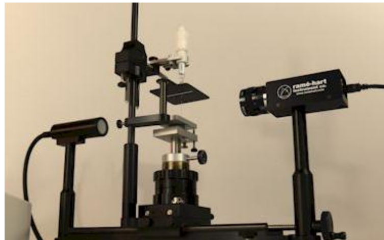
Figure 3.3: Advanced goniometer model 300 and CCD digital camera for drop image analysis [3.14]
