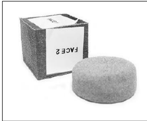
Figure 2.5. Image of solid Ti4Al4V (left) and sintered TiAl4V (right) used for 3D roughness analysis
