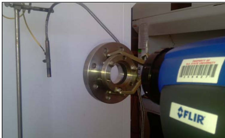
Figure 2.14. Viewport correction setup
