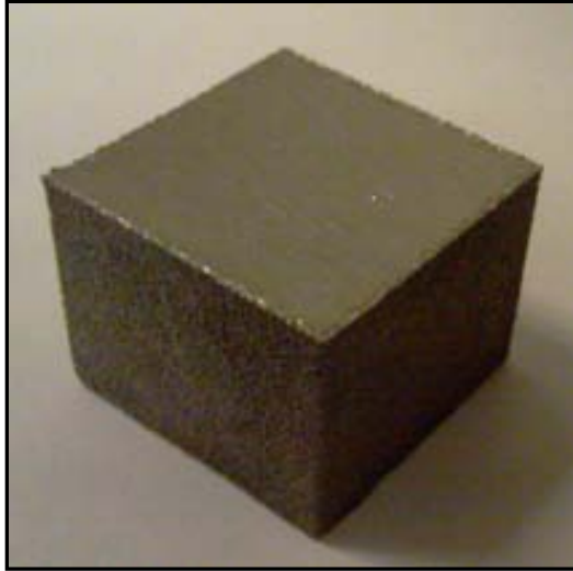
Figure 2.18. EBSM processed Ti6Al4V cube sample from PREP powder
