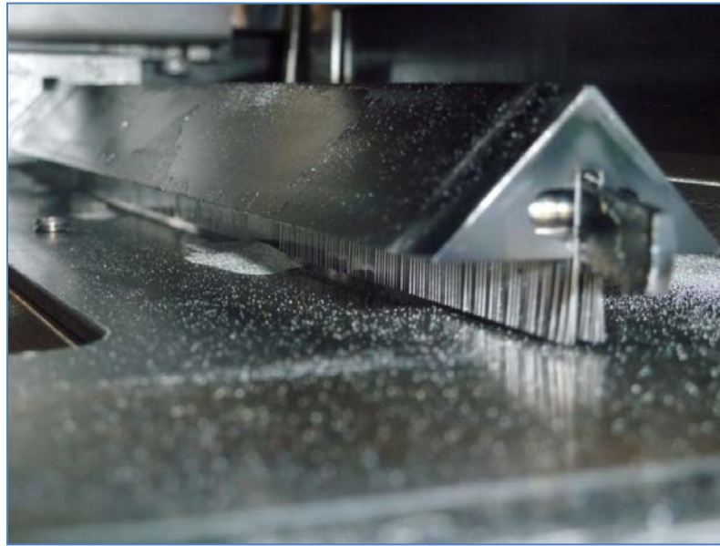
Figure 2.16. EBSM Powder Raking System
