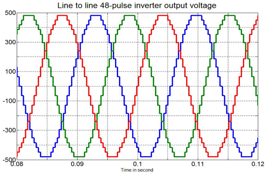
Figure 3-3. 48-pulse inverter line to line output voltages.
