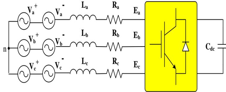
Figure 5-7. STATCOM equivalent circuit with series negative sequence voltage sources
