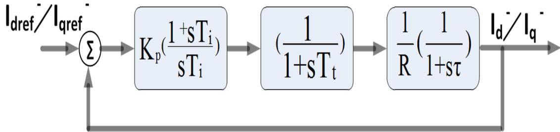
Figure 4-9. d and q current control loop [63]
