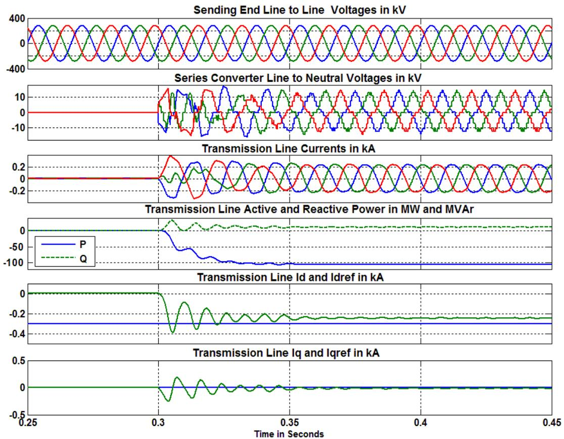
Figure 7-15. UPFC performance with a step change in the  $i_{d\text{ref}}$  (active power reference). UPFC series inverter is controlled with cross-coupling method.
