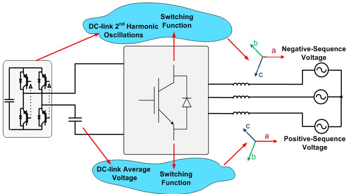
Figure 4-2. Simultaneous and independent control of positive and negative-sequence Voltage
