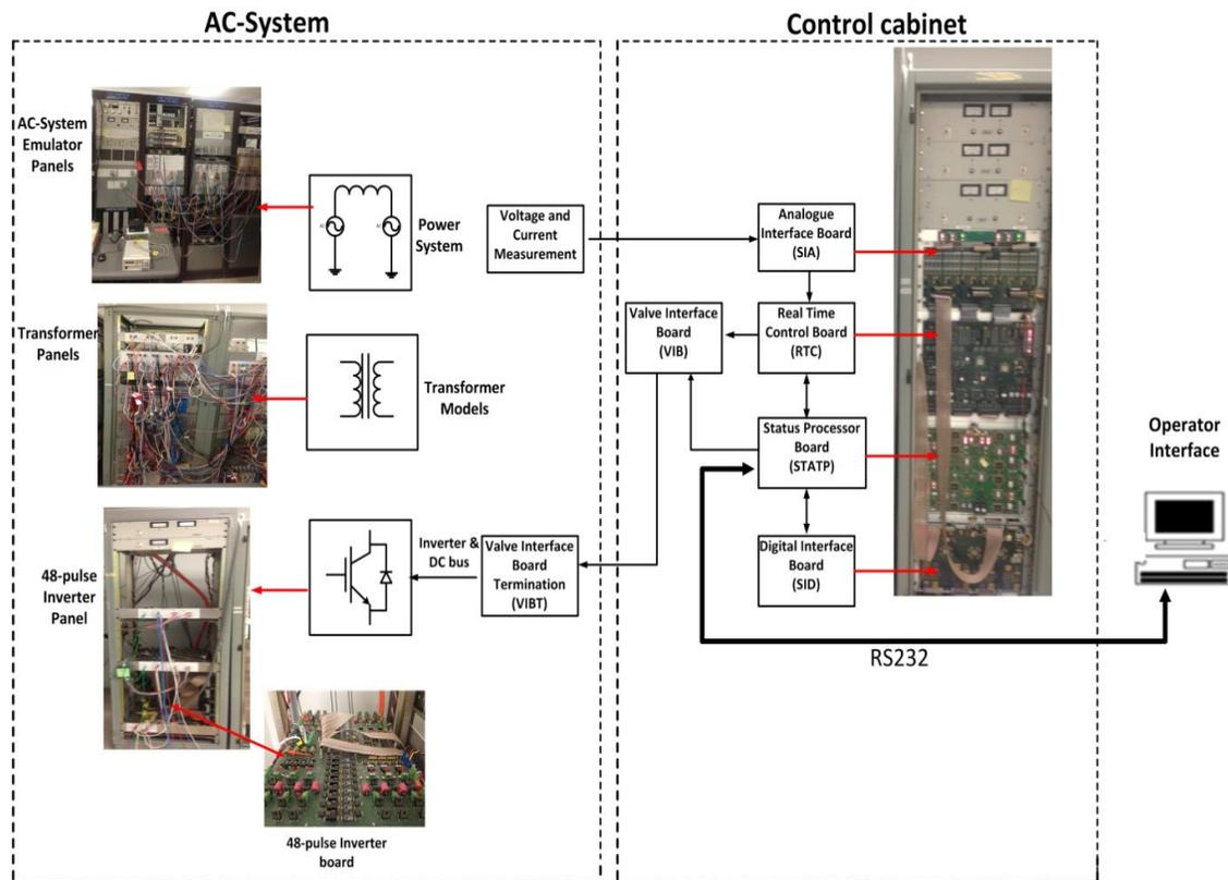
Figure 3-18. Interface of Control equipment to TNA
