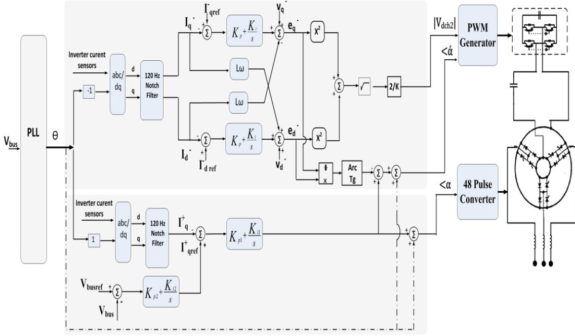
Figure 4-8. Control Structure
