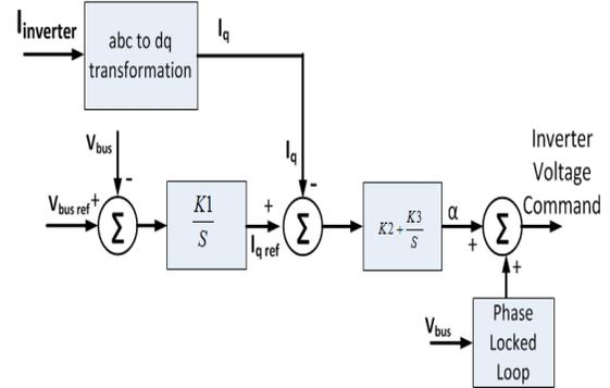
Figure 3-2. Control structure of an angle-controlled STATCOM.
