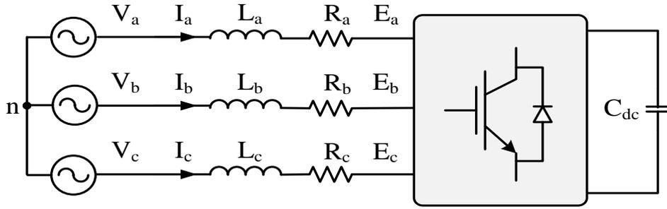
Figure 4-3. Equivalent circuit of a VSC connected to AC system.
