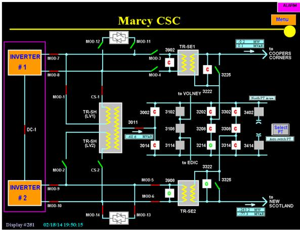
Figure 2-24. One-Line Diagram Screen
