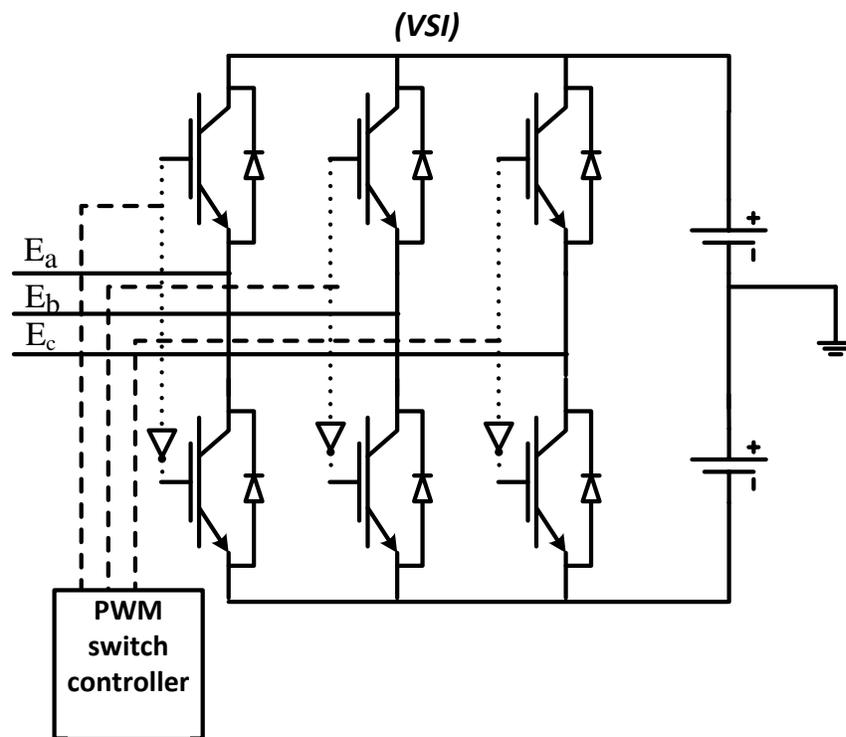
Figure 2-7. 2-level VSC-based PWM controlled inverter
