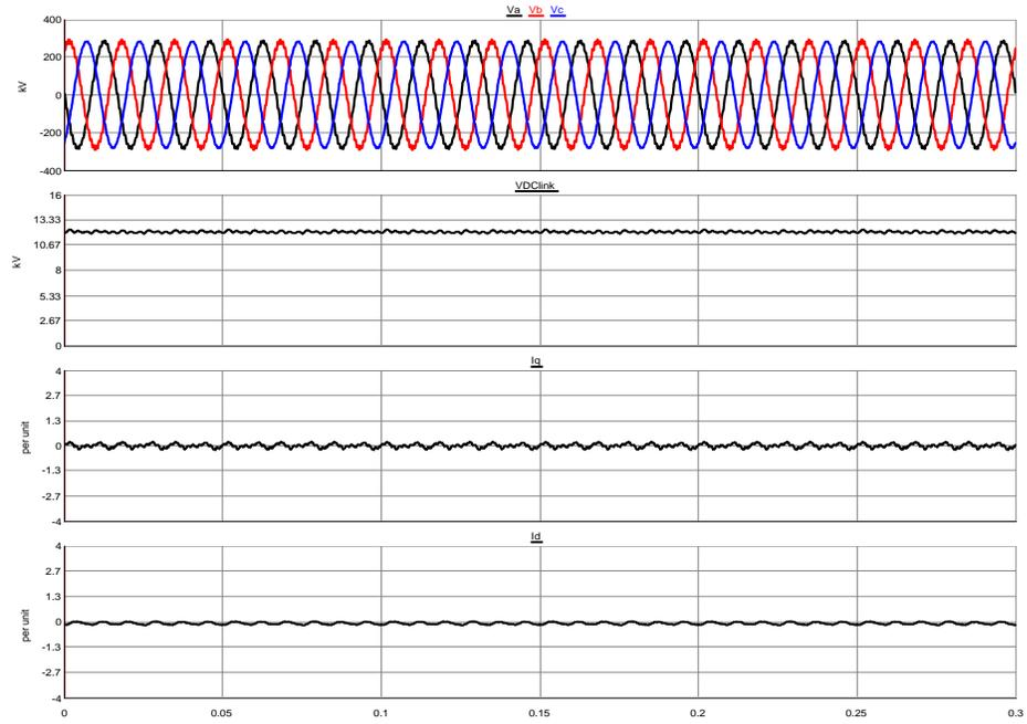
Figure 2-16. Angle-controlled STATCOM performance with  $i_q=0$
