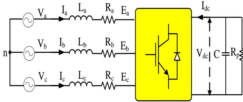
Figure 5-3. Equivalent circuit of an VSC connected to AC system
