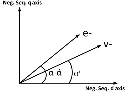
Figure 4-7. STATCOM instantaneous vectors in the negative synchronous frame
