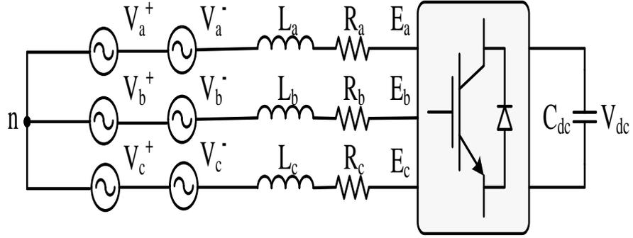
Figure 4-6. STATCOM equivalent circuit with series negative-sequence voltage sources
