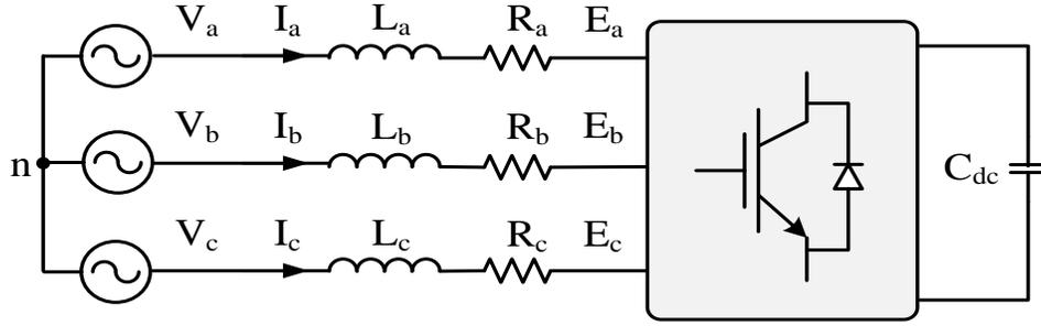
Figure 3-5. Equivalent circuit of a VSC connected to AC system.
