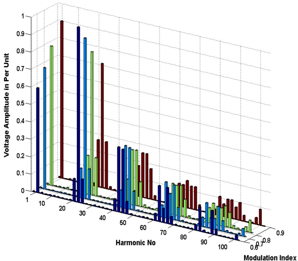
Figure 2-8. 2-level VSC-based PWM controlled inverter voltage spectrum with different modulation index
