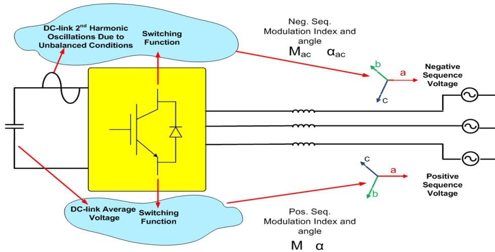
Figure 5-2. Simultaneous controlling of Neg. Seq. and Pos. Seq. voltages
