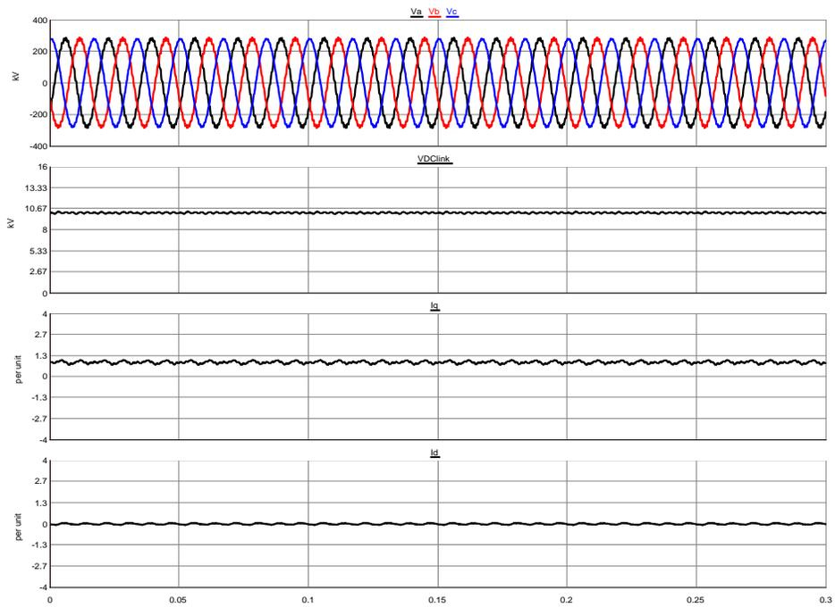
Figure 2-17. Angle-controlled STATCOM performance with  $i_q=1$  pu inductive
