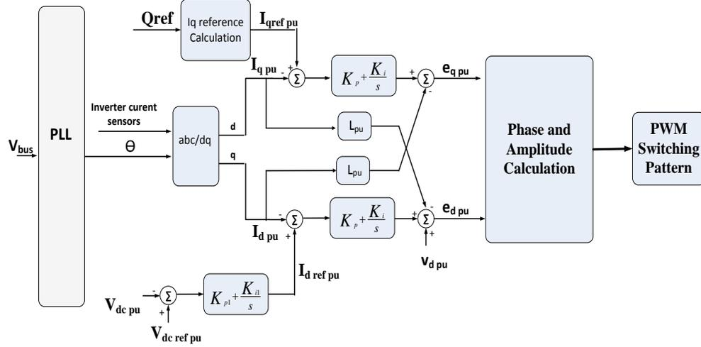
Figure 2-5. Vector controlled STATCOM control structure
