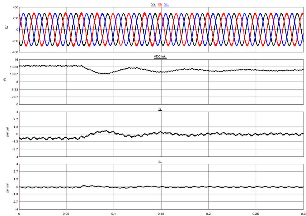
Figure 2-19. Angle-controller performance in transition from capacitive ( $i_q=-1$  pu) to zero current
