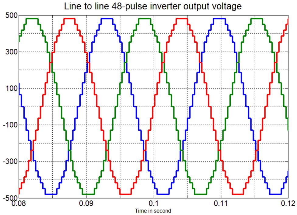
Figure 2-10. 48-pulse inverter line to line output voltages
