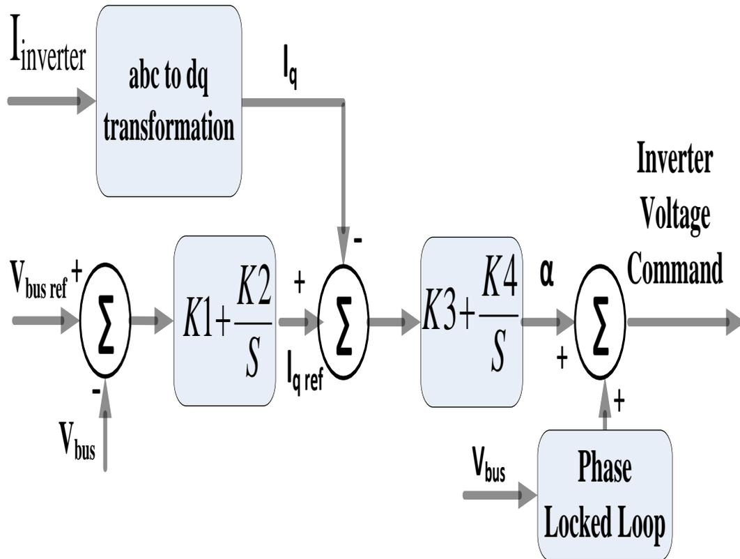
Figure 4-1. Control structure of an angle-controlled STATCOM
