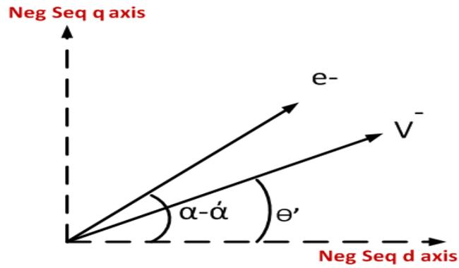
Figure 3-9. STATCOM instantaneous vectors in the negative synchronous frame
