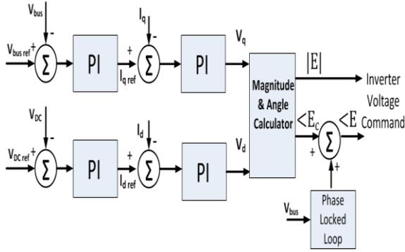
Figure 3-1. Control structure of a vector controlled (PWM) STATCOM.
