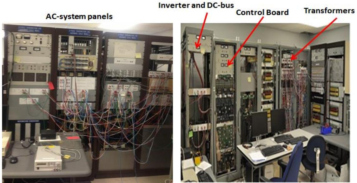
Figure 3-19. Control and magnetic panels
