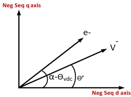
Figure 5-8. STATCOM instantaneous voltage vectors in the negative synchronous reference frame
