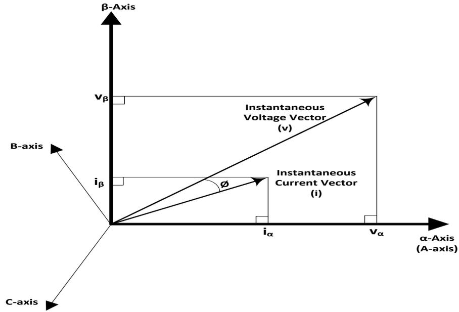
Figure 2-2. Instantaneous vectors in  $\alpha\beta$  coordinate system
