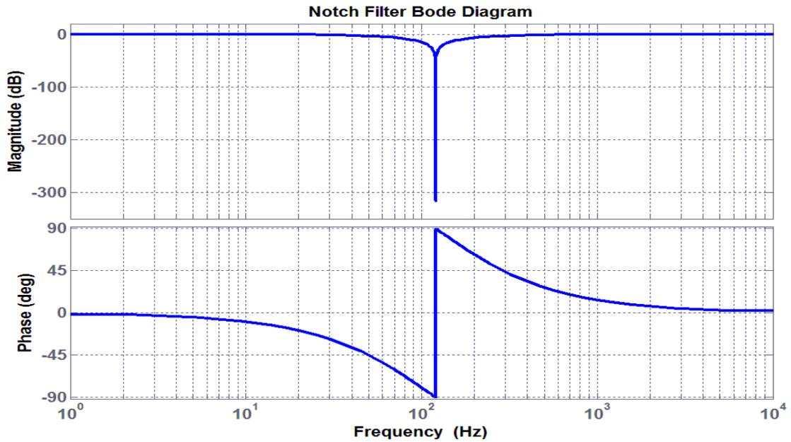
Figure 4-10. Notch filter bode plots
