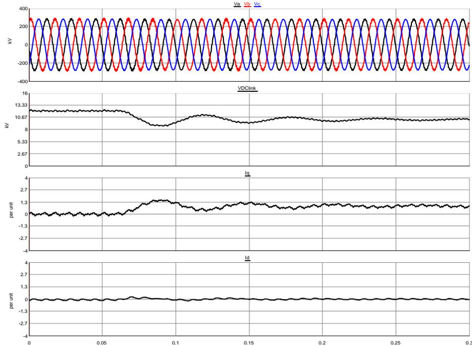
Figure 2-20. Angle-controlled STATCOM performance in transition from zero current to fully inductive ( $i_q=1\text{pu}$ )
