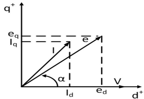
Figure 5-9. STATCOM vectors in the positive synchronous frame
