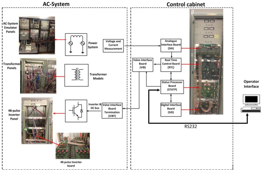
Figure 2-21. Interface of Control equipment to TNA
