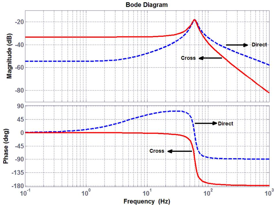
Figure 7-3. Bode plots of the direct and cross transfer functions.  $R=4\Omega$ ,  $L=0.123$  H (  $X/R=11.6$  ). The R, and L values are based on the 345 kV simulation AC-system explained in the section 7.7
