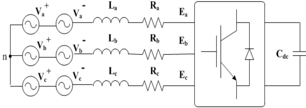
Figure 3-8. STATCOM equivalent circuit with series negative sequence voltage sources
