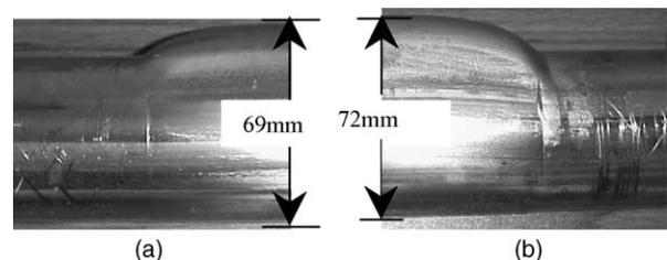
Fig. 12. Protrusion height for tube specimens after test: (a) non-lubricated; (b) lubricated.
