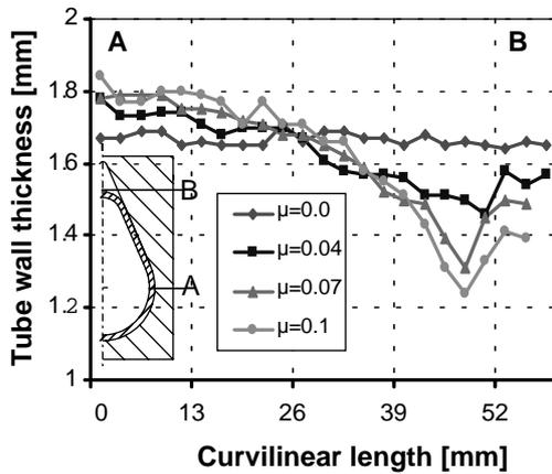
Fig. 8. Pear-shaped die with  $\alpha = 58^\circ$  wall thickness distribution ( $p_i = 200$  MPa).
