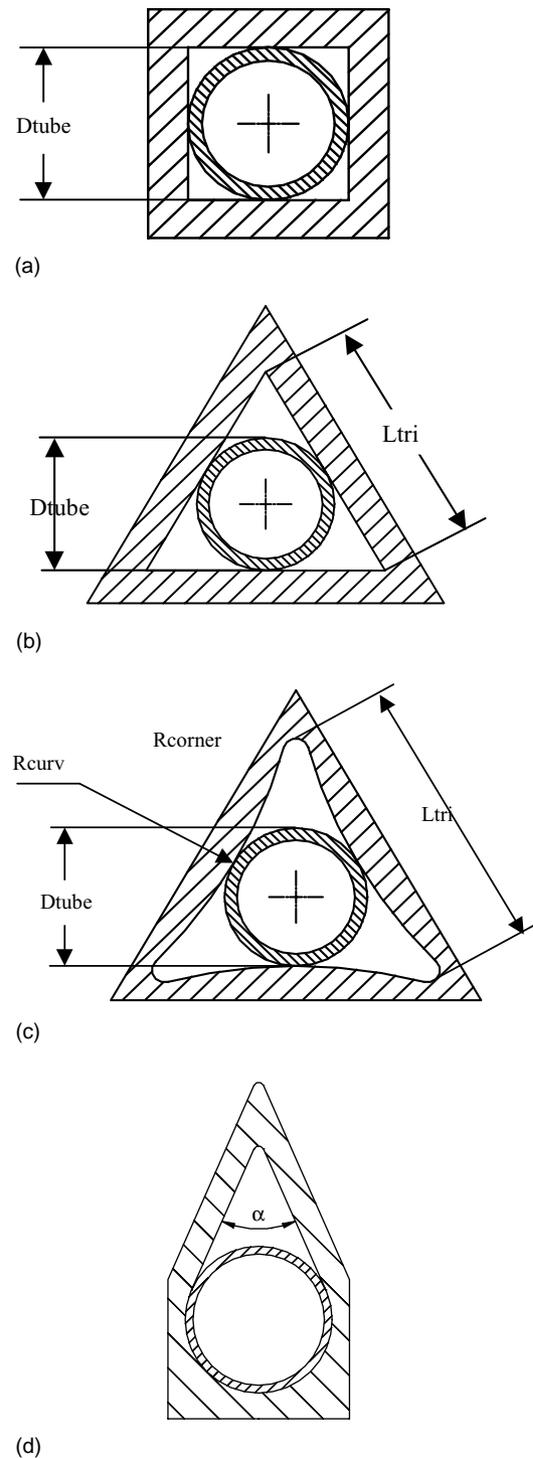
Fig. 7. Die geometrical configurations: (a) square die; (b) triangular die with flat surfaces; (c) triangular die with curved surfaces; (d) pear-shaped die.
