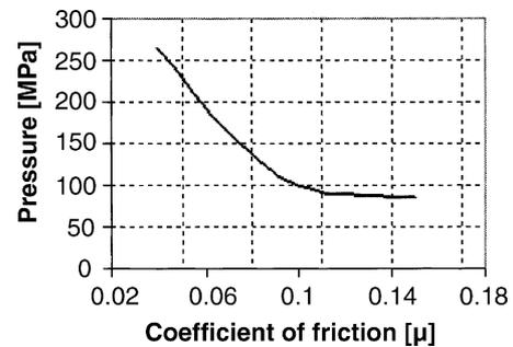
Fig. 11. Bursting (necking) pressure for different coefficients of friction.
