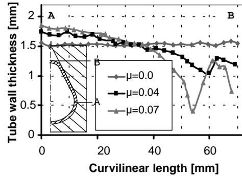
Fig. 10. Pear-shaped die with  $\alpha = 48^\circ$  wall thickness distribution ( $p_i = 200$  MPa).
