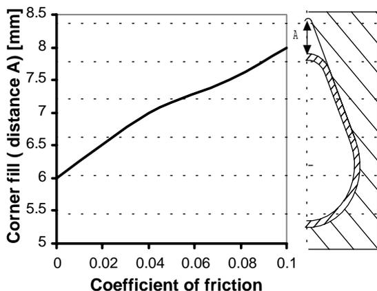
Fig. 9. Pear-shaped die with  $\alpha = 58^\circ$  corner fill ( $p_i = 200$  MPa).
