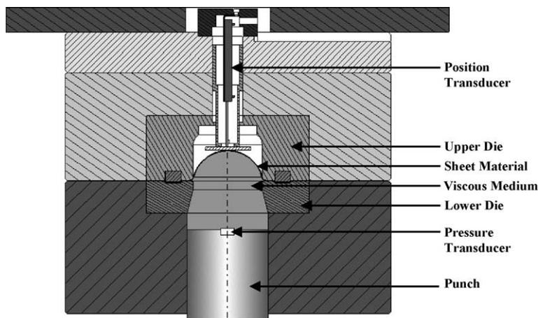
Fig. 2. Sketch of tooling used in the VPB test.
