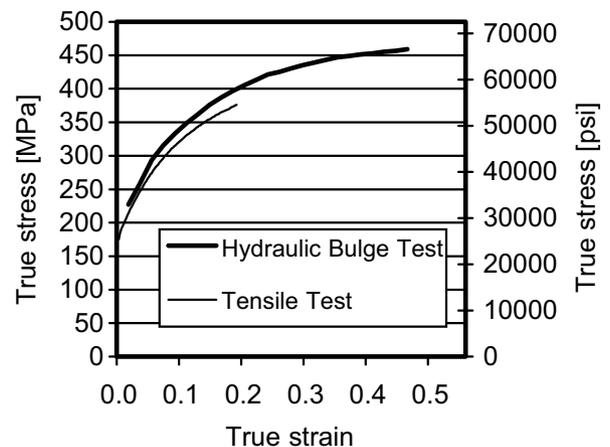
Fig. 14. Flow stress curves of aluminum AA 6111.
