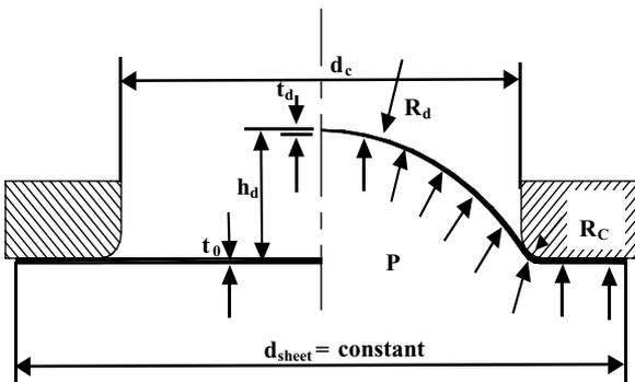
Fig. 1. Geometry of the bulge test.
