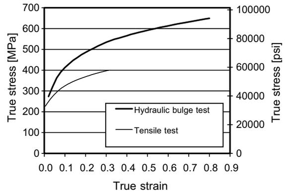
Fig. 12. Flow stress curves of AKDQ steel.
