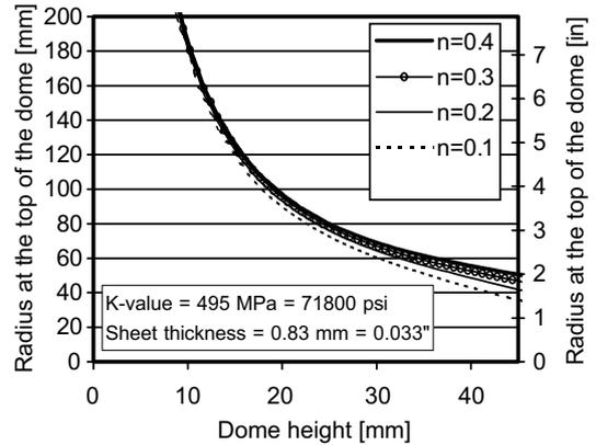
Fig. 6. Radius at the top of the dome versus dome height for constant  $k$  and various  $n$ -values.
