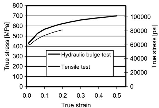
Fig. 13. Flow stress curves of HS steel.
