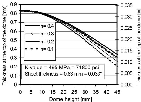
Fig. 5. Thickness at the top of the dome versus dome height for constant  $k$  and various  $n$ -values.
