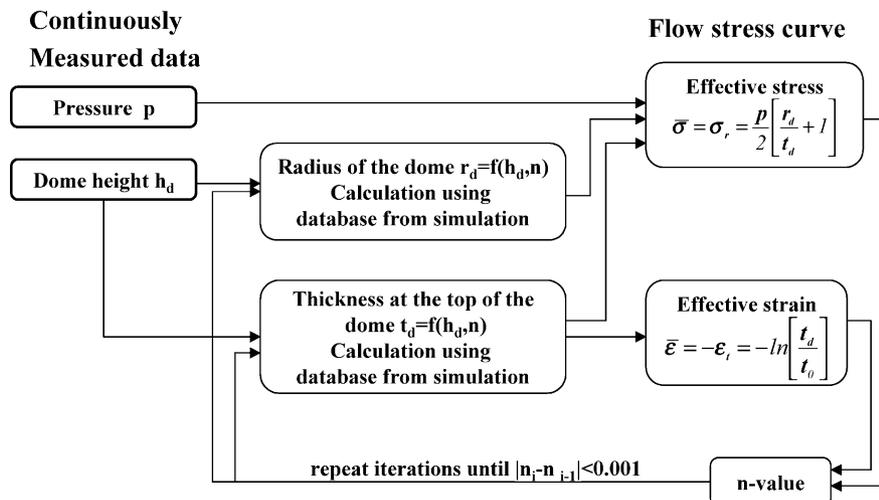
Fig. 10. Determination of flow stress curve.
