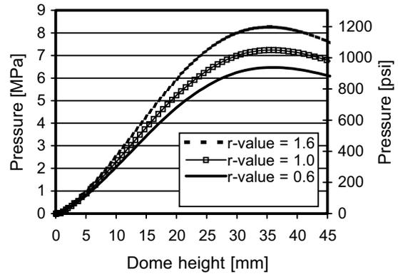
Fig. 9. Hydraulic pressure versus dome height for different  $r$ -values.
