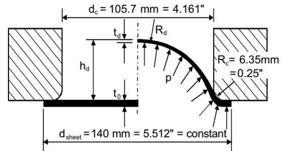
Fig. 3. Geometry of the simulated bulging test.
