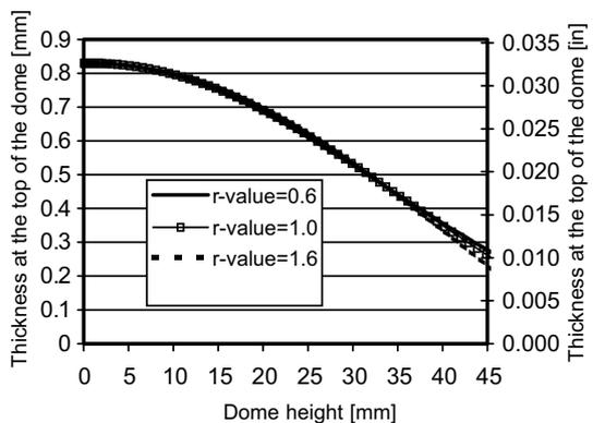
Fig. 7. Thickness at the top of the dome versus dome height for various  $r$ -values.
