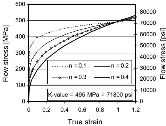
Fig. 4. Flow stress curves ( $\bar{\sigma} = K\bar{\epsilon}^n$ ) for constant  $k$  and various  $n$ -values.
