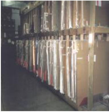
Figure 3.8: Stored Signs Kept Wrapped
