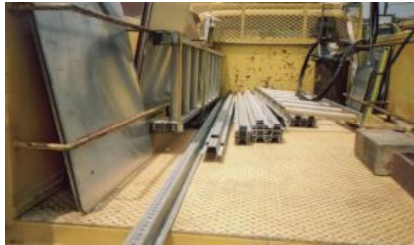
Figure 3.6: Sign Storage Racks on a Signing Truck
