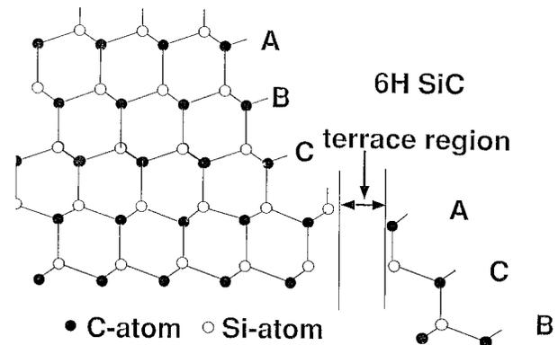
FIG. 1. Schematic representation of surface and step bonding for 6H SiC vicinal wafers. The C atom dangling bonds for the first 6-atom, 3-layer sequence are one per step edge C atom; for the second 6-atom, 3-layer sequence, there are two dangling bonds per step edge C atom. The 6-atom steps are separated by flat terrace regions with Si-atom dangling bonds.
