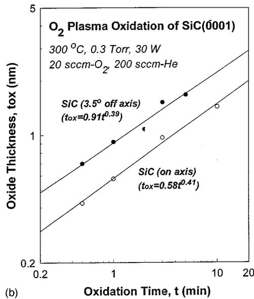
FIG. 6. Log-log plots of the oxide thickness versus the oxidation time for the O<sub>2</sub> RPAO of flat and vicinal (a) Si and (b) SiC. The data are fit to a power law dependence,  $t_{ox} = at^b$ .
