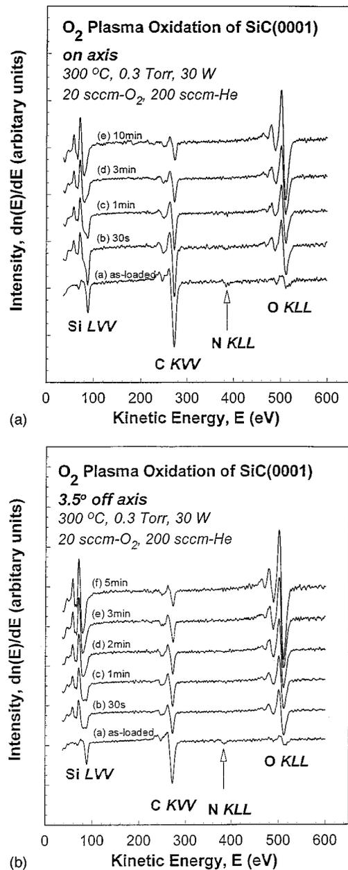
Fig. 2. Derivative mode AES spectra for (a) flat and (b) vicinal SiC obtained by RPAO at 300 °C using O<sub>2</sub> as the oxygen atom source gas.
