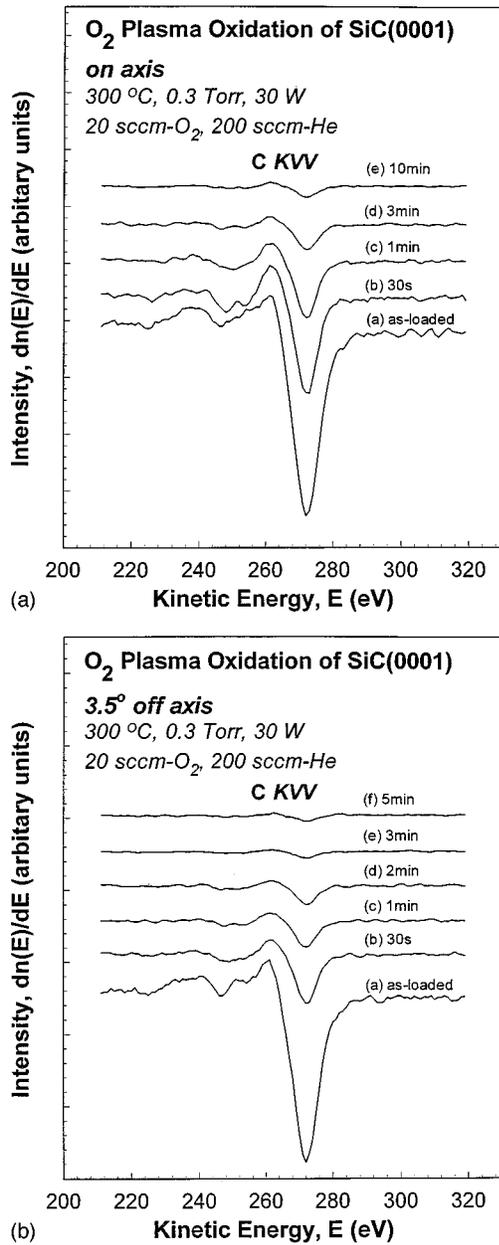
FIG. 4. Changes in the C<sub>KVV</sub> AES features as a function of the oxidation time for (a) flat and (b) vicinal SiC surfaces for O<sub>2</sub> RPAO.
