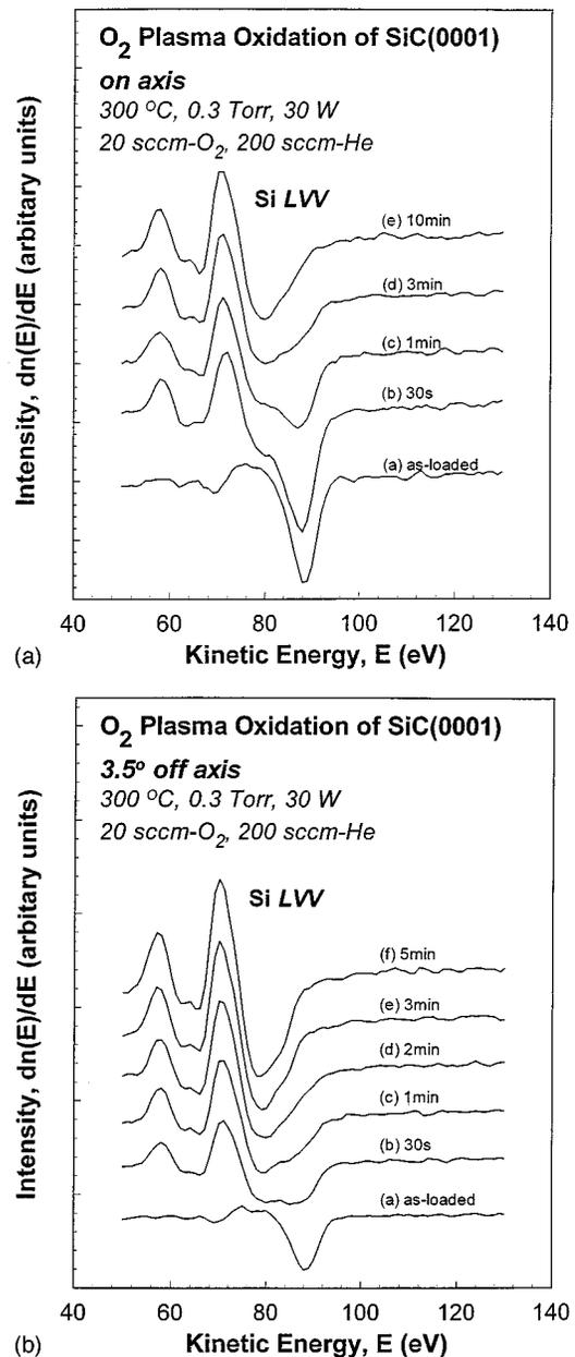
FIG. 3. Changes in the Si<sub>L<sub>VV</sub></sub> AES features as a function of the oxidation time for (a) flat and (b) vicinal SiC surfaces for O<sub>2</sub> RPAO.
