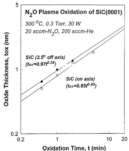
FIG. 8. Log-log plots comparing the oxide thickness versus the oxidation time for the RPAO of flat SiC using O<sub>2</sub> and N<sub>2</sub>O as the oxygen atom source cases. The data are fit to a power law dependence,  $t_{ox} = at^b$ .
