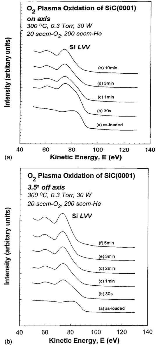
FIG. 5. Integral,  $n(E)$ , Si<sub>L<sub>VV</sub></sub> AES spectra as a function of the O<sub>2</sub> RPAO oxidation time for (a) flat and (b) vicinal SiC surfaces.
