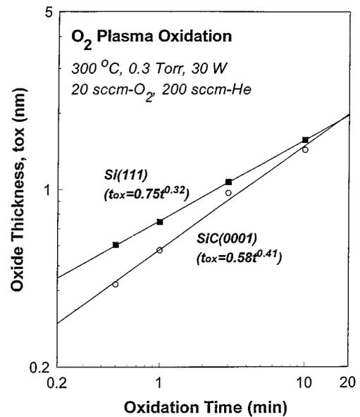
FIG. 7. Log-log plots comparing oxide thickness versus the oxidation time for the O<sub>2</sub> RPAO of flat Si and SiC. The data are fit to a power law dependence,  $t_{ox} = at^b$ .
