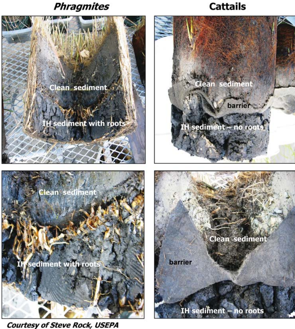
Figure 4 Phragmites australis and cattails ( Typha angustifolia ) growth in greenhouse containers. Plants were rooted in clean soil that was placed on top of IHC sediment. Phragmites grew around and into the oiled sediment, whereas cattails did not. (Courtesy of Steve Rock.)
