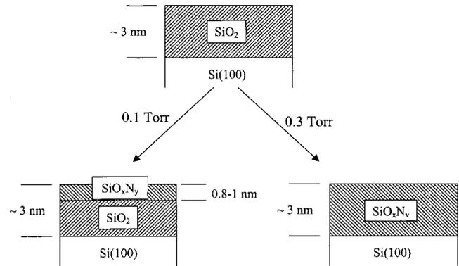
FIG. 12. Schematic representation of the nitridation process and the resultant N distribution for a He/N<sub>2</sub> plasma at (a) 0.1 Torr and (b) 0.3 Torr
