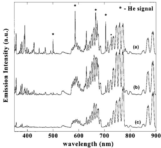
FIG. 10. Optical emission spectra of remote He/N<sub>2</sub> and N<sub>2</sub> plasmas at 0.3 Torr and applied power: 30 W (a) He(160 sccm)/N<sub>2</sub>(60 sccm) plasma (downstream) (b) He(160 sccm)/N<sub>2</sub>(60 sccm) plasma (upstream), and (c) undiluted N<sub>2</sub> (180 sccm) plasma (upstream).
