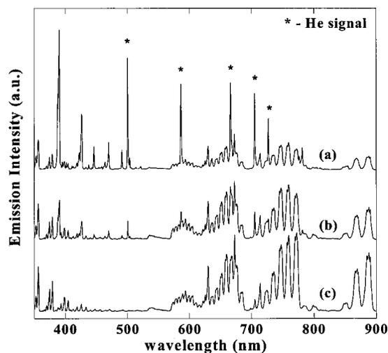
FIG. 9. Optical emission spectra of remote  $\text{He}/\text{N}_2$  and  $\text{N}_2$  plasmas at 0.1 Torr and applied power: 30 W (a)  $\text{He}(160 \text{ sccm})/\text{N}_2(60 \text{ sccm})$  plasma (downstream) (b)  $\text{He}(160 \text{ sccm})/\text{N}_2(60 \text{ sccm})$  plasma (upstream), and (c) undiluted  $\text{N}_2$  (60 sccm) plasma (upstream).
