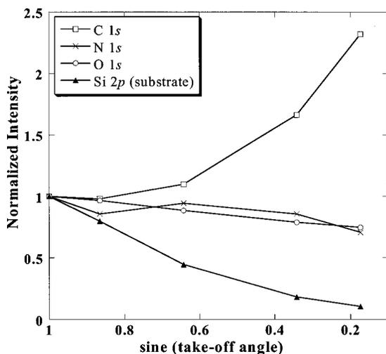
FIG. 8. Normalized N  $1s$ , O  $1s$ , Si  $2p$ (substrate), and C  $1s$  photoelectron signals as a function of sample orientation. The 3 nm  $\text{SiO}_2$  film was nitrided for 30 min at 0.3 Torr (upstream) and 30 W in  $\text{He}/\text{N}_2$  plasma.
