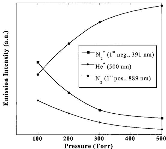
FIG. 11. Intensities of N<sub>2</sub><sup>+</sup> (391 nm), He (500 nm), and N<sub>2</sub> 1+ (889 nm) optical emission lines as a function of pressure for the for He/N<sub>2</sub> remote plasmas (upstream).
