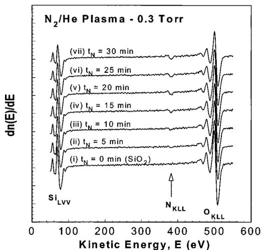
FIG. 2. AE spectra of a 3 nm SiO<sub>2</sub> film nitrided for different times at 0.3 Torr (upstream) and 30 W in He/N<sub>2</sub> plasma.
