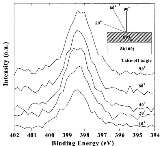
FIG. 7. N  $1s$  photoelectron spectra for selected takeoff angles from a 3 nm  $\text{SiO}_2$  film nitrided by  $\text{He}/\text{N}_2$  plasma (at 0.3 Torr, upstream) for 30 min at 30 W.
