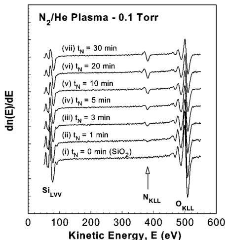
FIG. 1. AE spectra of a 3 nm SiO<sub>2</sub> film nitrided for different times at 0.1 Torr (upstream) and 30 W in He/N<sub>2</sub> plasma.
