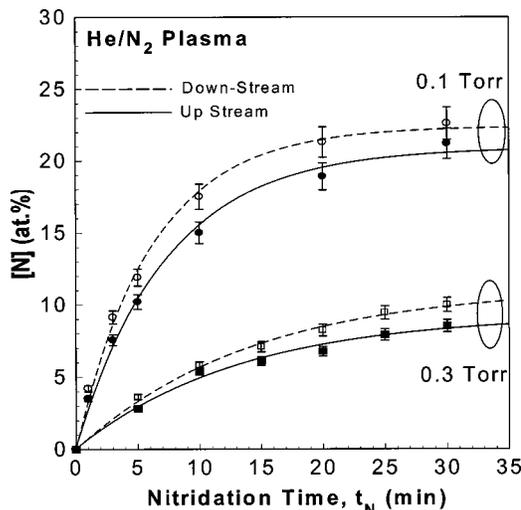
FIG. 3. Comparison of nitrogen concentration in a 3 nm SiO<sub>2</sub> film nitrided for different times at 0.1 and 0.3 Torr (upstream and downstream) and 30 W in He/N<sub>2</sub> plasma.
