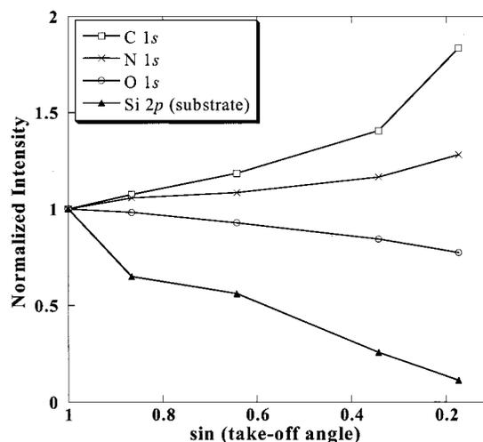
FIG. 6. Normalized  $\text{N } 1s$ ,  $\text{O } 1s$ ,  $\text{Si } 2p$ (substrate), and  $\text{C } 1s$  photoelectron signals as a function of sample orientation. The 3 nm  $\text{SiO}_2$  film was nitrided for 30 min at 0.1 Torr (upstream) and 30 W in  $\text{He}/\text{N}_2$  plasma.
