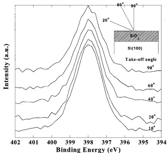
FIG. 5.  $\text{N } 1s$  photoelectron spectra for selected takeoff angles. The 3 nm  $\text{SiO}_2$  film was nitrided for 30 min at 0.1 Torr (upstream) and 30 W in  $\text{He}/\text{N}_2$  plasma.
