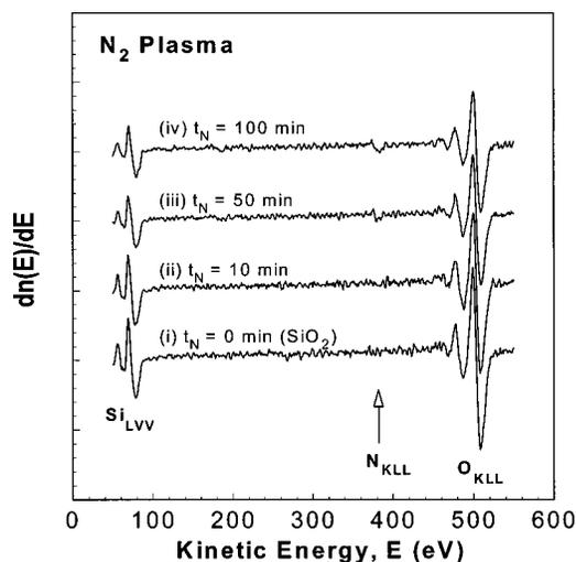
FIG. 4. AE spectra at different nitridation times for a 3 nm  $\text{SiO}_2$  film nitrided by  $\text{N}_2$  plasma (60 sccm) at 0.1 Torr and 30 W.
