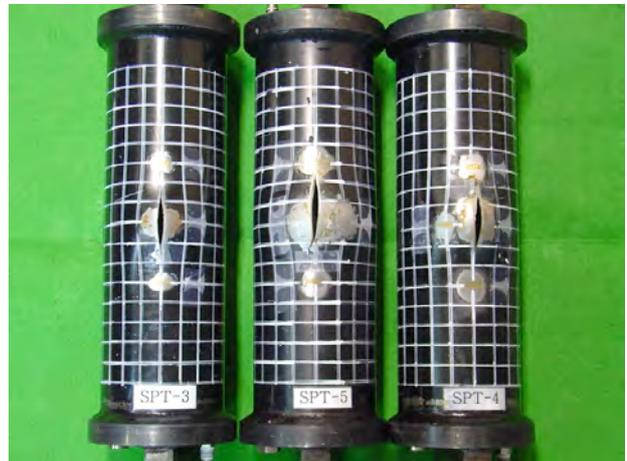
(b) Final failure mode
