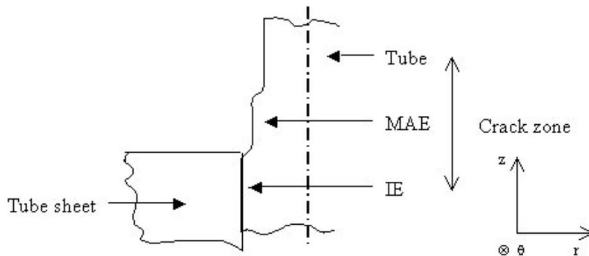
**Figure 1.** : Schematic representation of expansion variation zone of a Steam Generator tube
