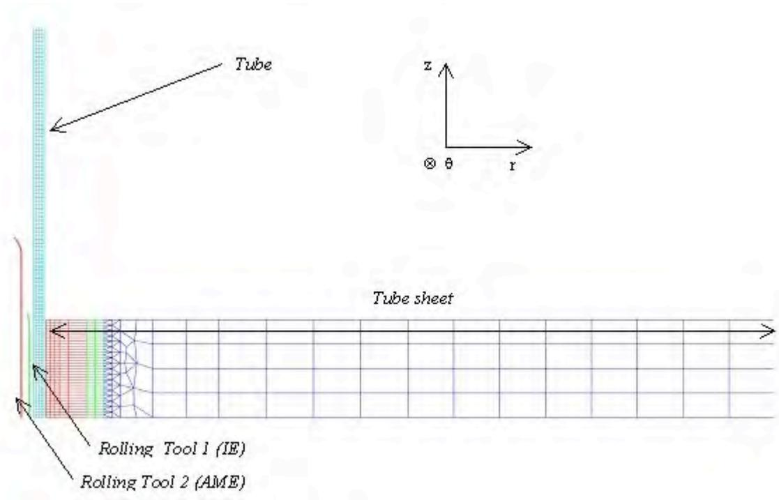
**Figure 4.** 2D-Axi-symmetric model
