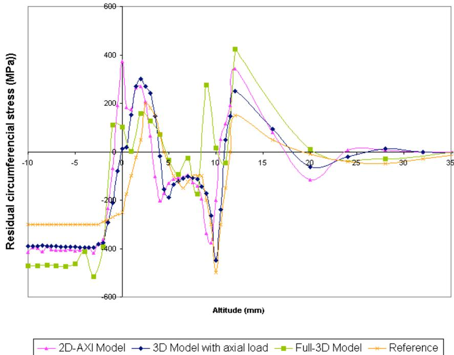
**Figure 8.** Comparison of the residual stress on the inner skin of tube for the different models
