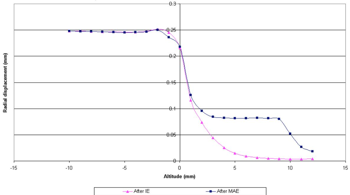
**Figure 6.** Inner skin profile after unload with Full-3D model
