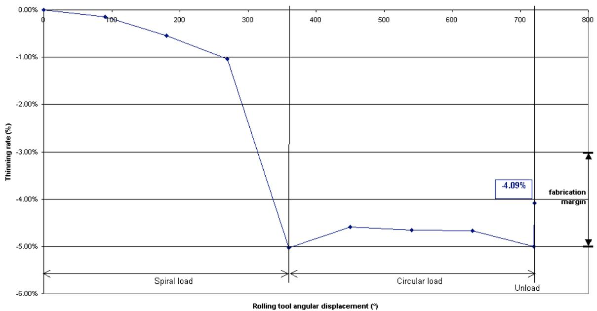
**Figure 7.** Thinning rate evolution with Full-3D model
