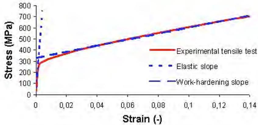
Figure 2. Identification of the elastic-plastic behaviour of the tube
