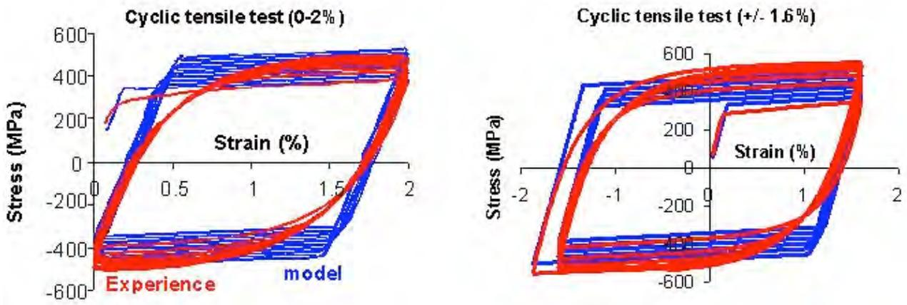
Figure 3. Identification of the cyclic behaviour of the tube
