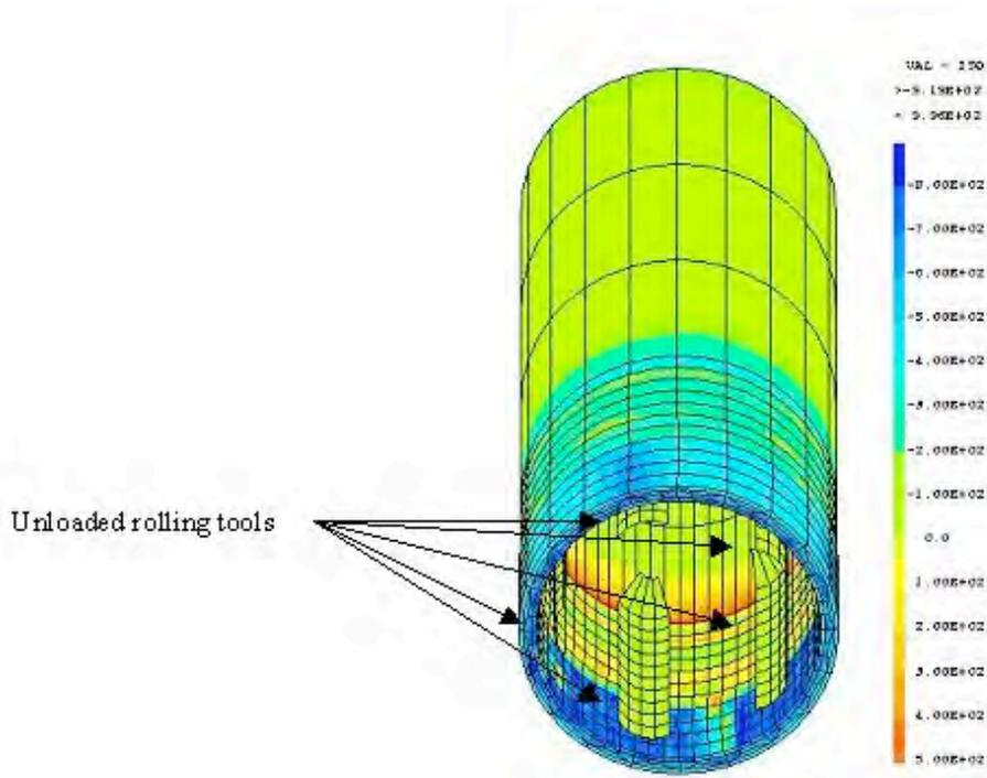
**Figure 9.** Projection of the circumferential residual stress field on the deformed mesh after unload
