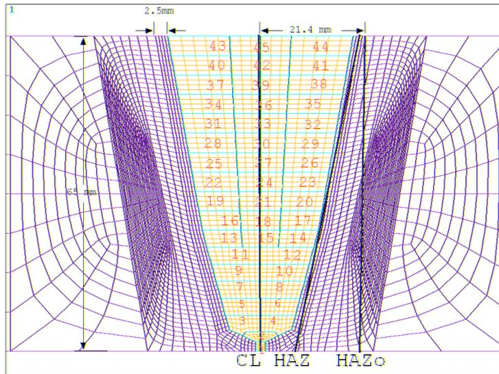
**Figure 8:** Geometry, finite element mesh and weld pass definition for Case 2.
