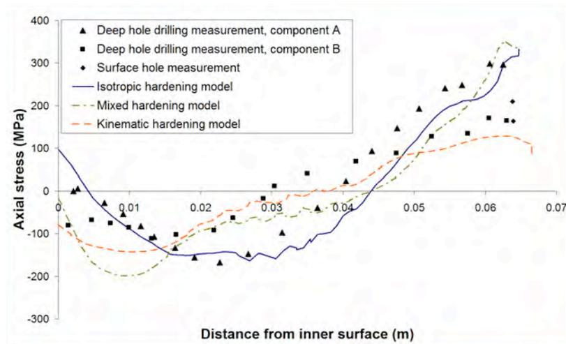
**Figure 11:** Case 2. Comparison of the predicted axial residual stress along path HAZo (defined in Figure 8) with the measured.
