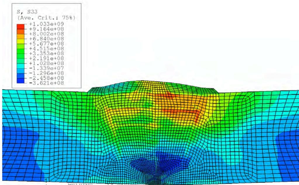
**Figure 5:** Hoop residual stress for the medium thick-walled case 2 weld at 20 °C (unit Pa).
