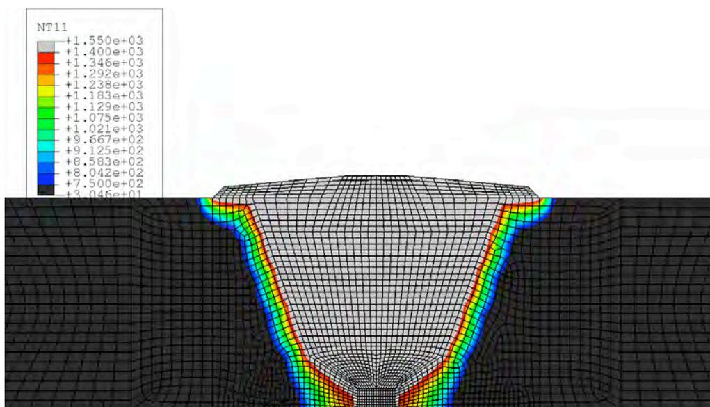
**Figure 3:** Fusion zone and HAZ. Maximum temperature experienced during the welding. The locations with maximum temperature >1400 °C are in gray, <750 °C are in black.
