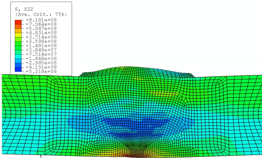
**Figure 4:** Axial residual stress for the medium thick-walled case 2 weld at 20 °C (unit Pa).
