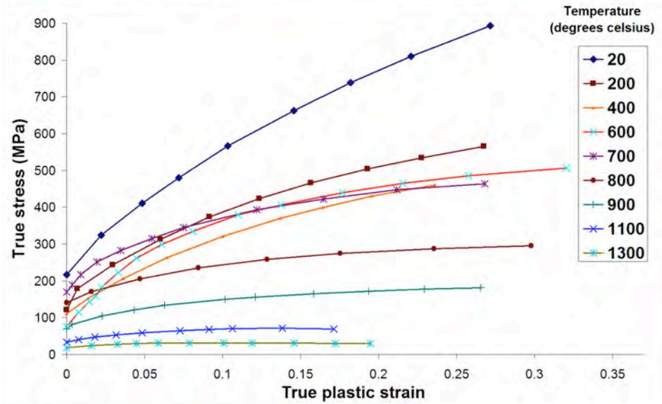
**Figure 1.** The flow stress of 316L stainless steel at a strain rate of  $10^{-2}\text{s}^{-1}$  for temperatures between 20 and 1300°C (Lindgren, 2008).
