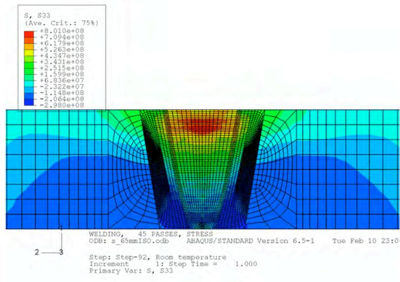
**Figure 10:** Hoop residual stress for the thick-walled case 2 weld at 20 °C (unit Pa).
