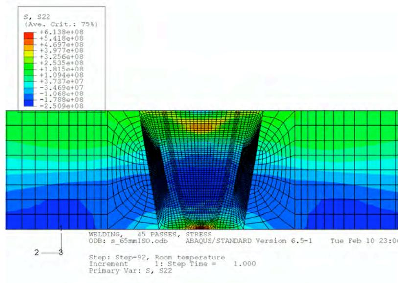
**Figure 9:** Axial residual stress for the thick-walled case 2 weld at 20 °C (unit Pa).
