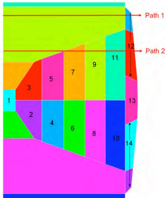
**Figure 2:** Geometry and definition of sequence of welding for Case 1.
