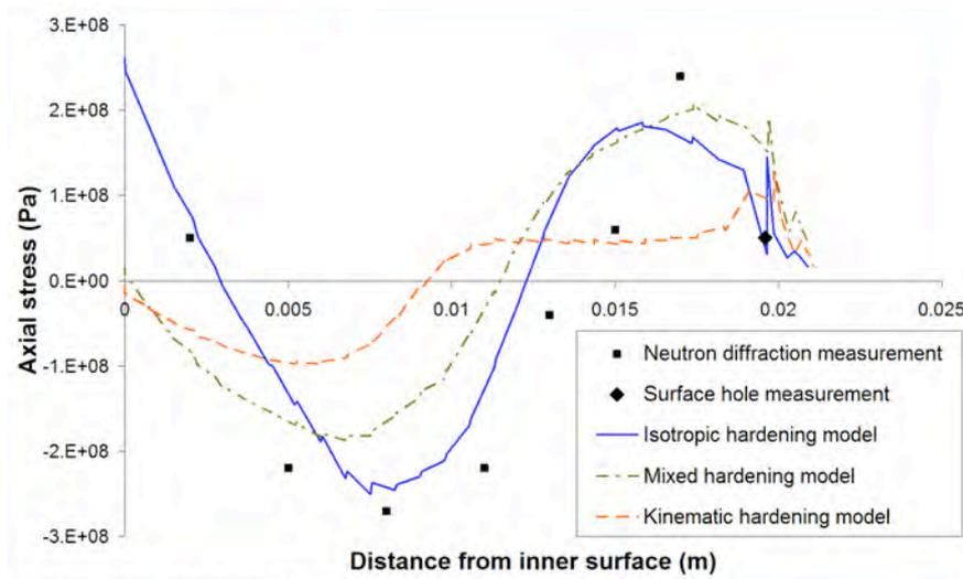
**Figure 6:** Case 1. Comparison of predicted axial residual stress along Path 1 (defined in Figure 2) for different hardening models. Available experimental data is also plotted.
