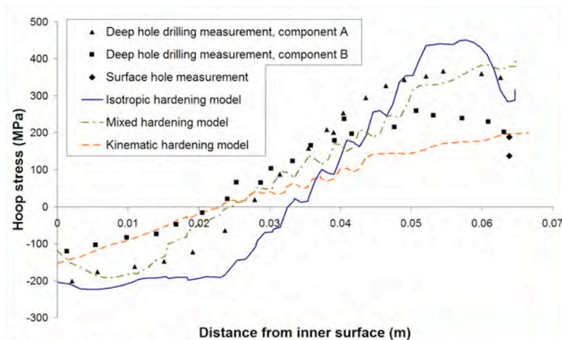
**Figure 12:** Case 2. Comparison of the predicted hoop residual stress along path HAZo (defined in Figure 8) with the measured.
