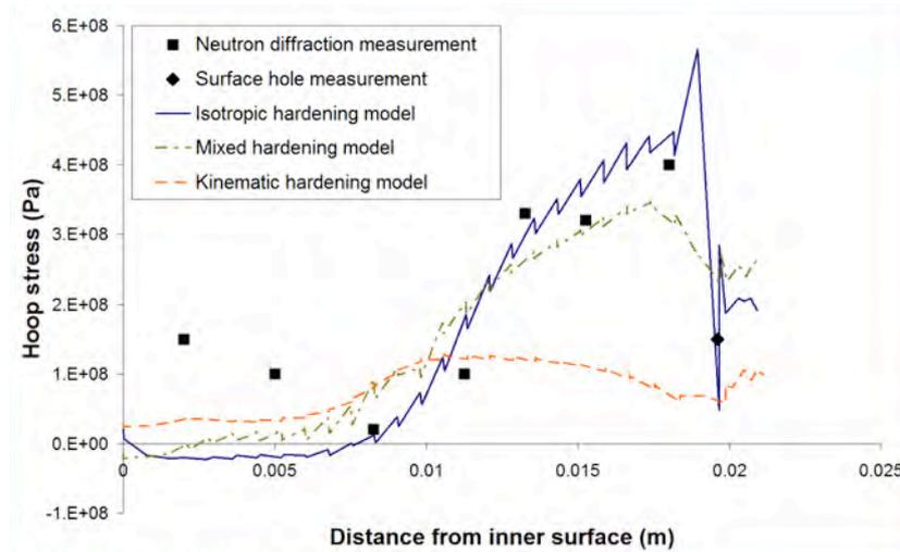
**Figure 7:** Case 1. Comparison of predicted hoop residual stress along Path 1 for different hardening models. Available experimental data is also plotted.
