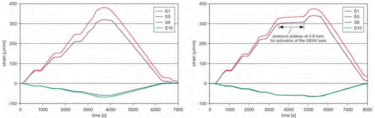
**Figure 8.** Internal strain measurements during RUN 2 (left) and RUN 3 (right)
