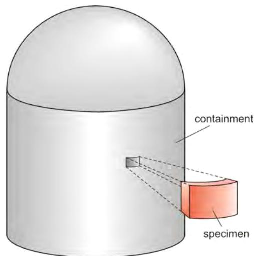
**Figure 2.** The specimen is cut out of the cylindrical part of the containment
