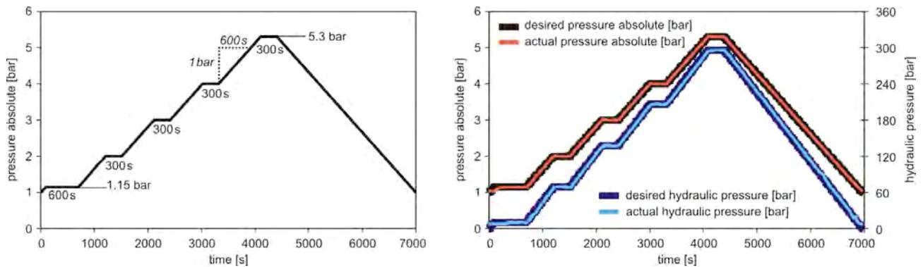
**Figure 7.** Pressure scenario for RUN 1 to RUN 3 (left), example for control (right)
