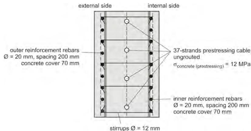
**Figure 5.** Section of the specimen as part of the containment
