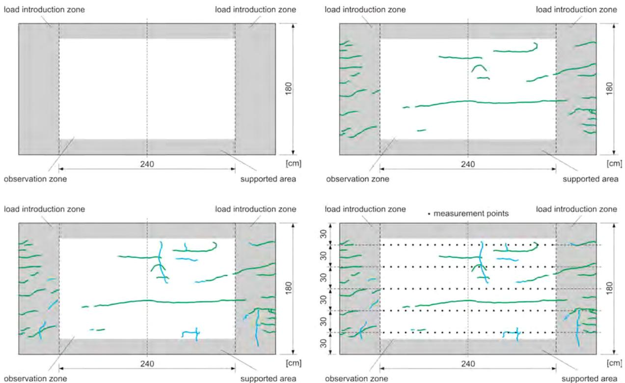
**Figure 11.** Crack development at the lower surface of the specimen after RUN 1 (top left), RUN 2 (top right), RUN 3 (bottom left) and the prepared steel ball grid for RUN 4 (bottom right)
