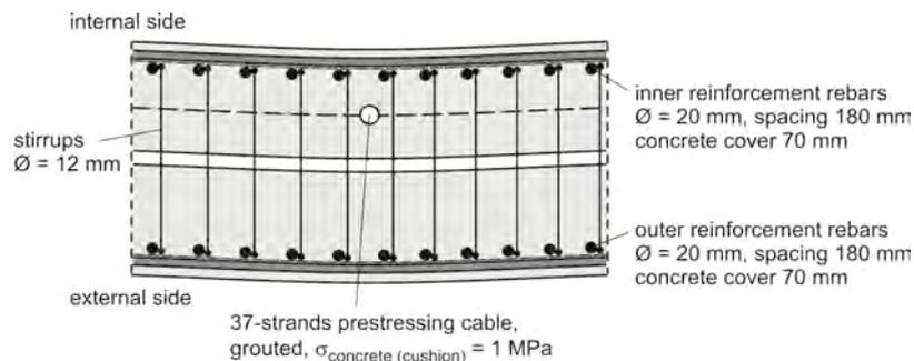
**Figure 6.** Vertical section of the specimen in longitudinal direction positioned as in the tests
