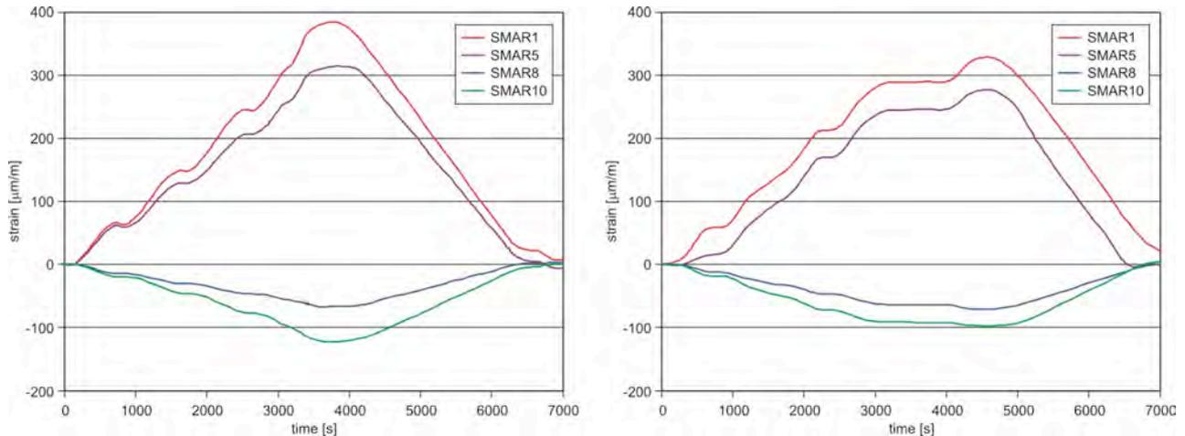
**Figure 9.** Internal strain measurements by the SMARTEC-sensors during RUN 2 (left) and RUN 3 (right)
