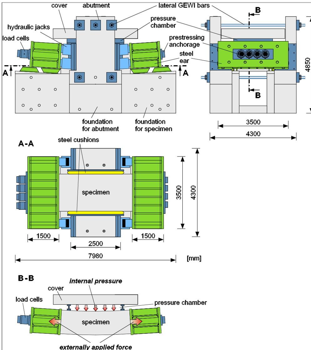
**Figure 3.** Drawings of the mechanical part of the facility, in section B-B the internal pressure and the externally applied force is shown in principle
