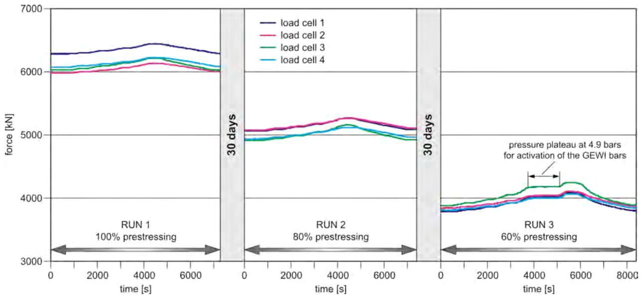
**Figure 10.** Change in the prestressing force during RUN 1, RUN 2 and RUN 3
