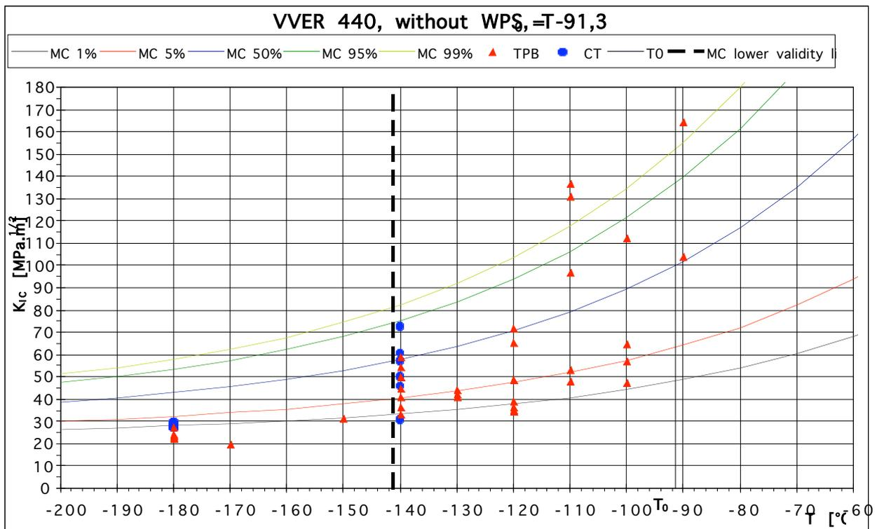
fracture were chosen, namely temperatures -180°C, -140 °C and -120 °C. As the Master Curve theory is valid only within the range  $T_0 \pm 50$  °C and the proposed fracture temperatures lye outside or close to the limits, it was decided to perform sufficient number of tests (without WPS) directly at these proposed
