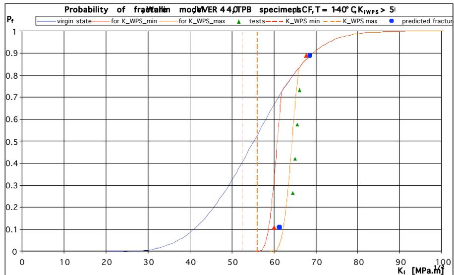
Figure 7. LCF regime, results of evaluation of experimental data for using Wallin model
