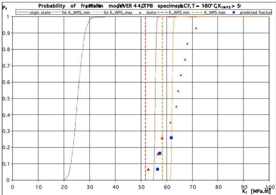
Figure 6. LCF regime, results of evaluation of experimental data for using Wallin model
