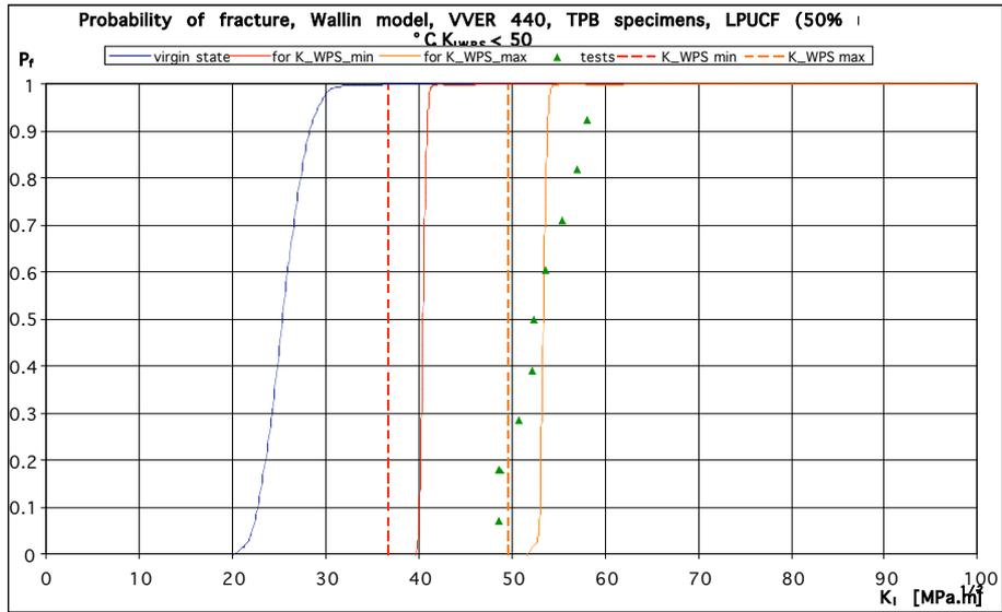
Figure 5. LPUCF regime, results of evaluation of experimental data for using Wallin model
