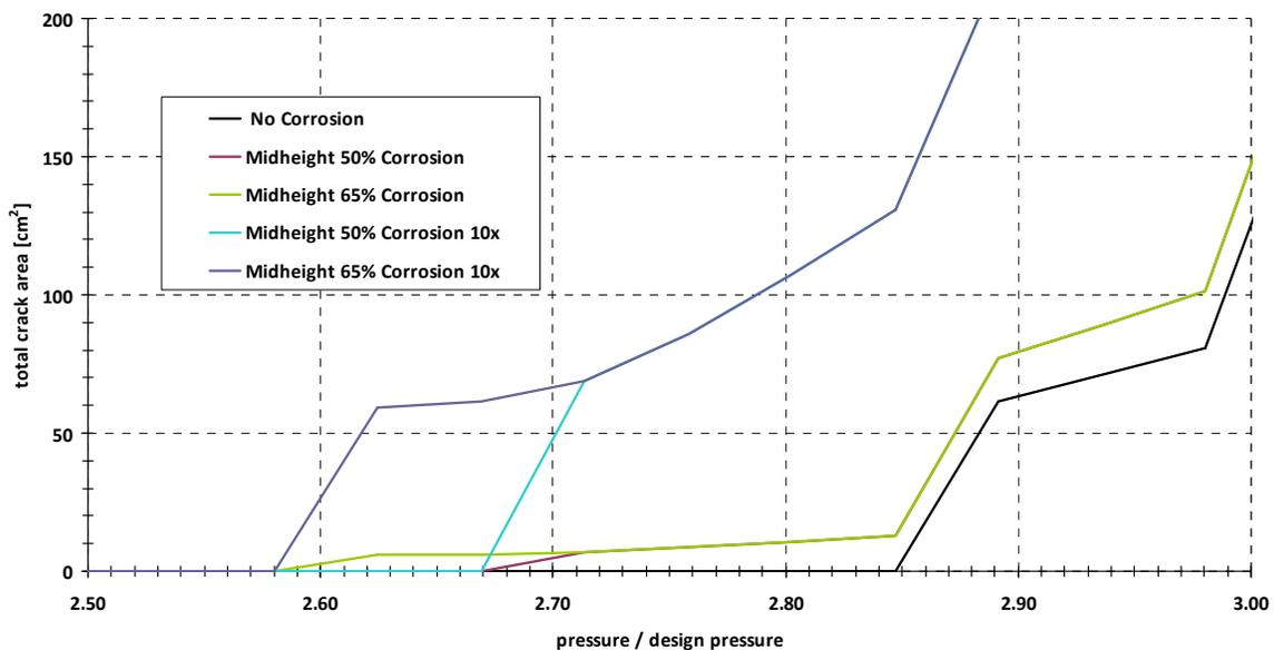
**Figure 4.** Crack Area vs Pressure
