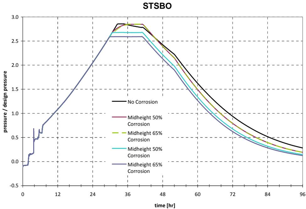
**Figure 6.** STSBO Containment Pressure vs Time
