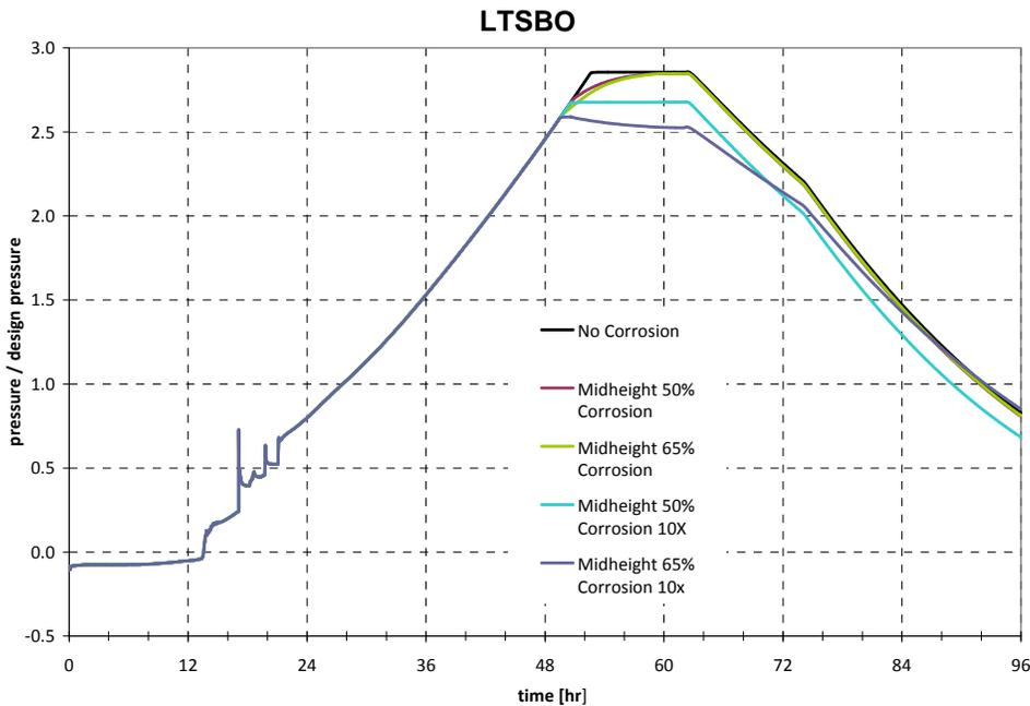
Figure 5. LTSBO Containment Pressure vs Time
