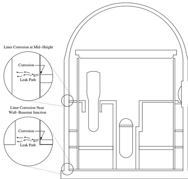
**Figure 1.** Reinforce Concrete Containment Leak Paths
