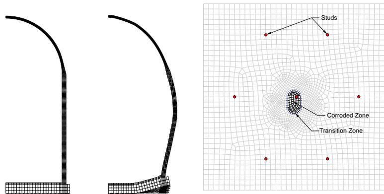
**Figure 2.** Reinforced Concrete Containment Finite Element Model
