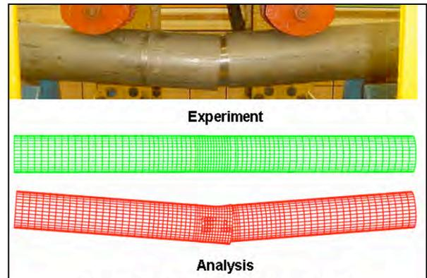
Fig. 6 Deformation of pipe after unloading
