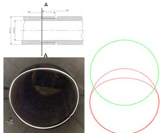
Fig. 8 Deformation at section A-A
