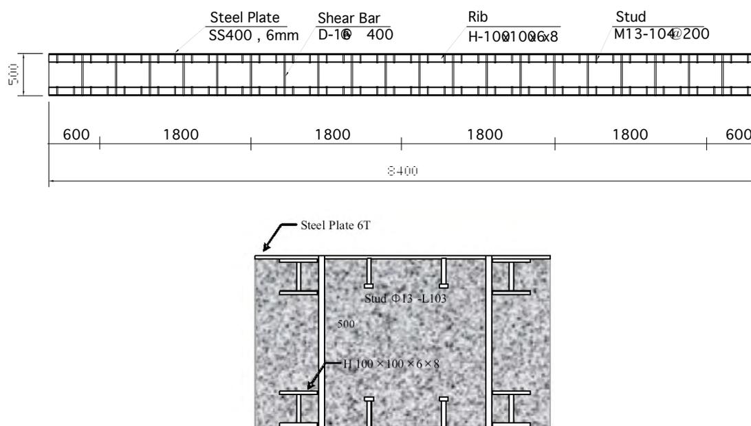
Figure 2. Detail of standard specimen (top), Section detail (bottom)
