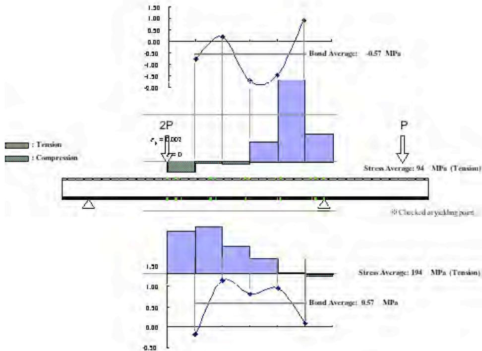
Figure 6. Average bond stress in shear span (S-4R-0S-4ST)
