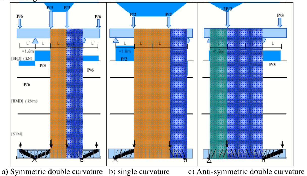
Figure 1. Loading condition for shear transfer
