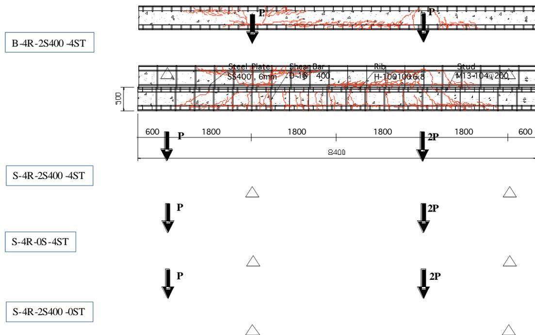
Figure 4. Crack patterns of single curvature test and double curvature test
