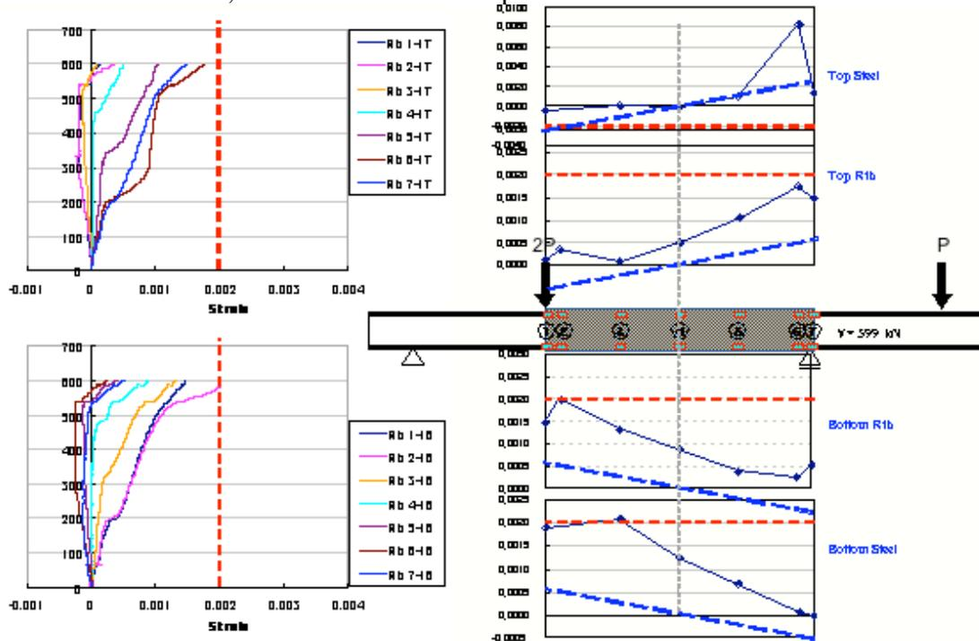
Figure 5. Strain distribution in ribs (S-4R-0S-4ST)
