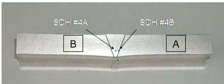
**Figure 3.** Wrought-to-wrought SS calibration standard showing two of five side drilled holes. Fusion lines of the weld with the base metal have been drawn in to add clarity to the location of the SDHs.
