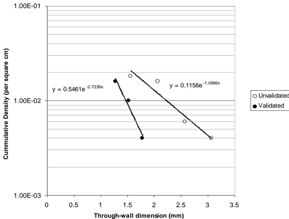
**Figure 8.** Cumulative through-wall size distribution for flaws in wrought-to-wrought SS weld specimen #6 and #7
