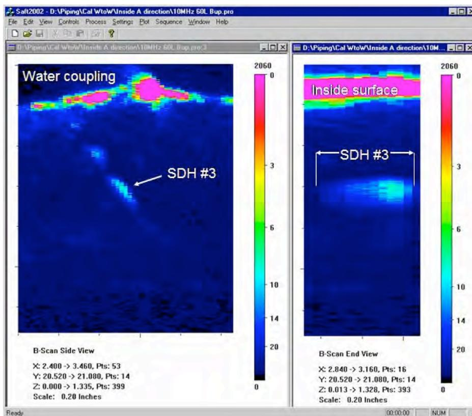
**Figure 4.** SAFT-UT images of 1.5-mm-diameter SDH in wrought-to-wrought SS weld calibration specimen
