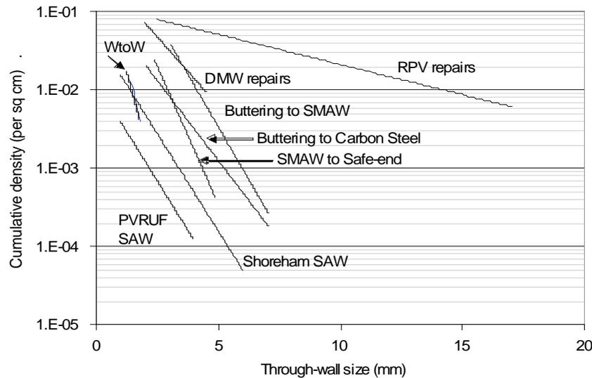
**Figure 9.** Comparison of flaw density and through-wall size distributions. (Note: Wrought-to-wrought is the same as SS to SS).
