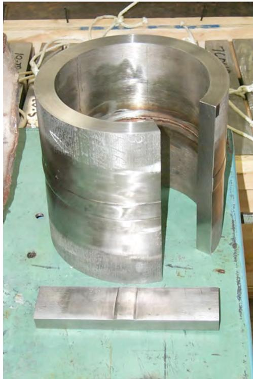
**Figure 1.** Weld #6 with calibration specimen removed from weld
