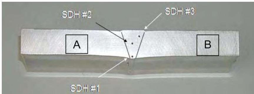
**Figure 2.** Wrought-to-wrought stainless steel (SS) calibration standard showing three of five side-drilled holes. Fusion lines of the weld with the base metal have been drawn in to add clarity to the location of the SDHs.
