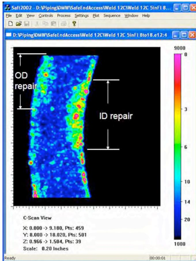
**Figure 7.** Top (C-scan) view image of the segmented ultrasonic responses from the safe end of a dissimilar metal weld showing two repairs (crescent-shaped areas) to the fusion zone of the SMAW with the safe end
