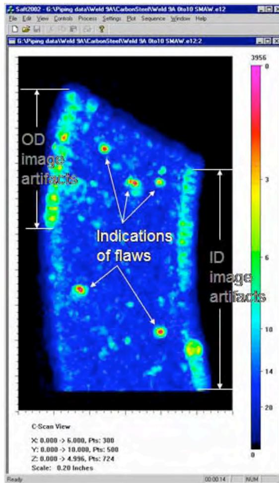
**Figure 6.** Top (C-scan) view image of the segmented ultrasonic responses from SMAW of a DMW
