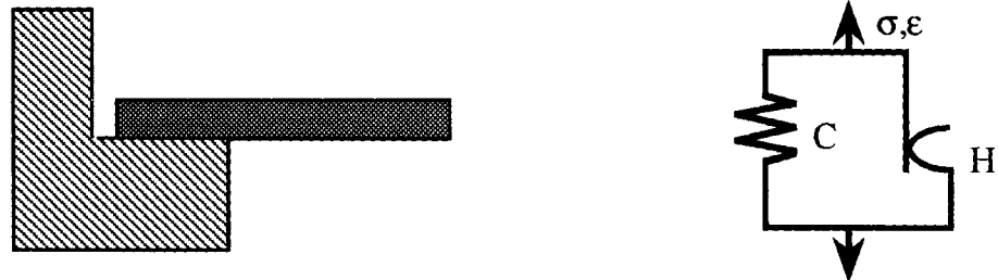
Fig.3 Non-anchored support and its rheological model
