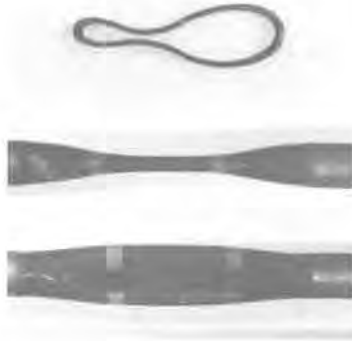
Fig. 5 Tube after creep collapse
