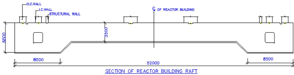
**Fig. 1: Section of Reactor Building Raft**
