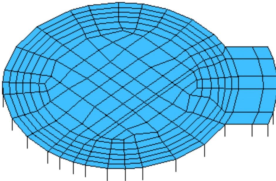
**Fig. 2: FE Model of RB Raft (Without Super Structure)**
