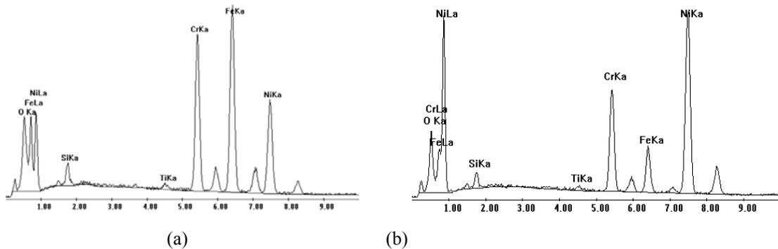
Fig. 5 Worn surface composition of Incoloy 800 and Inconel 690 tested in 290°C water
