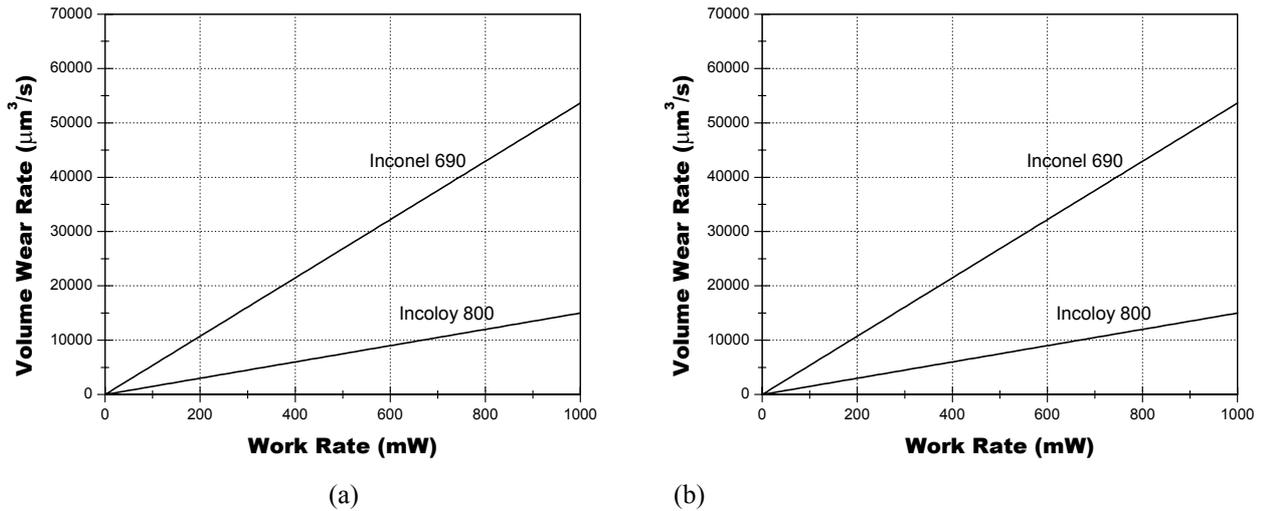
Fig.4 Results of wear test in 290°C water; using work rate model,
