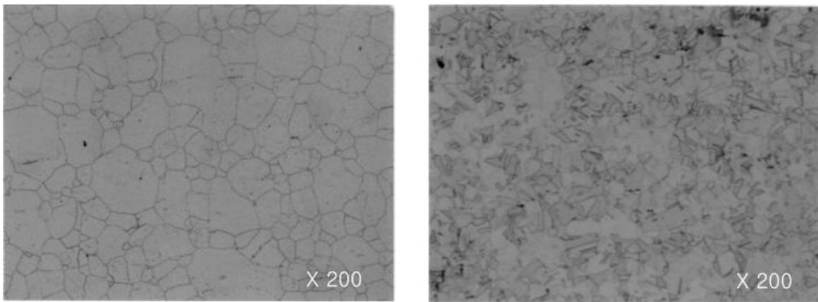
Fig. 1 Microstructures of test materials, (a) Inconel 690, (b) Incoloy 800
