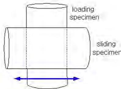
Fig. 2 Sliding specimen setup in autoclave of tube to tube type
