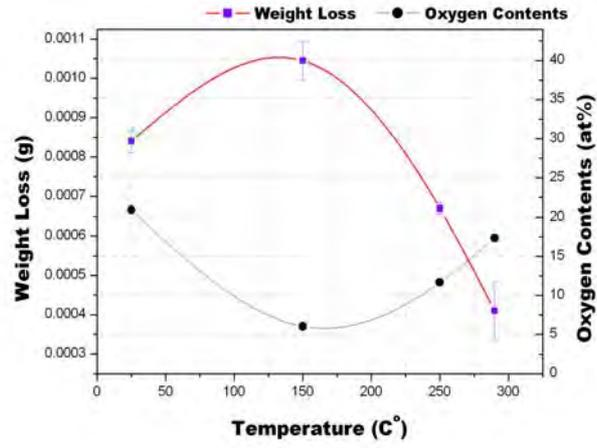
Fig. 6 Changes of weight losses and worn surface oxygen contents with increasing temperature,
