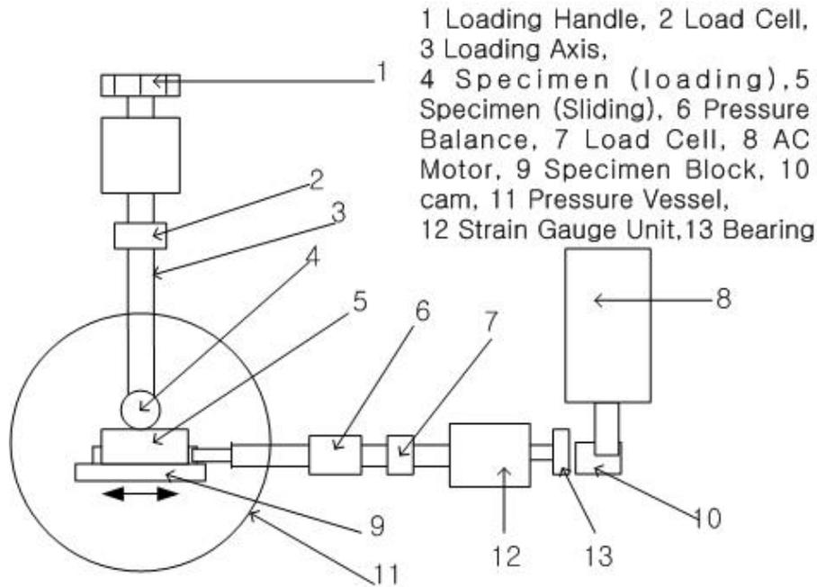
Fig. 3 Schematic diagram of high temperature wear test rig
