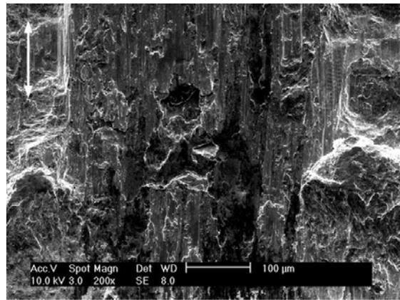
Fig. 7 SEM image worn surface of Incoloy 800 at 290°C water
