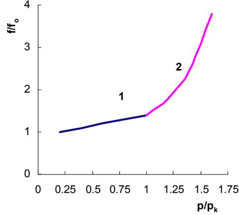
Fig. 2. Typical dependency of friction coefficient on specific mean pressure in the tribo-junction for crystalline solids
