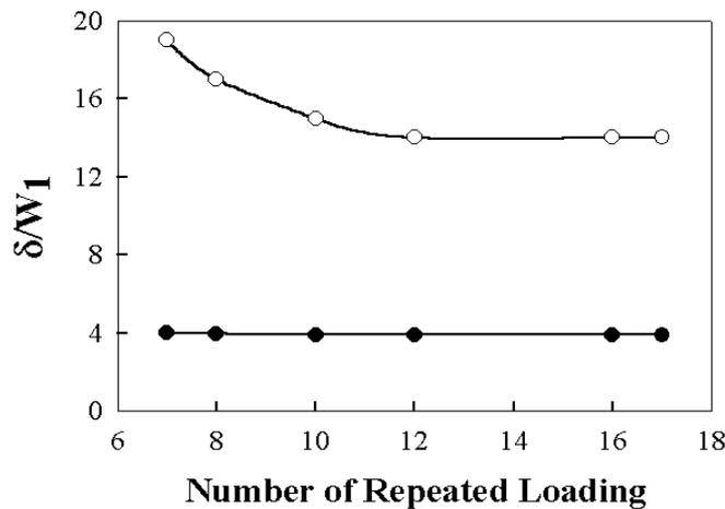
Fig. 3. Dependence of hysteresis deformation  $\delta/w_1$  on the number  $N$  of repeated loading cycles of pressure vessel steels (•) and industrial glass (•)
