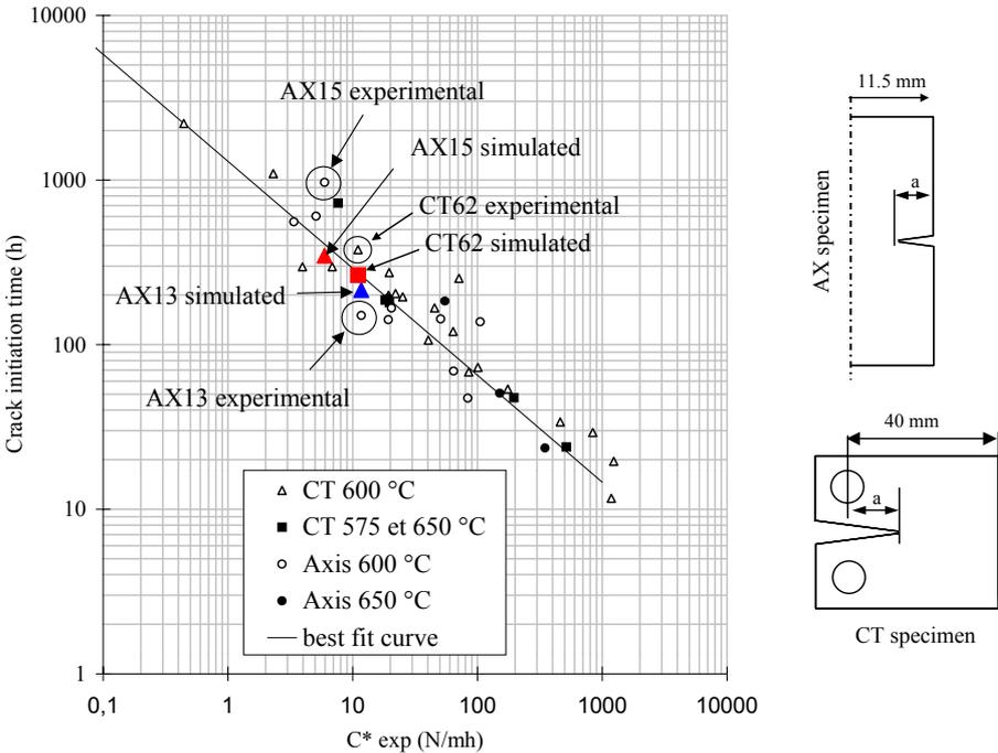
Figure 6 : Creep crack initiation time in fatigue pre-cracked specimens
