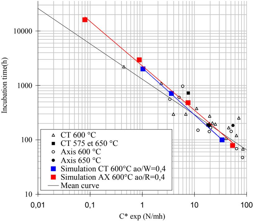
Figure 8 : Long time extrapolation of creep crack initiation assessment.
