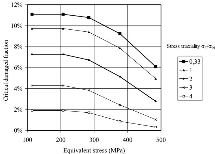
Figure 4 : Critical damaged fraction for 316L(N) steel at 600°C.
