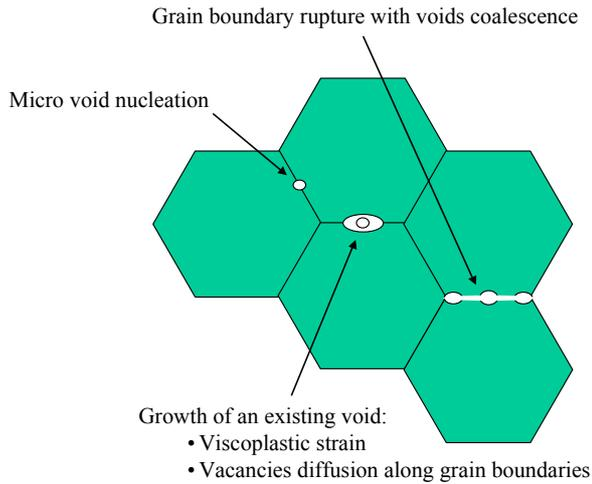
Figure 1 : Intergranular creep damage mechanism in austenitic steels.
