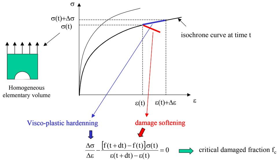
Figure 2 : Mechanical model used for intergranular creep cavities coalescence.
