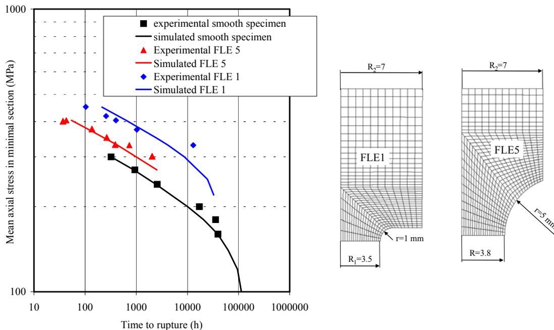
Figure 5 : Creep rupture curves for 316L(N) at 600°C on smooth and notch specimens.
