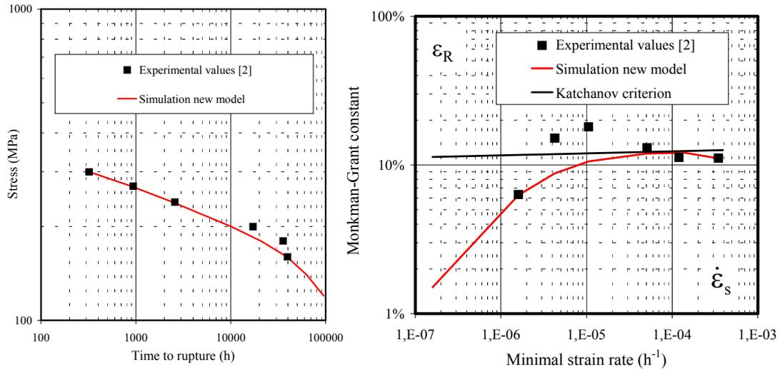
Figure 3 : Tensile creep rupture properties of 316L(N) steel at 600°C.
