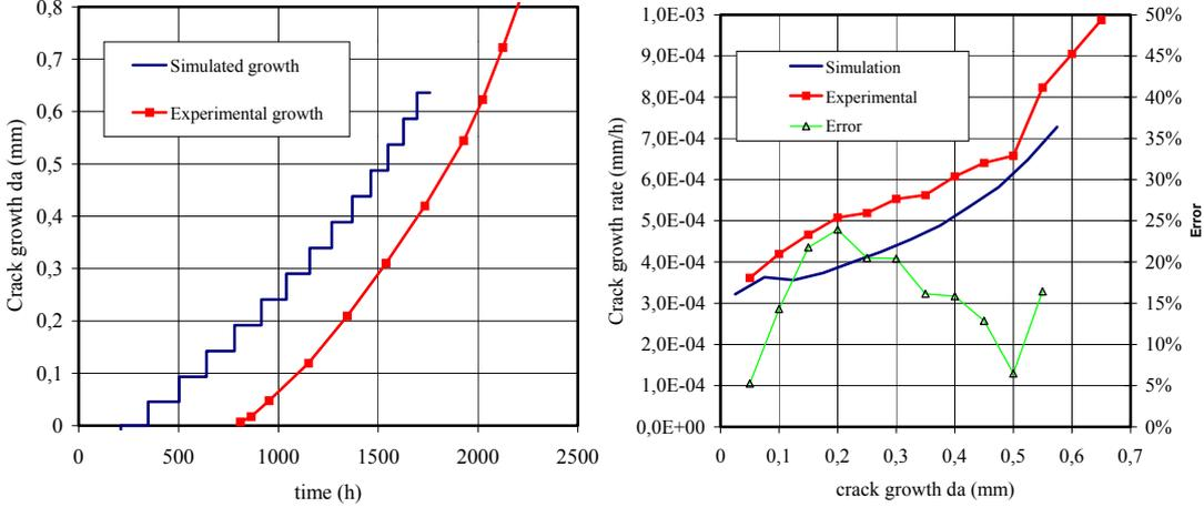
Figure 7 : Creep crack growth on AX15 specimen.
