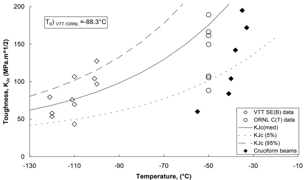
Fig. 4 Comparison the NESC-IV cruciform beam test data with the Master Curve determined for the weld.
