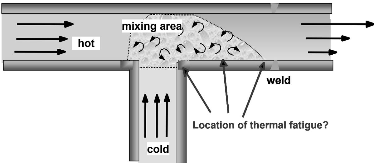
Fig. 7. Schematic of one cause of thermal fatigue at a piping tee-connections
