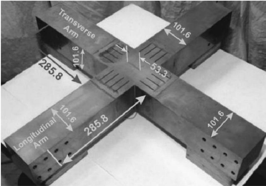
Fig. 3 The ORNL cruciform beam design used for the NESC-IV tests, showing detail of the implanted defect.
