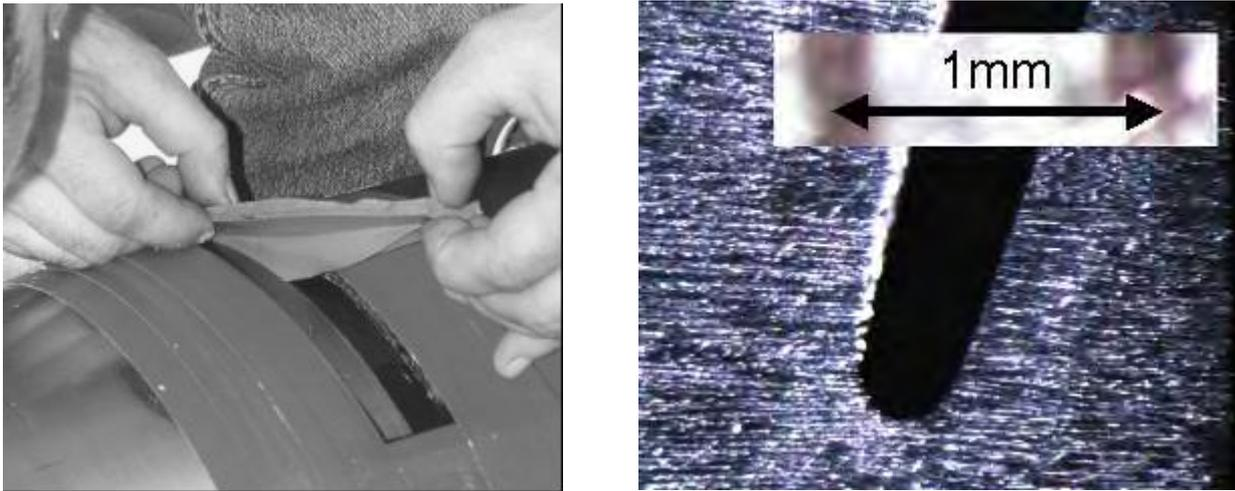
Fig. 6 Insertion of a precision simulated crack in the Adimew dissimilar weld component.
