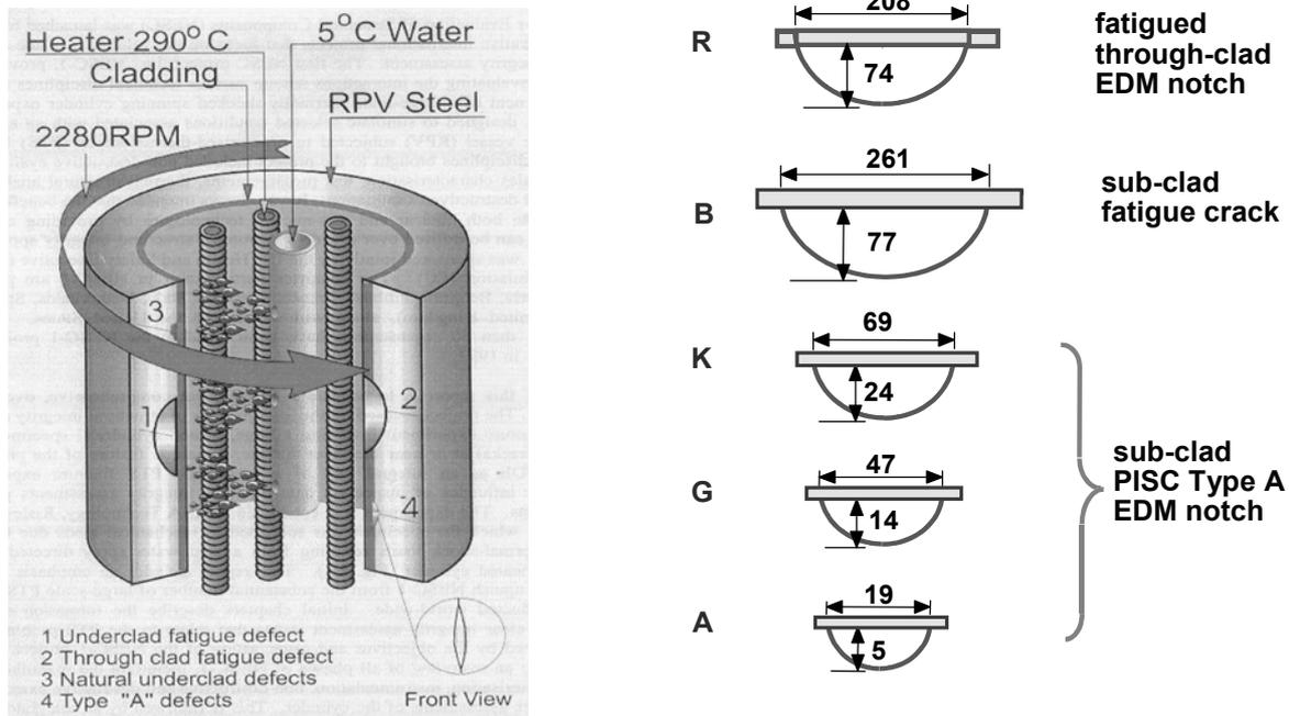
Fig. 2 NESCI component and the principal defects considered in the fracture assessment.
