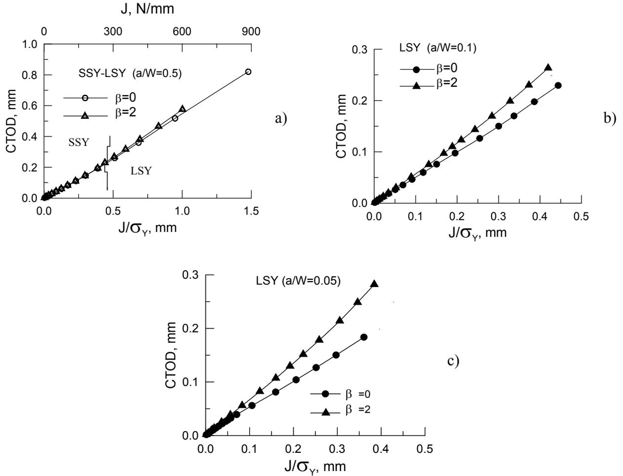
Fig.3 The dependence of CTOD on  $J/\sigma_Y$  for various values of  $\beta$  and  $a/W$ :
