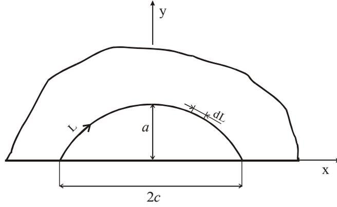
Fig.4 To the calculation brittle strength of reactor pressure vessel for heterogeneous distribution of SIF along the crack front
