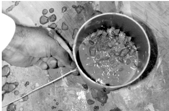
FIGURE 1 : Installation of a thermocouple at the time of the specimen casting
