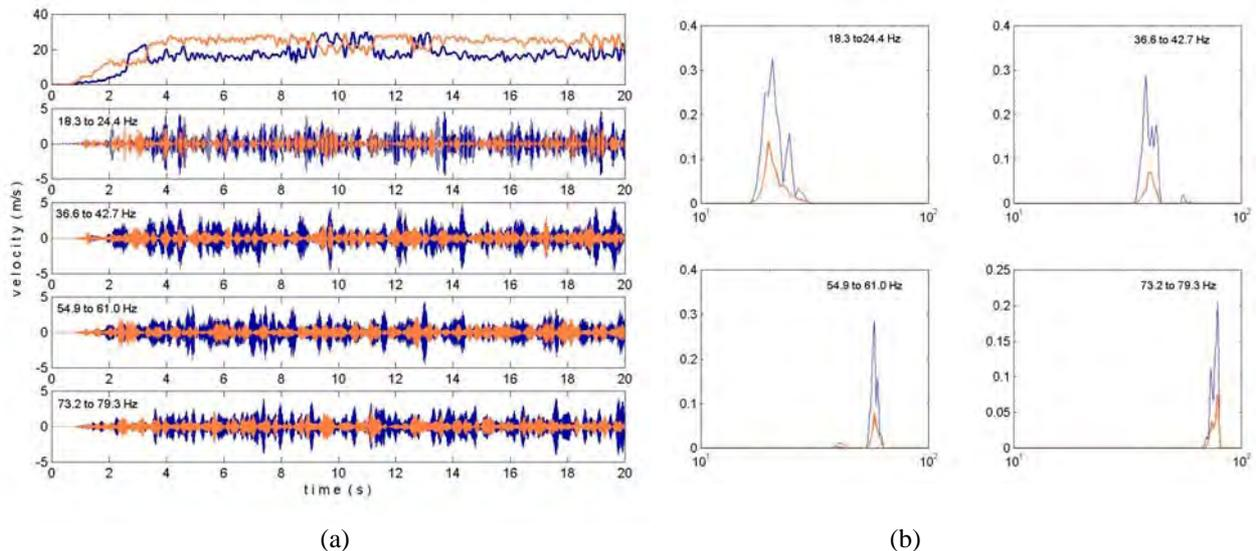
Fig. 7: (a) Time-frequency analysis of velocity and velocity fluctuation behind the central tube of the third row of the bank. (b) Auto spectral densities of the decompositions. Probe "1" blue, Probe "2" orange.
