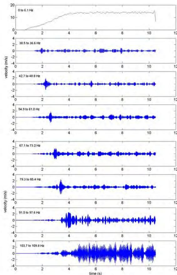
Fig. 3: Some reconstructed nodes for the transient velocity in the wake of a cylinder of Fig (2a), showing the time frequency evolution of the wake.
