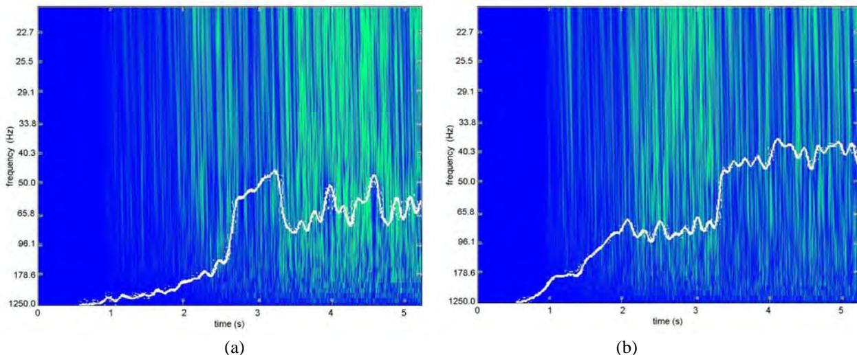
Fig. 8: Continuous wavelet transform of the first quarter part of the velocity signals starting from rest. (a) Probe “1”, (b) Probe “2”. Mean velocity signal is superimposed as reference.
