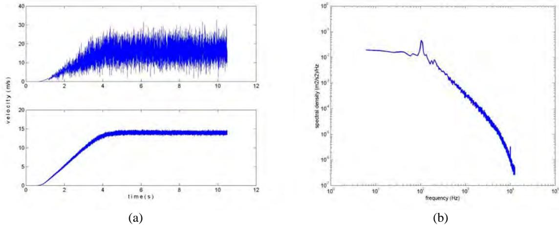
Fig.2: (a) Transient velocity in the wake of a cylinder and free stream reference velocity. (b) Power spectrum of the stationary part of the vortex street series.
