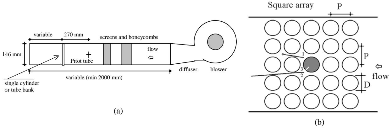
Fig. 1: Schematic view of the test section: (a) wind tunnel configuration; (b) tube bank with location of probes: 1, 2- hot wires, 3- pressure tap for pressure transducer.
